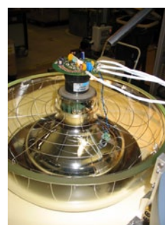
Photomultiplier with PHQ socket supply / Photomultiplier mit PHQ Sockelversorgung
