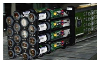
Photomultiplier with PHQ socket supply / Photomultiplier mit PHQ Sockelversorgung
