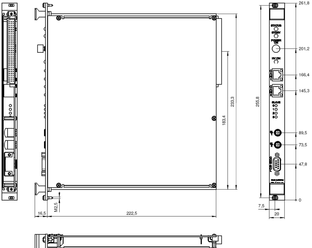
Figure 13: Dimensional drawing CC23, SLAVE
