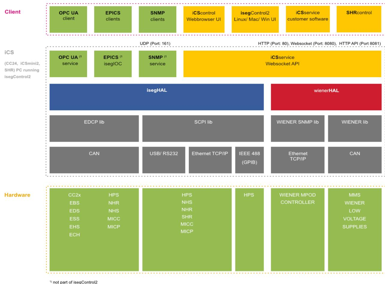
Figure 7: Software architecture
