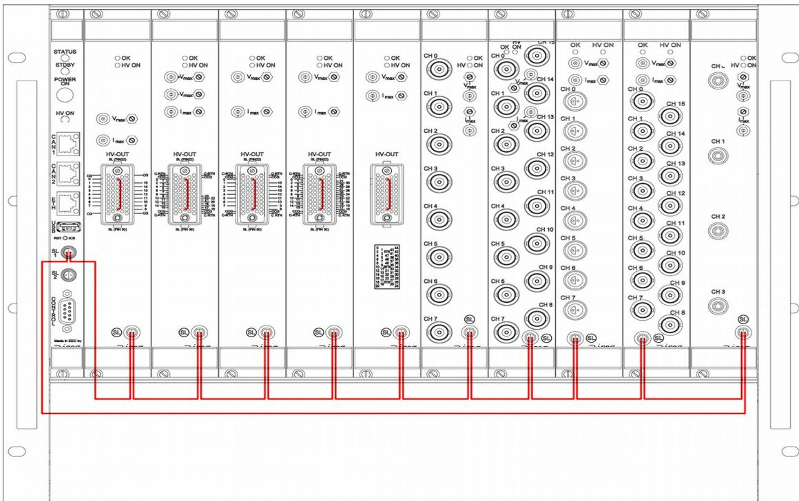
Figure 4: Safety loop 1 - wiring example
