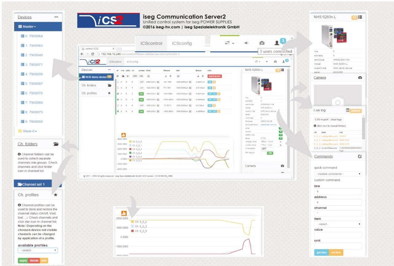
The screenshot displays the iCScontrol software interface for an iCS2 server. The interface is divided into three main sections:
