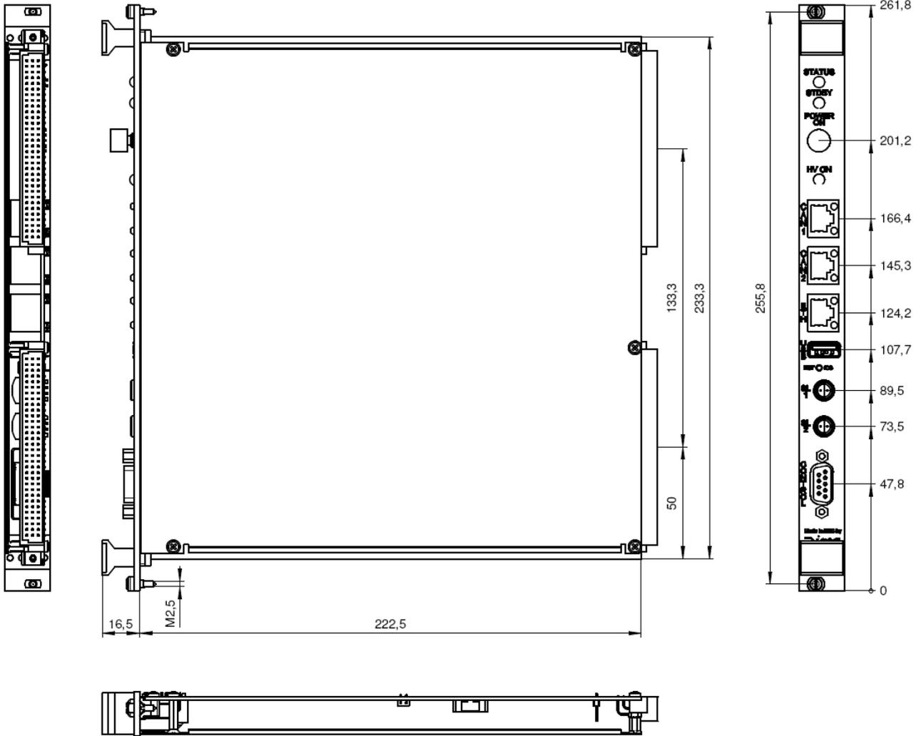
Figure 14: Dimensional drawing CC24, MASTER
