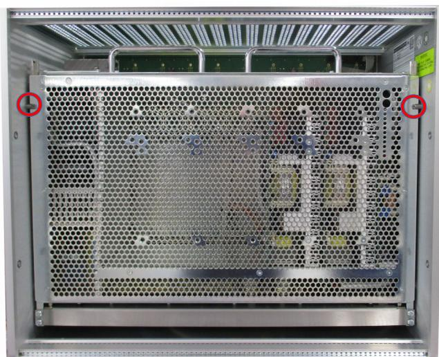
Figure 2: remove screws at the side panel
