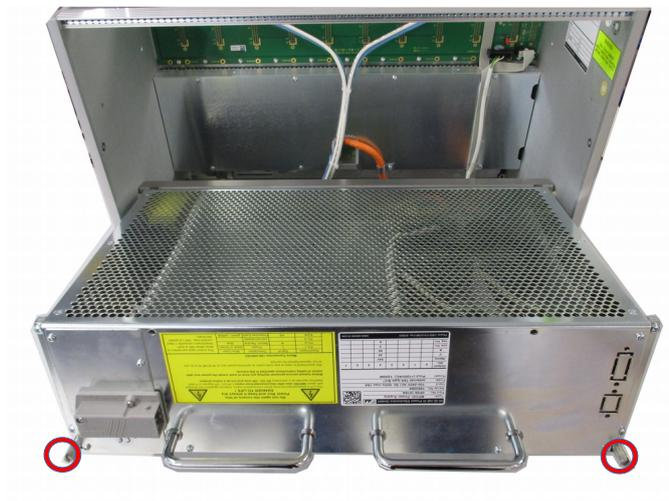
Figure 3: remove wire tie and loosen screws
