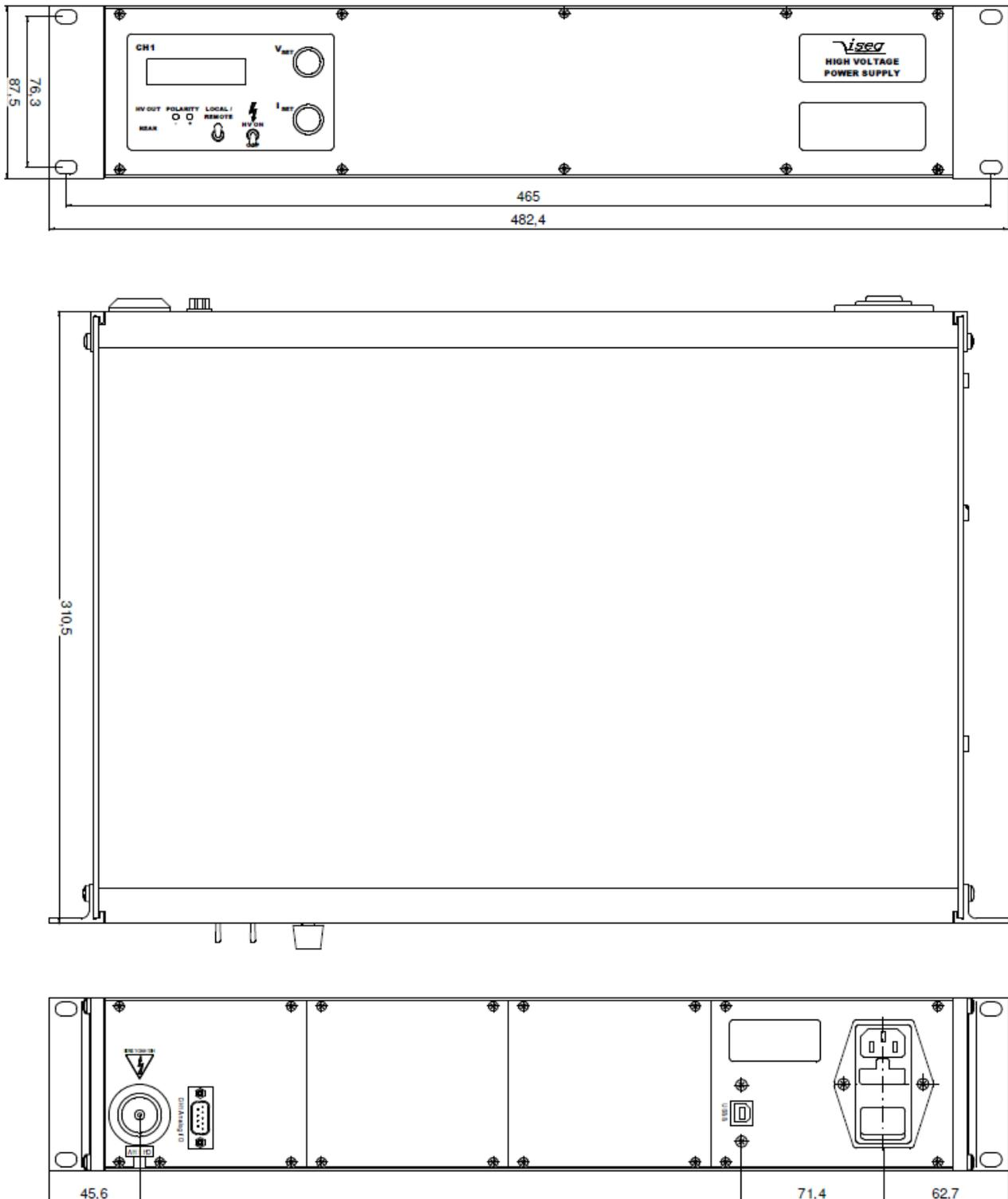
Figure 8: THQ 19 Zoll, Example for 1 Channel 30kV
