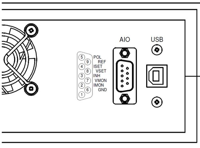
Figure 2: Example rear panel with AIO and USB
