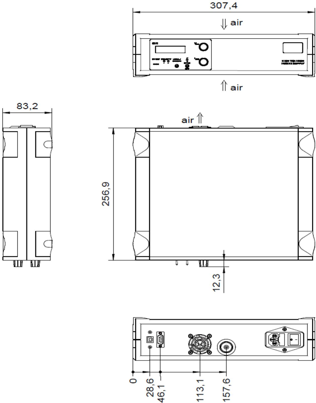
Figure 12: THQ Desktop, Example for 1 Channel 30kV
