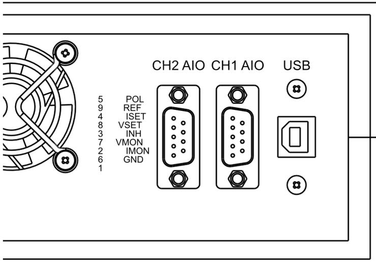
Figure 3: Rear panel with AIO and USB connectors
