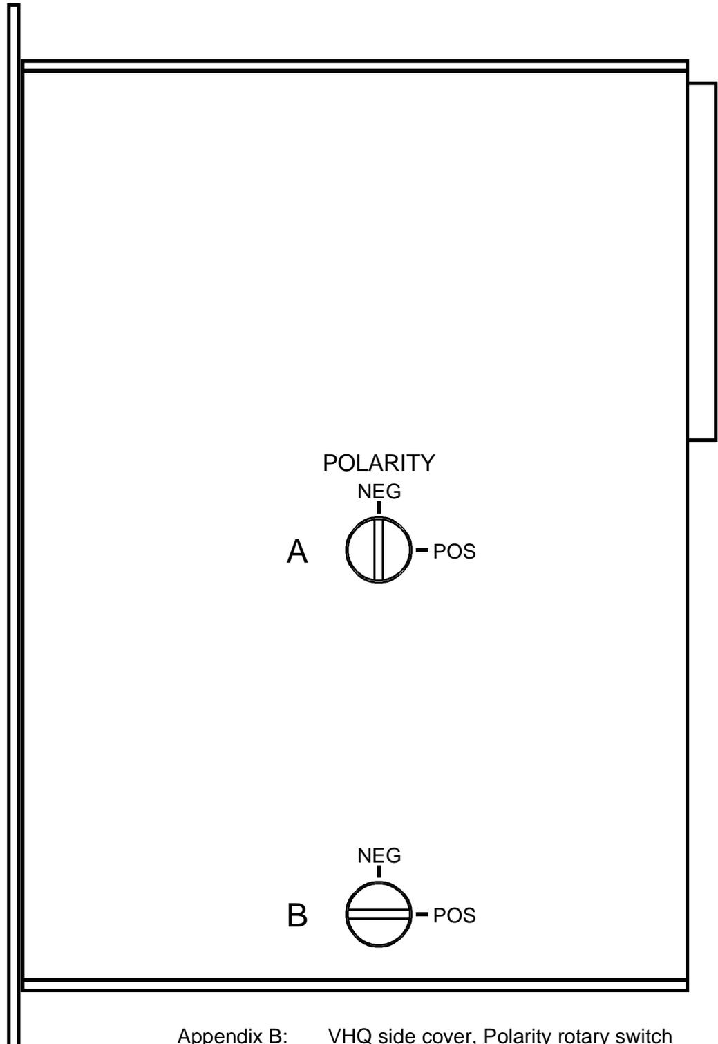
Appendix B: VHQ side cover, Polarity rotary switch
