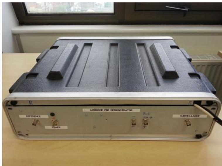
Figure 4.15: Completed receiver ready for experimental data collection - front interface
