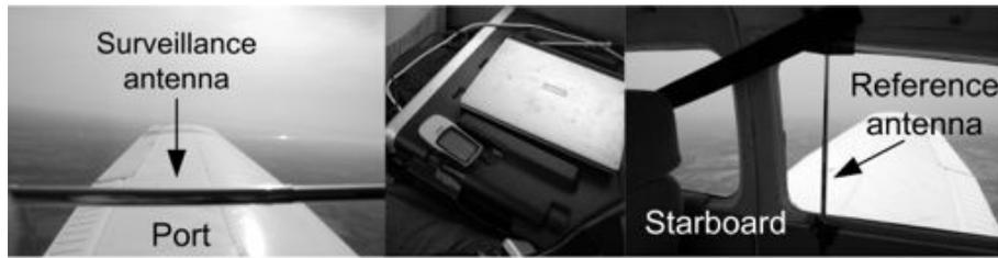
Figure 5.8: System installation in the PA 28-181.
