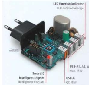
(it may be sold under various brand names). It has the additional advantage that you may supply both KrakenSDR and Pi from this single PS by connecting e.g. the Pi to the orange QC 3.0 connector and the KrakenSDR to one of the other connectors.
