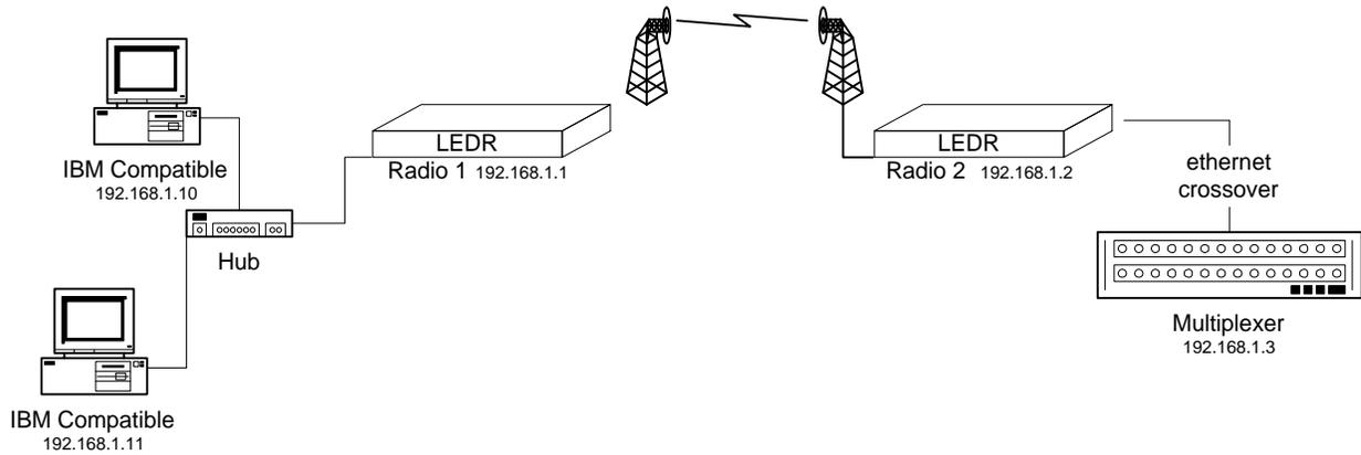
In this configuration both PC's need to send data to the mux at the far end of the radio link. Instead of adding a gateway route to each PC, Radio #1 can be configured to proxy ARP for the MUX as well as Radio #2. This can be done easily using the **arp -s** command on Radio #1. In the above example the command would be:
