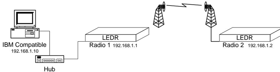
Normally, the PC would need a route added to its routing table using the first radio as a gateway to the second radio. This route would look like this:
