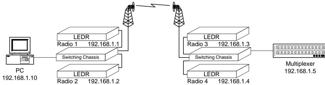
Assign each radio an IP address, netmask, default gateway, and port as follows:
