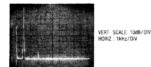
(A) Response of a 25Hz Notch Filter to a 1kHz, 1V RMS Input Sinewave
