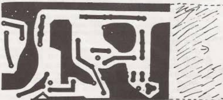
FIG. F PCB DESIGN FOR BUFFER STAGE OF OSCILLATOR. (The actual pattern you get on top side of board is mirror of this! Viewed from below. (Figs B & F on same board!)) ACTUAL SIZE
