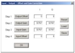
For baseband modem chipset designers, deliberately introducing I/Q impairments can stress test a chipset's performance. Fine I/Q balancing capability can also be used to compensate for input and output signal offsets, as well as for internal calibration routines.
