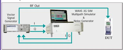
Combining WAVE-3G SIM with a Base Station Emulator and Vector Signal Generator yields a powerful and comprehensive 3G mobile test solution. Since a digital power meter enables accurate and
