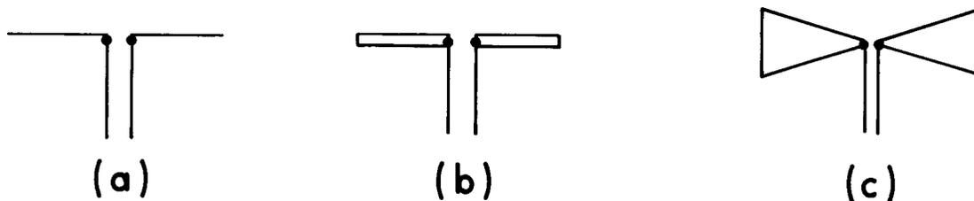
Figure 3.41. Short dipole used to sense the presence of an electric field.
