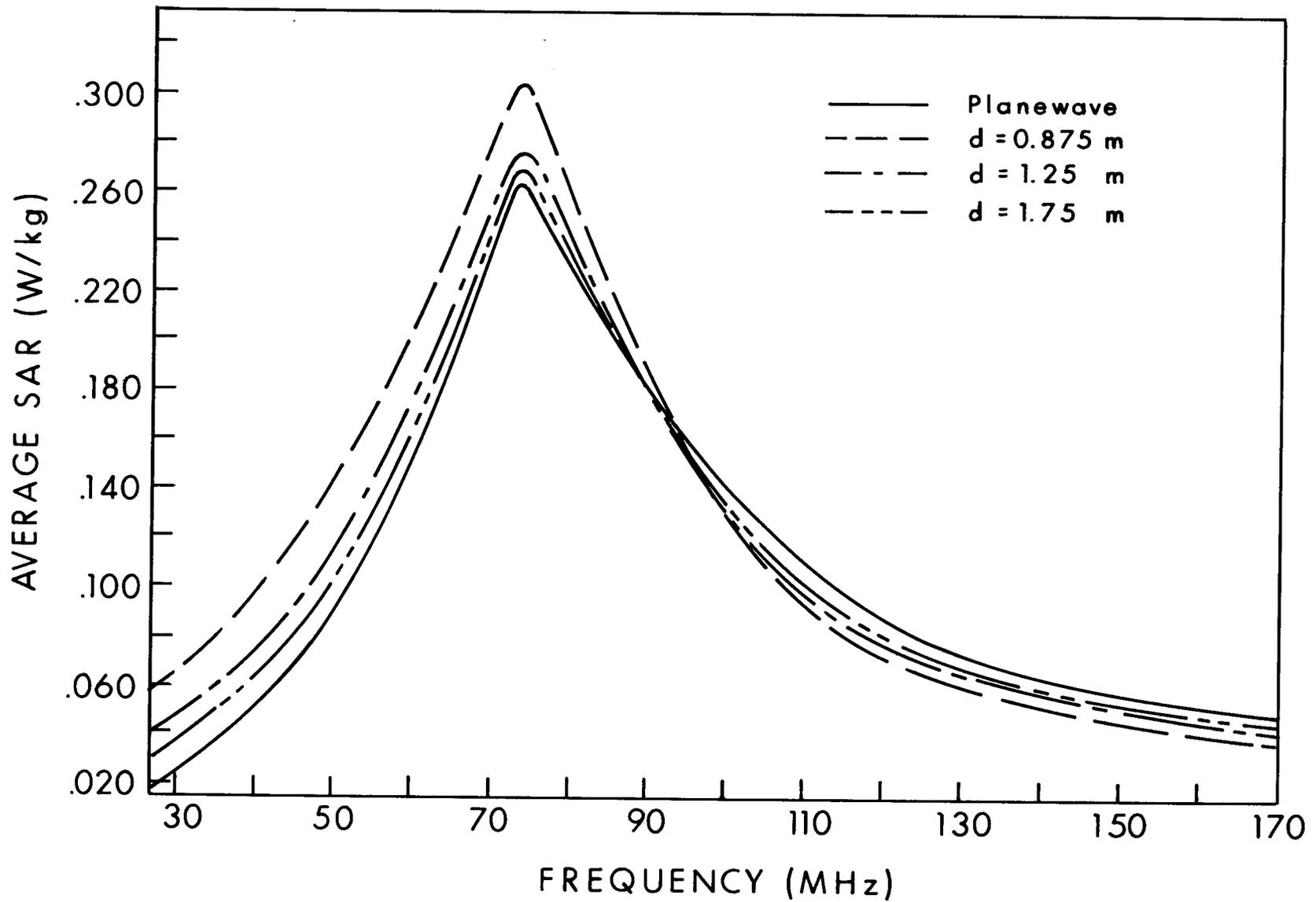
Figure 6.42. Calculated average SAR in a prolate spheroidal model of an average man irradiated by the near fields of a small magnetic dipole, as a function of the dipole-to-body spacing,  $d$ .
