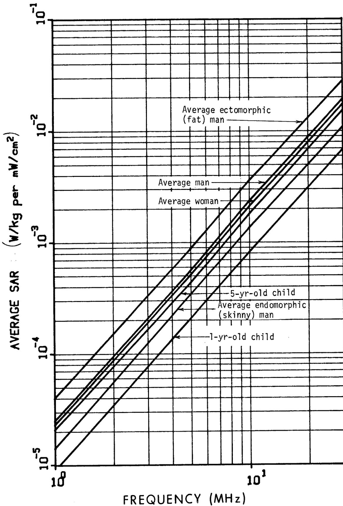
Figure 6.2. Calculated planewave average SAR in ellipsoidal models of different human-body types, EKH polarization.
