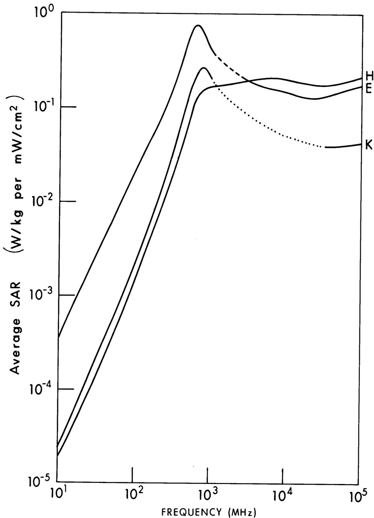
Figure 3.40. Calculated whole-body average SAR versus frequency for models of a medium-sized rat for three standard polarizations. The incident-power density is  $1 \text{ mW/cm}^2$ .
