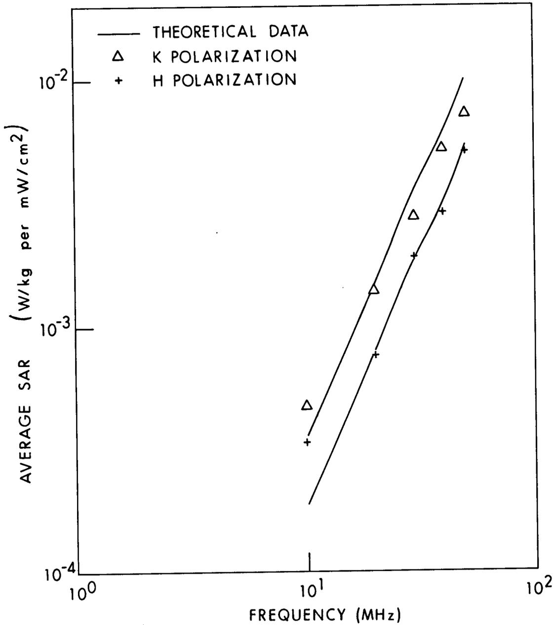
Figure 8.2. Calculated and measured values of the average SAR for a human prolate spheroidal phantom;  $a = 0.875$  m,  $b = 0.138$  m,  $V = 0.07$  m<sup>3</sup> (Allen et al., 1975).
