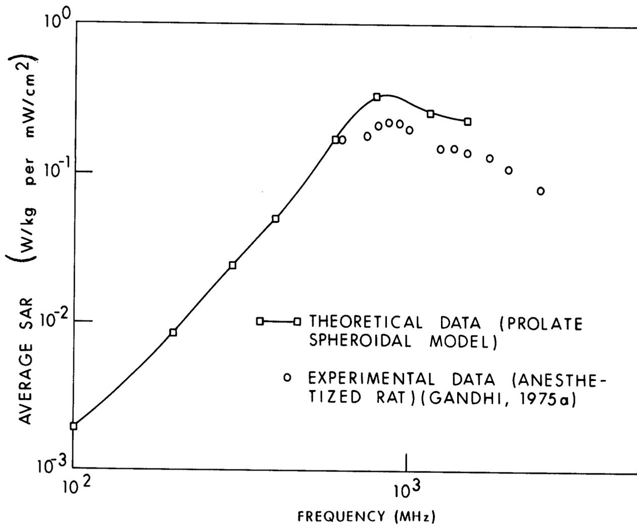
Figure 8.11. Calculated and measured values of the average SAR for a 261-g rat, K polarization.
