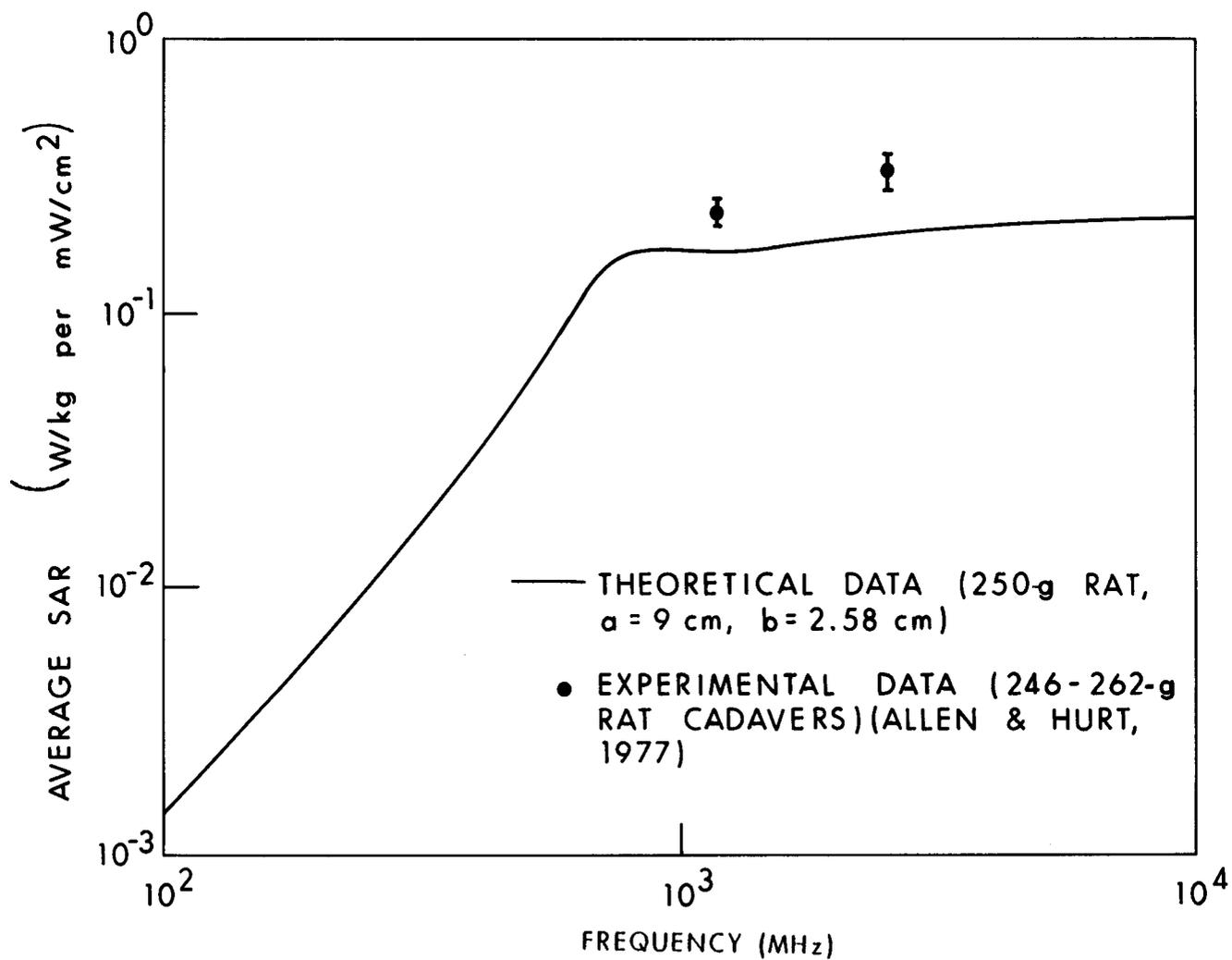
Figure 8.13. Calculated and measured values of the average SAR for models of a rat, H polarization.
