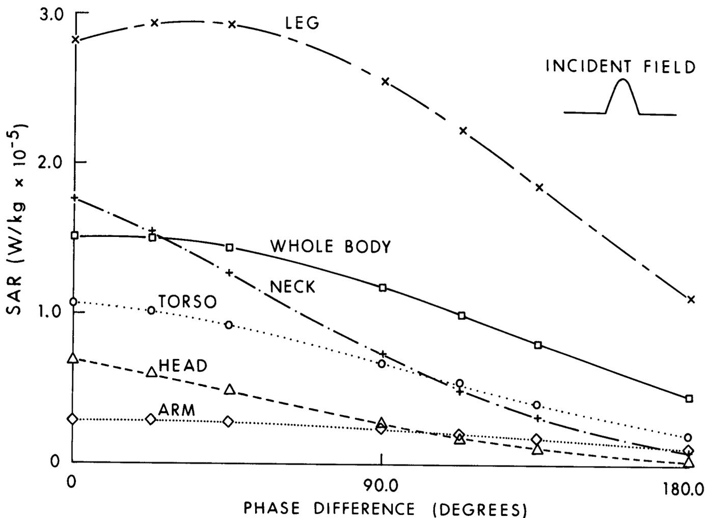
Figure 6.47. Whole- and part-body SAR at 77 MHz in the block model of man as a function of an assumed linear antisymmetric phase variation in the incident  $E_z$ ;  $E_z|_{\max} = 1 \text{ V/m}$ . Calculated by Chatterjee et al. (1980a, 1980b, 1980c).
