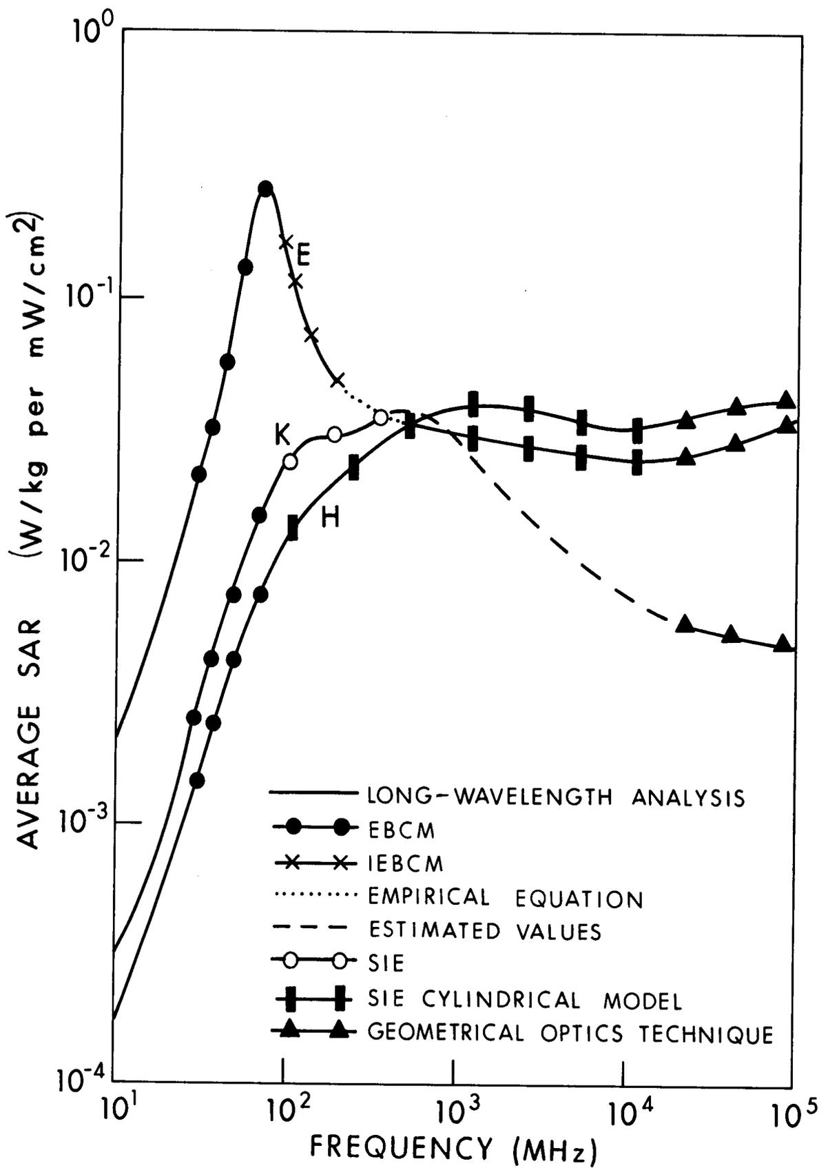
Figure 5.1. Illustration of different techniques, with their frequency limits, used for calculating SAR data for models of an average man.
