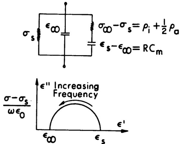
Figure 4.4. Equivalent circuit for the  $\beta$ -dispersion of a cell suspension and corresponding plot in the complex dielectric constant plane (Schwan and Foster, 1980).
