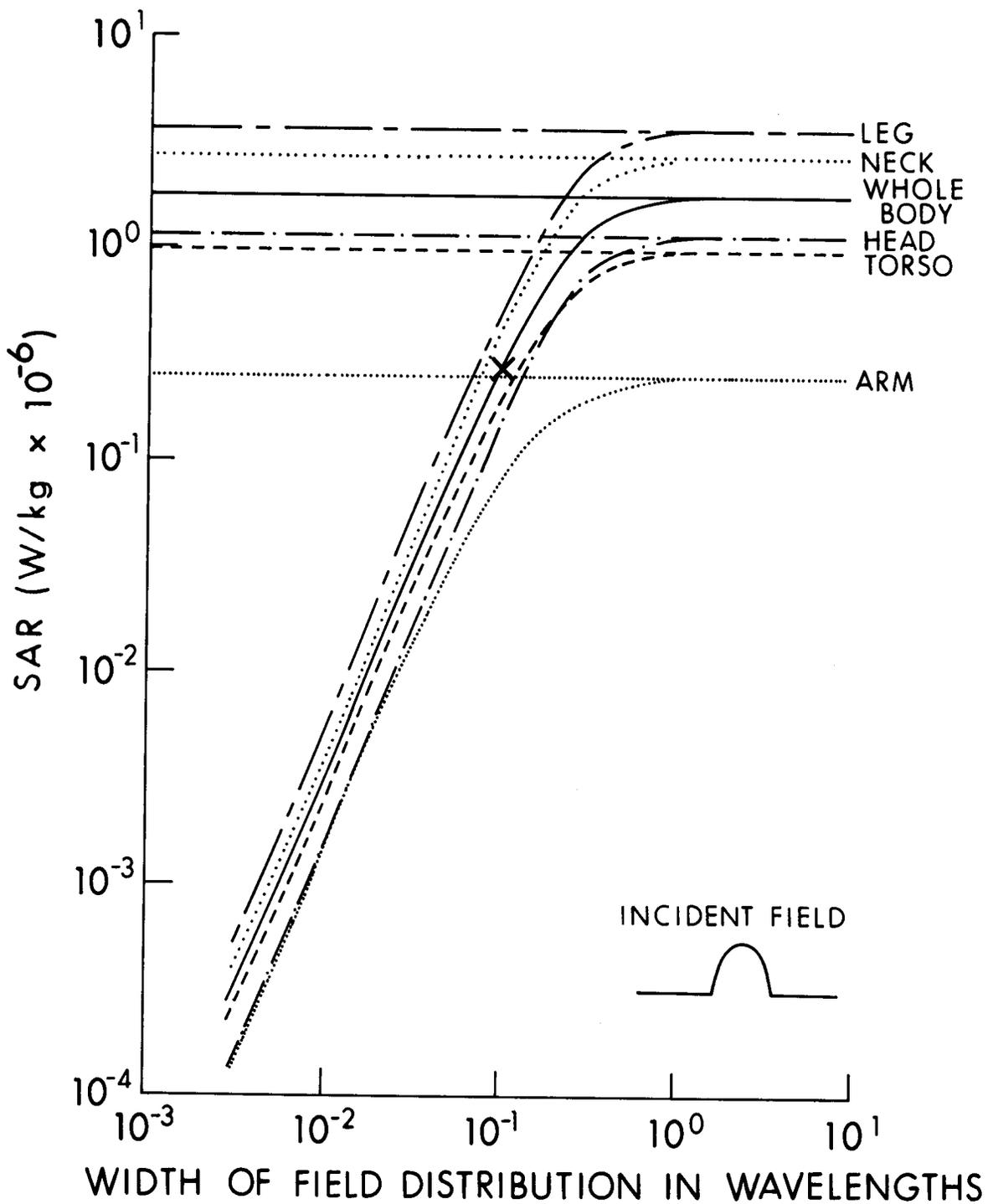
Figure 6.45. Average whole- and part-body SAR in the block model of man placed in front of a half-cycle cosine field,  $E_z$ ; frequency = 27.12 MHz,  $E_z |_{\text{max}} = 1$  V/m. Calculated by Chatterjee et al. (1980a, 1980b, 1980c).
