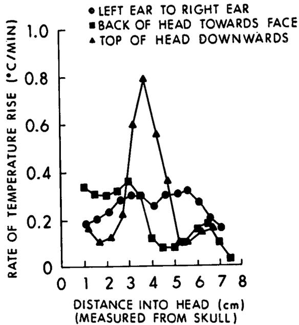
Figure 8.27. Rate of temperature rise from RFR exposure at the back of a detached *M. mulatta* head; 1.2 GHz, CW, 70 mW/cm<sup>2</sup>, far field (Burr and Krupp, 1980).
