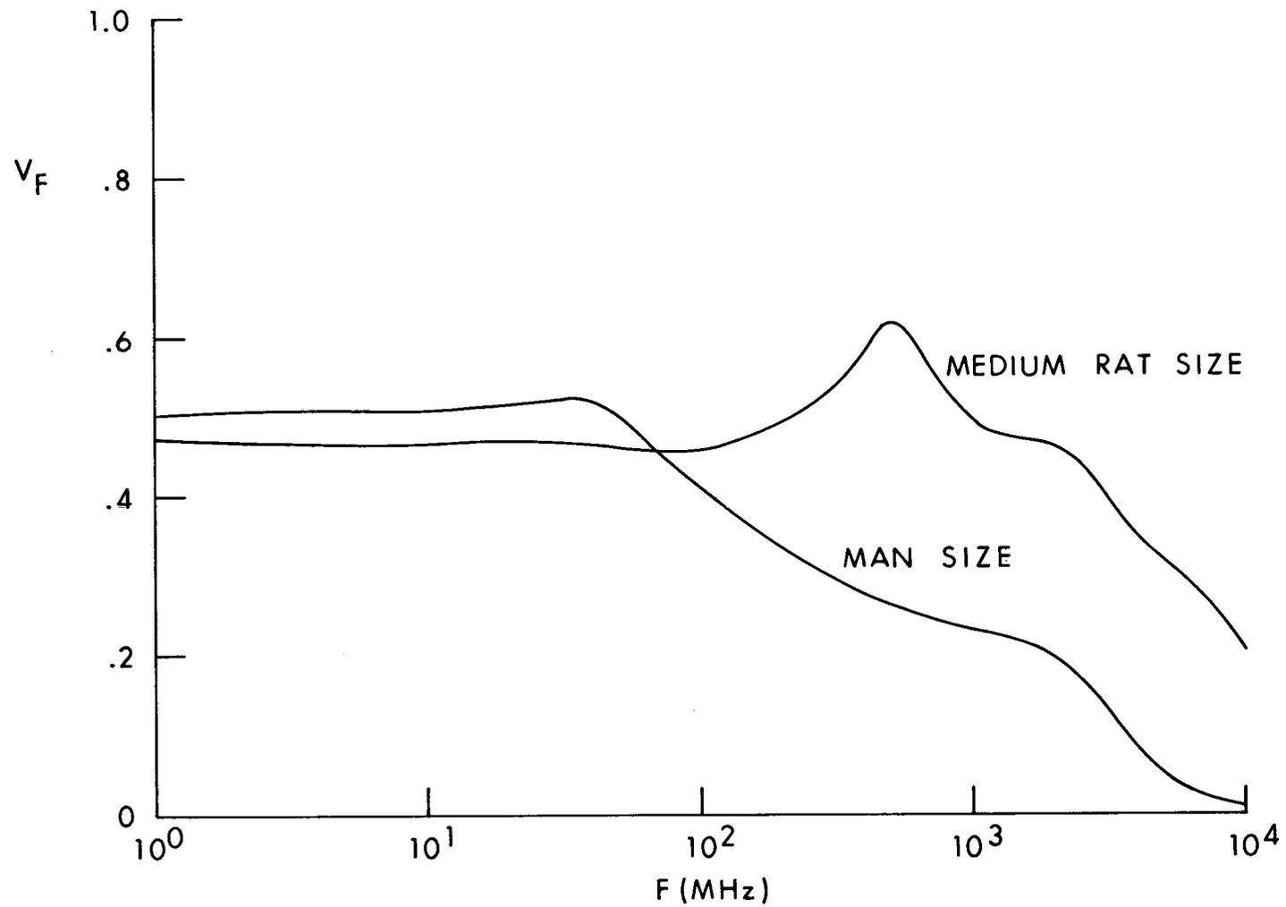
Figure 5.6. The volume fraction,  $V_F$ , as a function of frequency for two spheres of muscle material.  $V_F$  is the fraction of the volume in which 90% of the power is absorbed (see p. 5.15).
