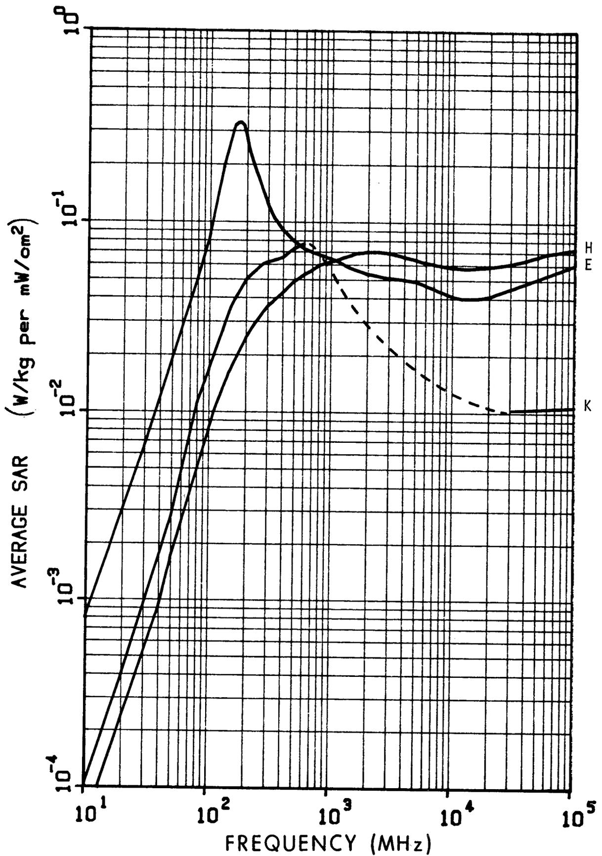
Figure 6.9. Calculated planewave average SAR in a prolate spheroidal model of a 1-year-old child for three polarizations;  $a = 0.37$  m,  $b = 0.08$  m,  $V = 0.01$  m<sup>3</sup>. The dashed line is estimated values.
