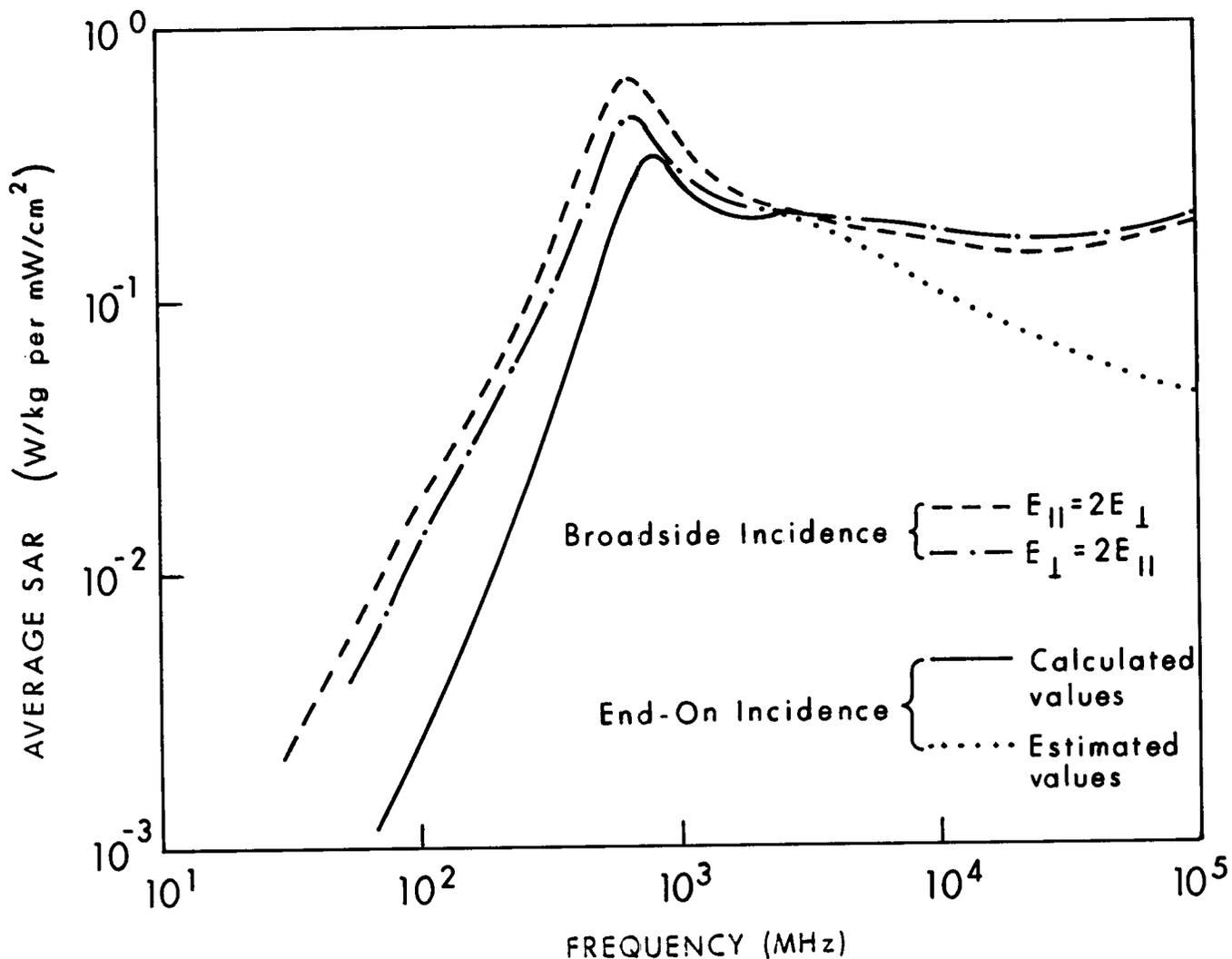
Figure 6.30. Calculated planewave average SAR in a prolate spheroidal model of a medium rat irradiated by an elliptically polarized wave,<sup>3</sup> for two orientations;  $a = 0.1$  m,  $b = 0.0276$  m,  $V = 3.2 \times 10^{-4}$  m<sup>3</sup>.
