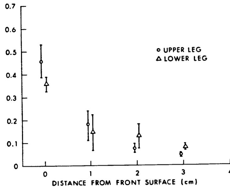
Figure 8.24. Normalized microwave absorption profiles in man-size model at 2.0 GHz. Vertical bars represent  $\pm 1$  SD of the mean SAR. Minimum N, 3; average N, 5 (Olsen, 1982).
