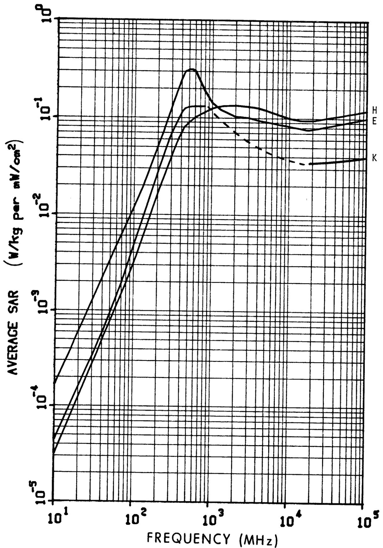
Figure 6.11. Calculated planewave average SAR in a prolate spheroidal model of a squirrel monkey for three polarizations;  $a = 0.115$  m,  $b = 0.0478$  m,  $V = 1.1 \times 10^{-3}$  m<sup>3</sup>. The dashed line is estimated values.
