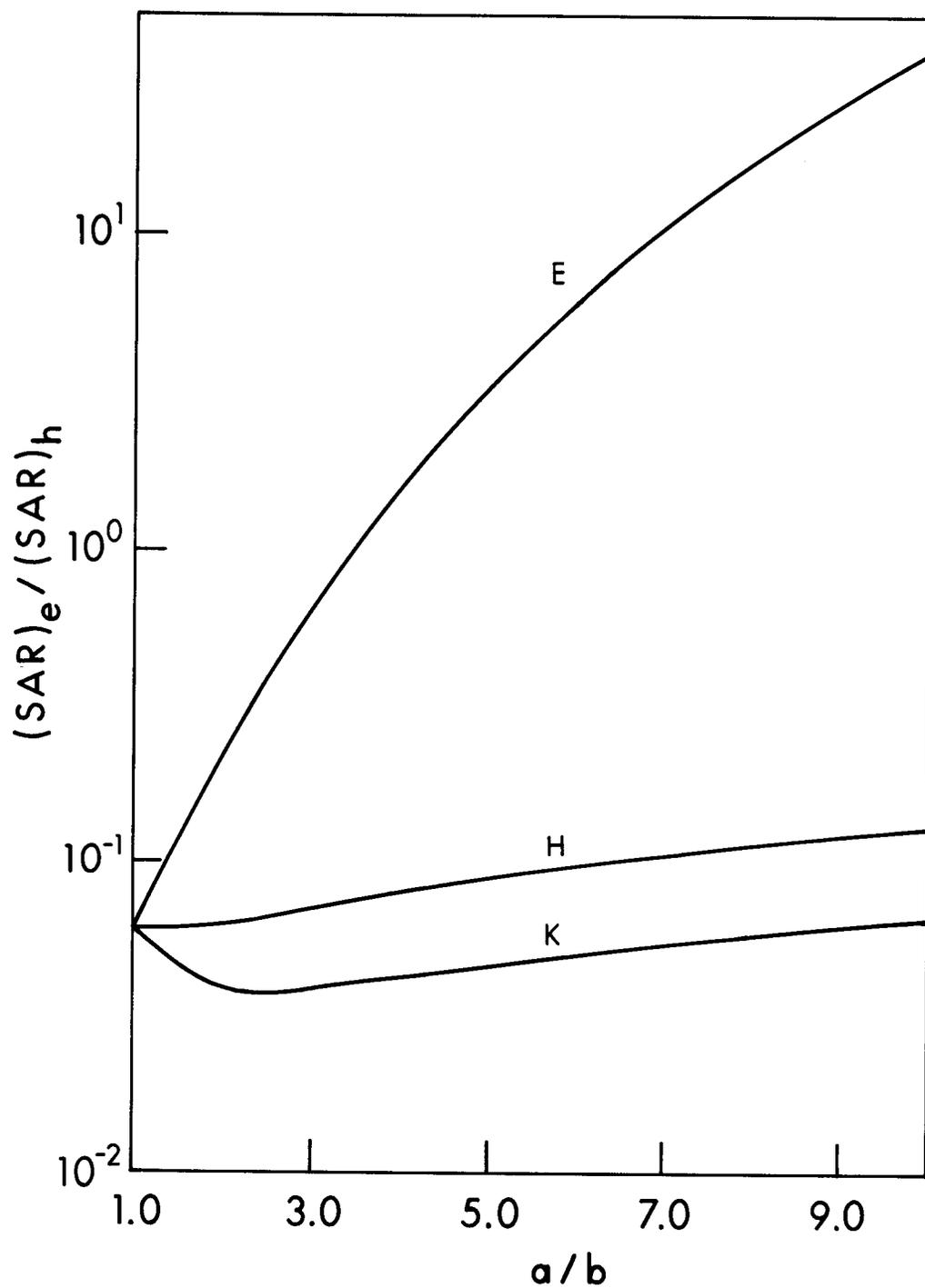
Figure 5.14. Ratio of  $(SAR)_e$  to  $(SAR)_h$  of a  $0.07\text{-m}^3$  prolate spheroid for each polarization as a function of the ratio of the major axis to the minor axis of the spheroid at 27.12 MHz,  $\sigma = 0.4$  S/m.
