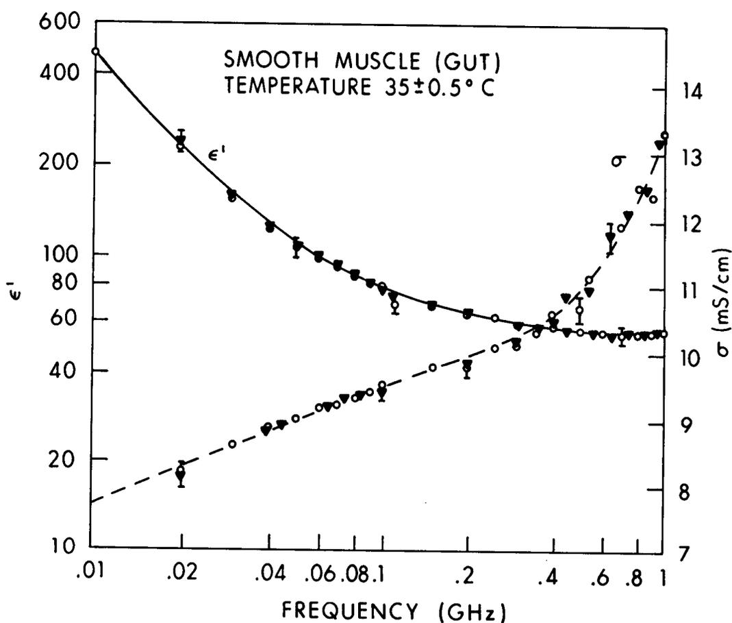
Figure 4.20. Relative permittivity of cat smooth muscle in vivo:  $\blacktriangledown$  and  $\circ$  show results obtained for two locations in the tissue. The vertical bars show the uncertainty due to the estimated measurement errors (SD) (Stuchly et al., 1981).
