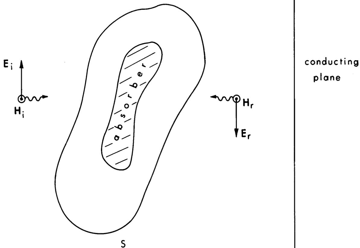
Figure 3.29. Absorber placed between an incident plane wave and a conducting plane.
