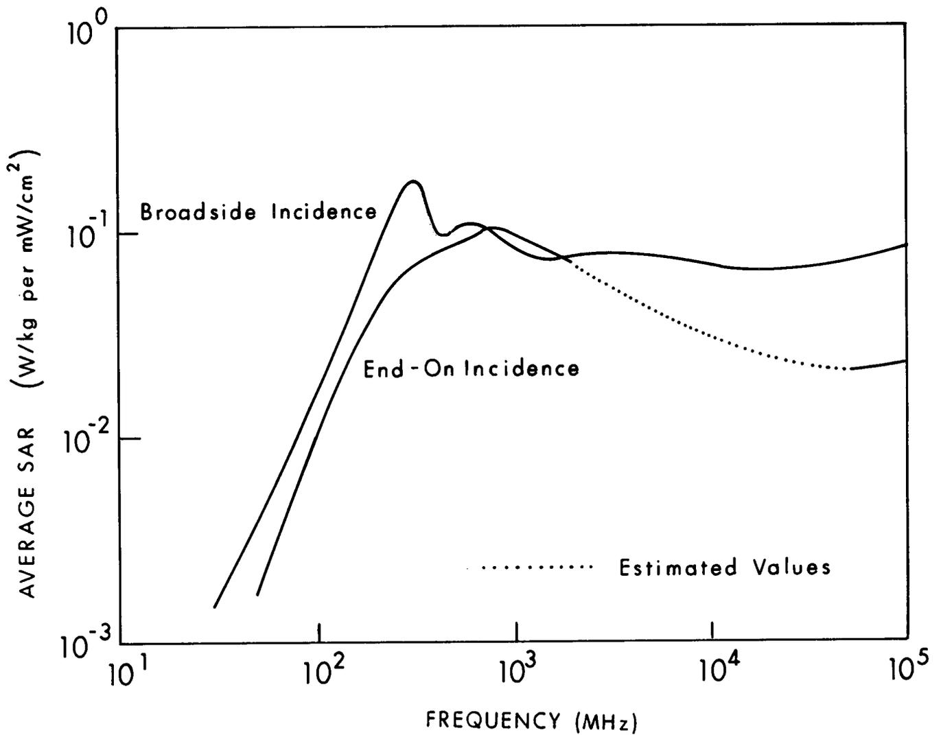
Figure 6.26. Calculated planewave average SAR in a prolate spheroidal model of a sitting rhesus monkey irradiated by a circularly polarized wave, for two orientations;  $a = 0.2$  m,  $b = 0.0646$  m,  $V = 3.5 \times 10^{-3}$  m<sup>3</sup>.
