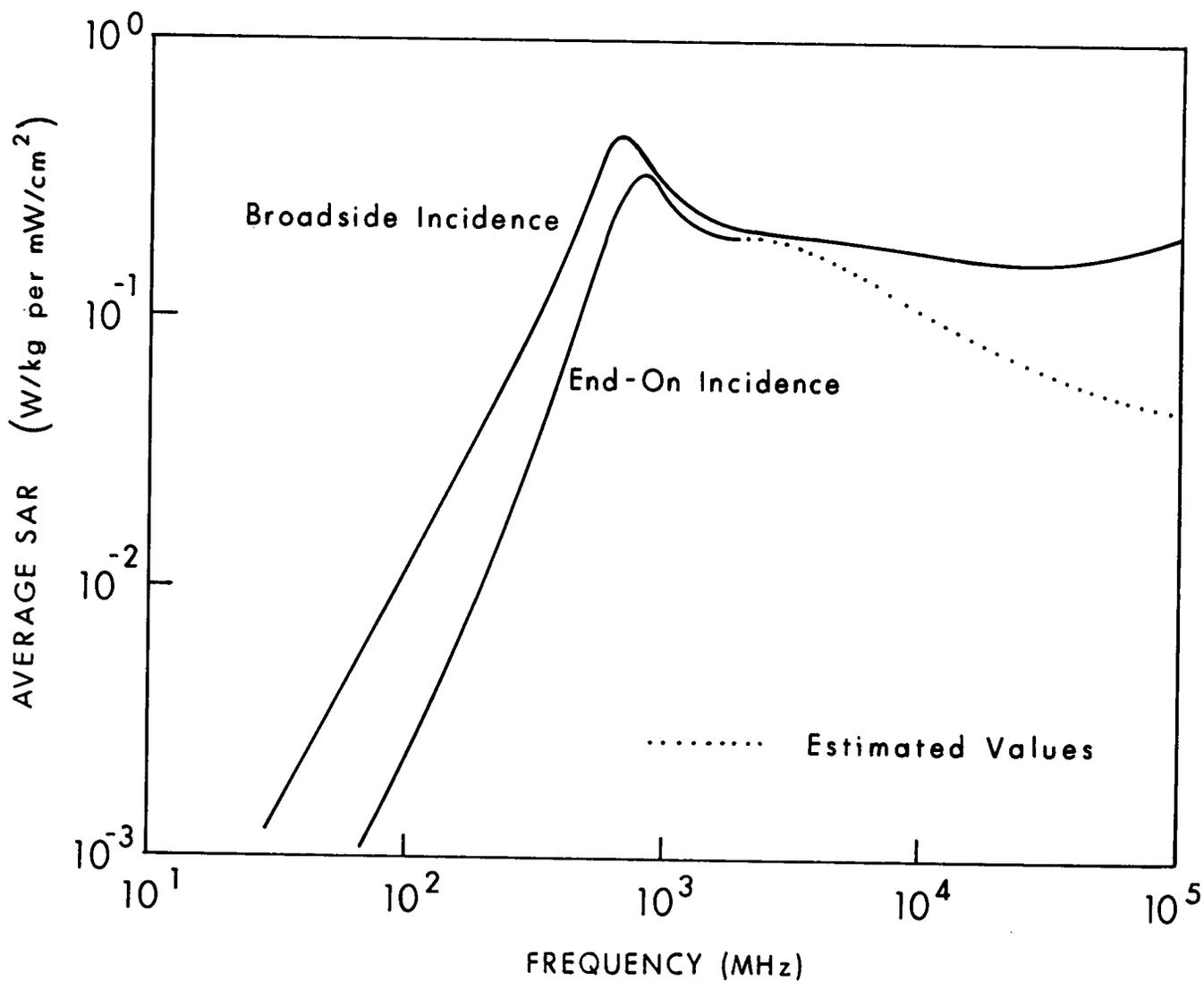
Figure 6.27. Calculated planewave average SAR in a prolate spheroidal model of a medium rat irradiated by a circularly polarized wave, for two orientations;  $a = 0.1$  m,  $b = 0.0276$  m,  $V = 3.2 \times 10^{-4}$  m<sup>3</sup>.
