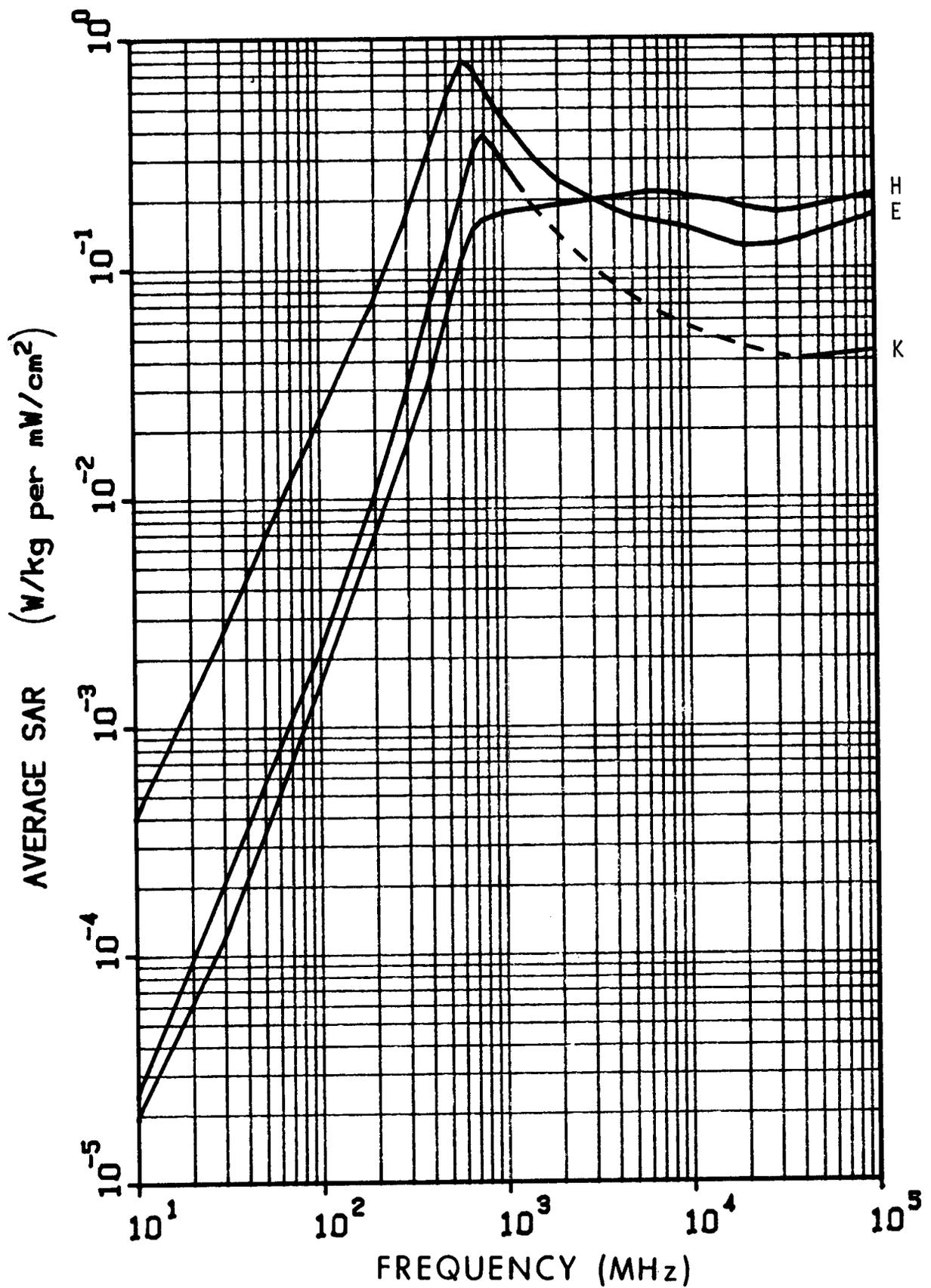
Figure 6.16. Calculated plane-wave average SAR in a prolate spheroidal model of a medium rat for three polarizations;  $a = 0.1$  m,  $b = 0.0276$  m,  $V = 3.2 \times 10^{-4}$  m<sup>3</sup>. The dashed line is estimated values.
