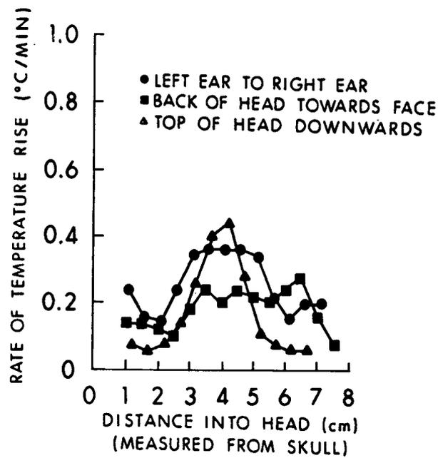
Figure 8.25. Rate of temperature rise from RFR exposure in the face of a detached *M. mulatta* head; 1.2 GHz, CW, 70 mW/cm<sup>2</sup>, far field (Burr and Krupp, 1980).
