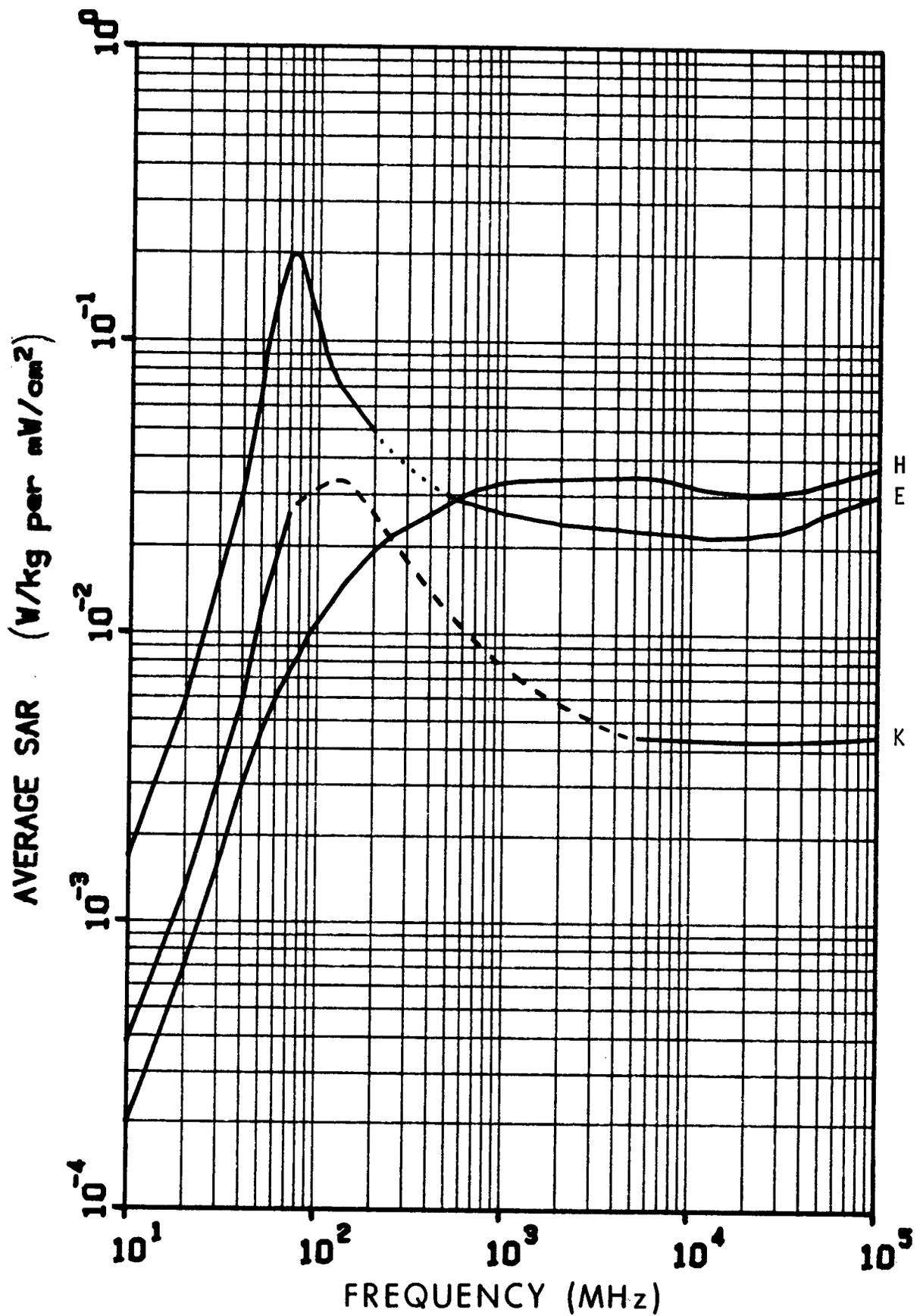
Figure 6.7. Calculated planewave average SAR in a prolate spheroidal model of a large woman for three polarizations;  $a = 0.865$  m,  $b = 0.156$  m,  $V = 0.08845$  m<sup>3</sup>. The dotted line is calculated from Equation 5.1; the dashed line is estimated values.
