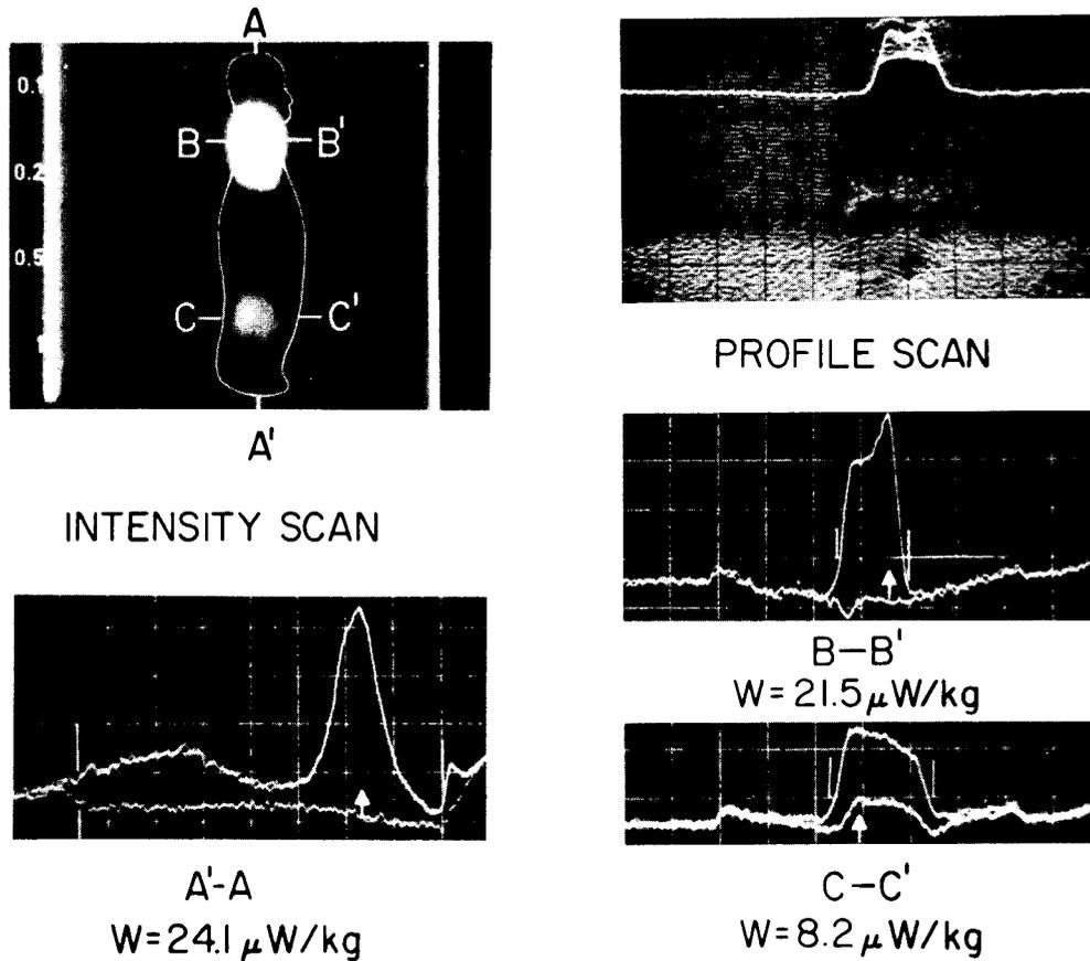
Figure 8.39. Scale-model thermograms and measured peak SAR for 70-kg, 1.74-m-height medial-plane man model exposed to 31.0-MHz electric field parallel to the major axis: vertical divergence =  $2^\circ\text{C}$ , horizontal divergence = 2.65 cm (Guy et al., 1976b) (© 1976 IEEE).
