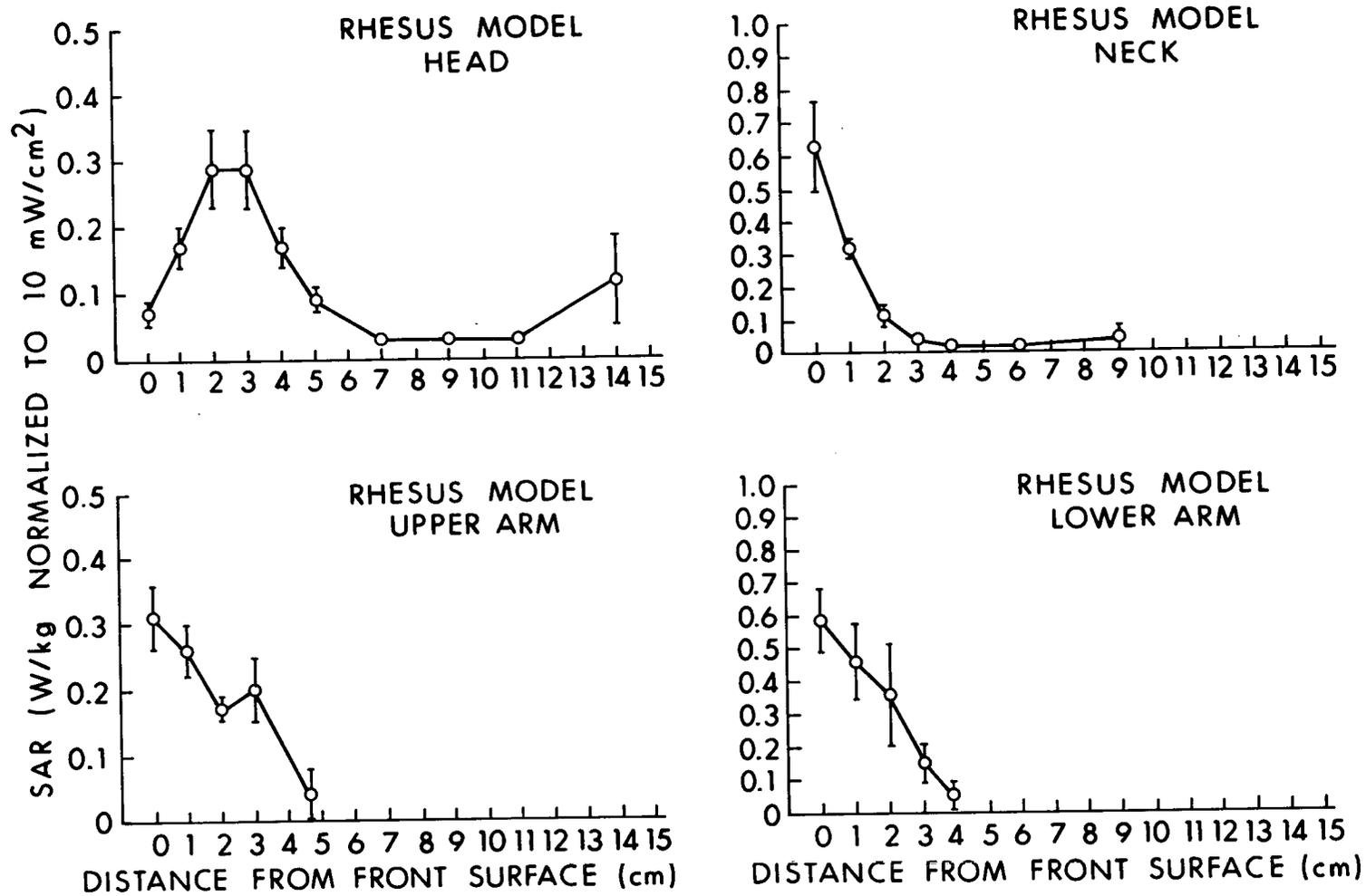
Figure 8.22. Microwave absorption profiles for rhesus monkey model. Irradiation frequency was 1.29 GHz. Vertical bars represent  $\pm$  in the calculated value of the SAR (Olsen et al., 1980).
