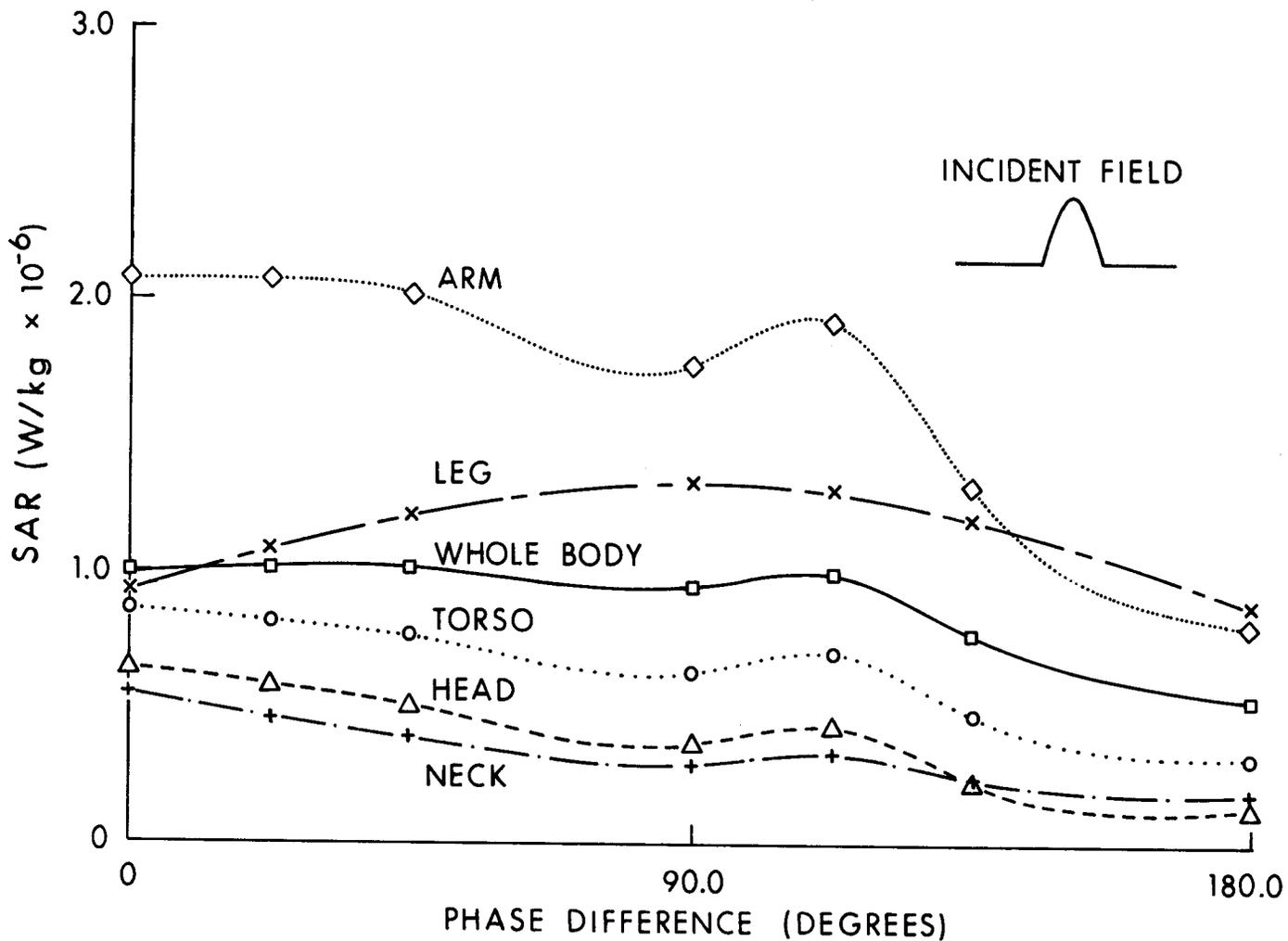
Figure 6.49. Whole- and part-body SAR at 350 MHz in the block model of man as a function of an assumed linear antisymmetric phase variation in the incident  $E_z$ ;  $E_z|_{\max} = 1 \text{ V/m}$ . Calculated by Chatterjee et al. (1980a, 1980b, 1980c).
