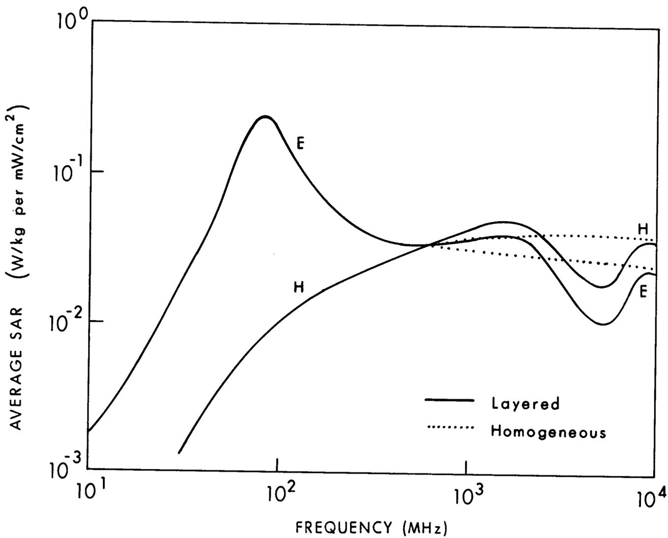
Figure 6.21. Calculated planewave average SAR in homogeneous and multi-layered models of an average woman for two polarizations.
