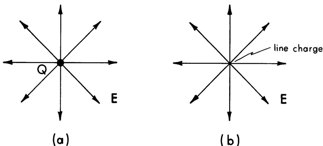
Figure 3.8. (a)  $\mathbf{E}$ -field produced by one point charge,  $Q$ , in space.
