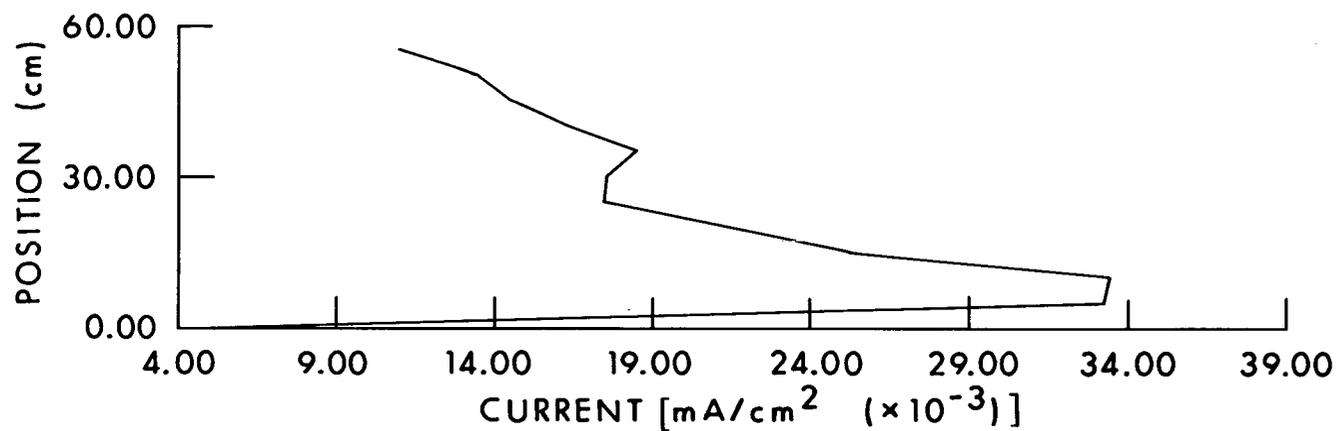
Figure 9.17. Calculated current density flowing through one arm. Exposure condition is same as for Fig. 9.16 (Guy and Chou, 1982).
