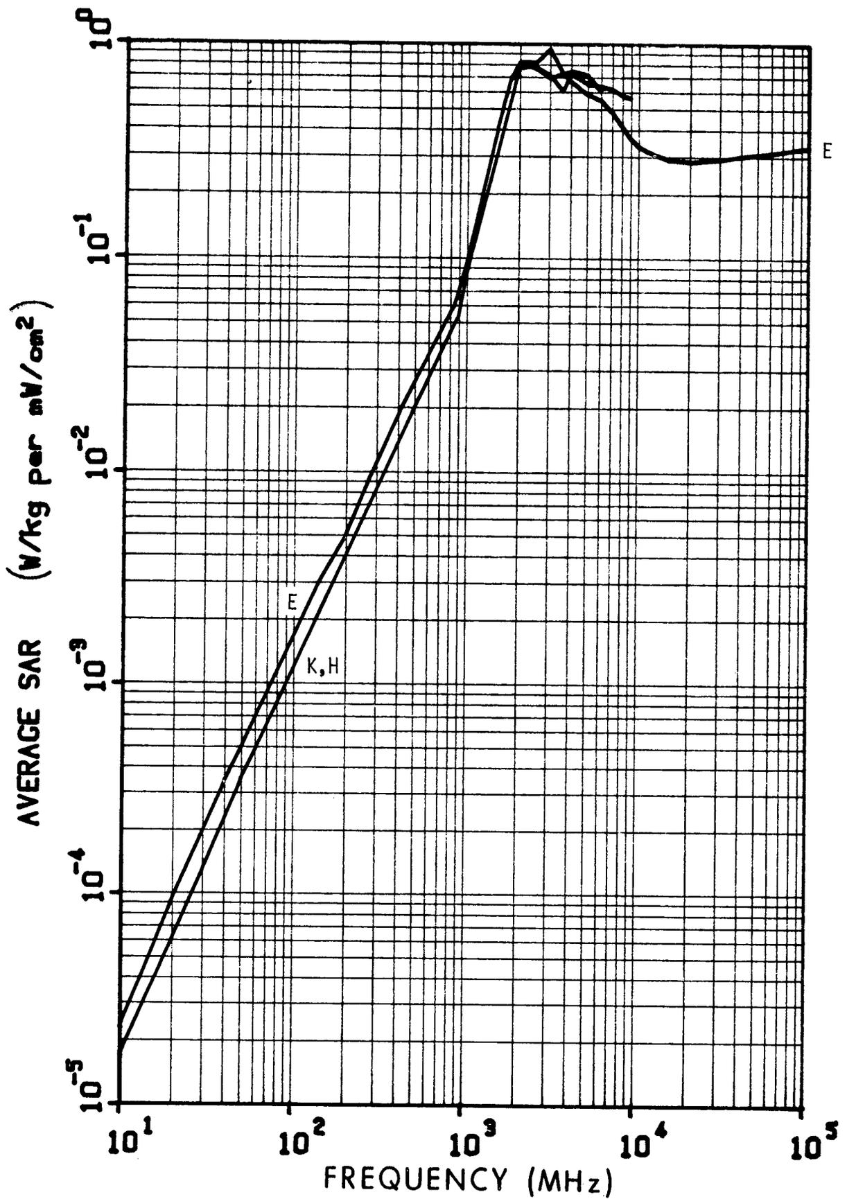
Figure 6.19. Calculated planewave average SAR in a prolate spheroidal model of a quail egg for three polarizations;  $a = 1.5$  cm,  $b = 1.26$  cm, and  $V = 10$  cm<sup>3</sup>.
