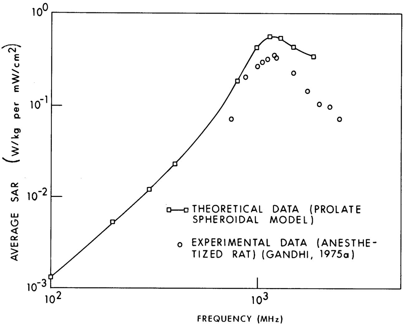
Figure 8.9. Calculated and measured values of the average SAR for a 96-g rat, K polarization.
