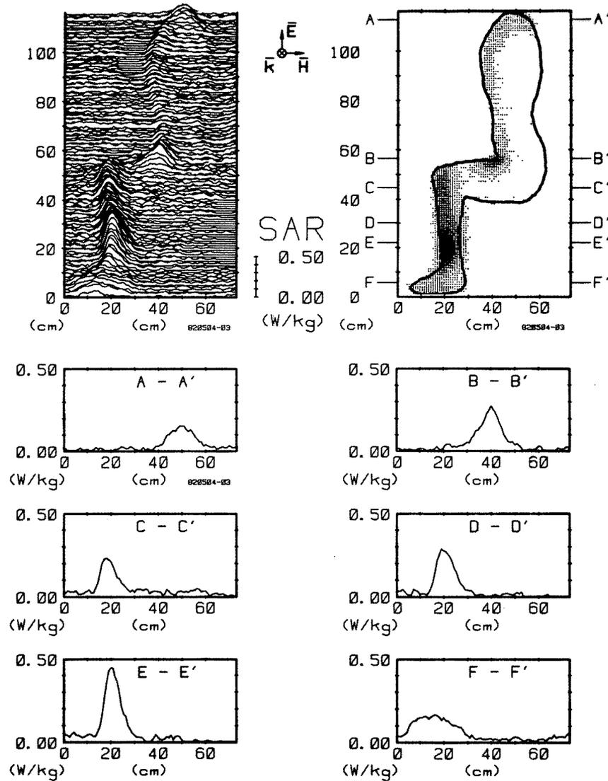
Figure 8.46. Computer-processed whole-body thermograms expressing SAR patterns for man sitting (sagittal plane through leg), exposed to 1-mW/cm<sup>2</sup> 450-MHz radiation with EHK polarization (Guy et al., 1984) (© 1984 IEEE).
