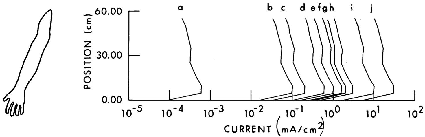
Figure 9.15. Calculated current density flowing through one arm. Exposure condition is the same as for Figure 9.14 (Guy and Chou, 1982).
