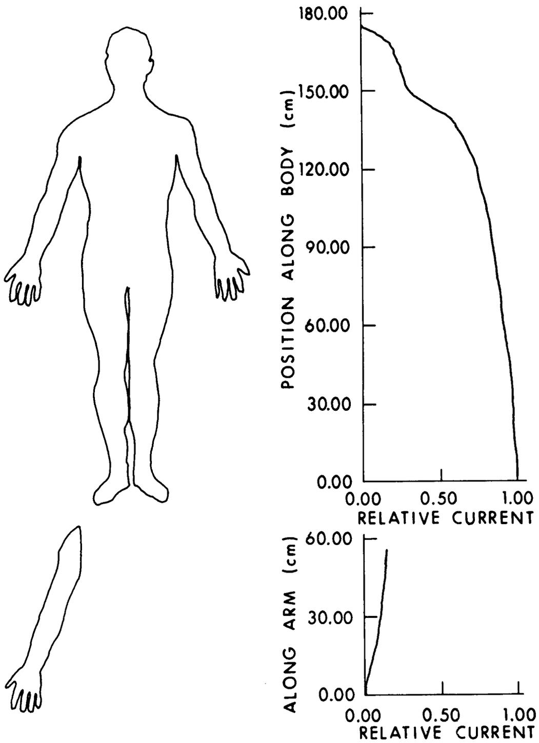
Figure 9.2. Relative surface-current distribution in grounded man exposed to VLF-MF fields [after Deno, 1977 (Guy and Chou, 1982)].
