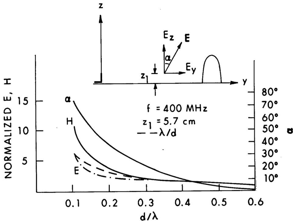
Figure 8.21. Measured relative fields versus distance for the thick monopole on a ground plane. The values of  $E$  and  $H$  are normalized with respect to their values at  $d/\lambda = 0.6$  (Iskander et al., 1981).
