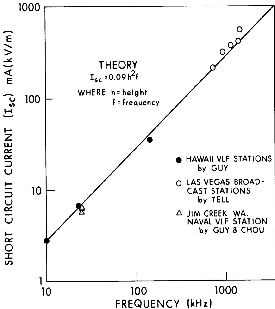
Figure 9.5. Comparison of theoretical and measured short-circuit body current of grounded man exposed to VLF-MF electric field that is parallel to body axis (Guy and Chou, 1982).
