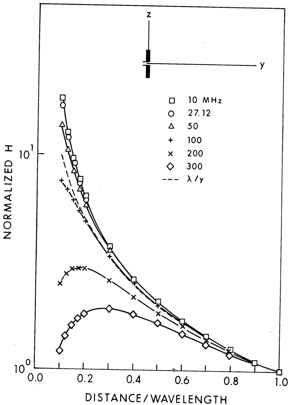
Figure 6.38. Calculated normalized H-field of a short electric dipole, as a function of  $y/\lambda$  at  $z = 30$  cm.
