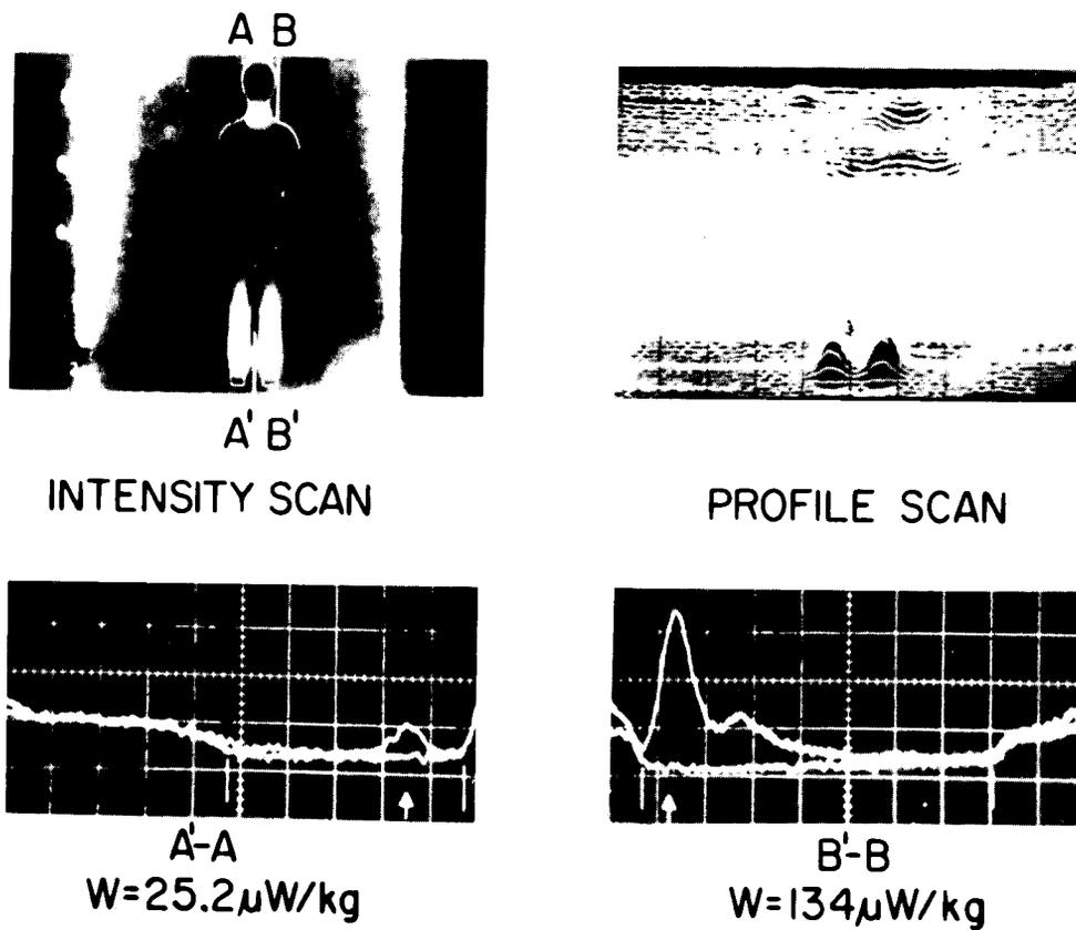
Figure 8.36. Scale-model thermograms and measured peak SAR for 70-kg, 1.74-m-height frontal-plane man model exposed to 31.0-MHz electric field parallel to the long axis: vertical divergence = 2°C, horizontal divergence = 4 cm (Guy et al., 1976b) (© 1976 IEEE).
