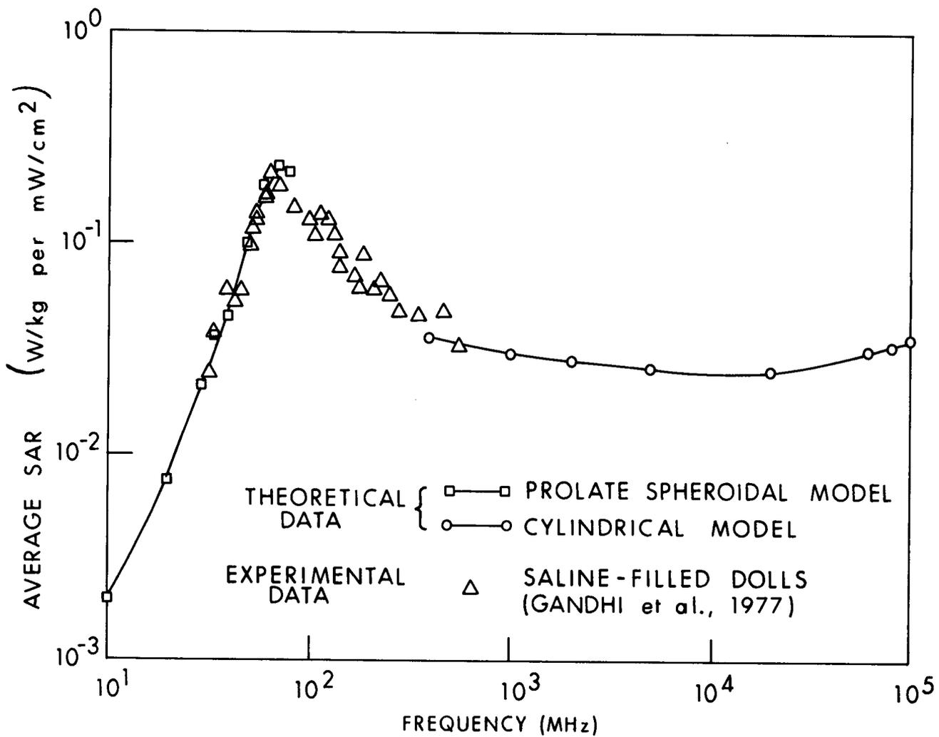
Figure 8.1A. Comparison of measured (experimental) and calculated (theoretical) SAR values for an average man in free space, E polarization.
