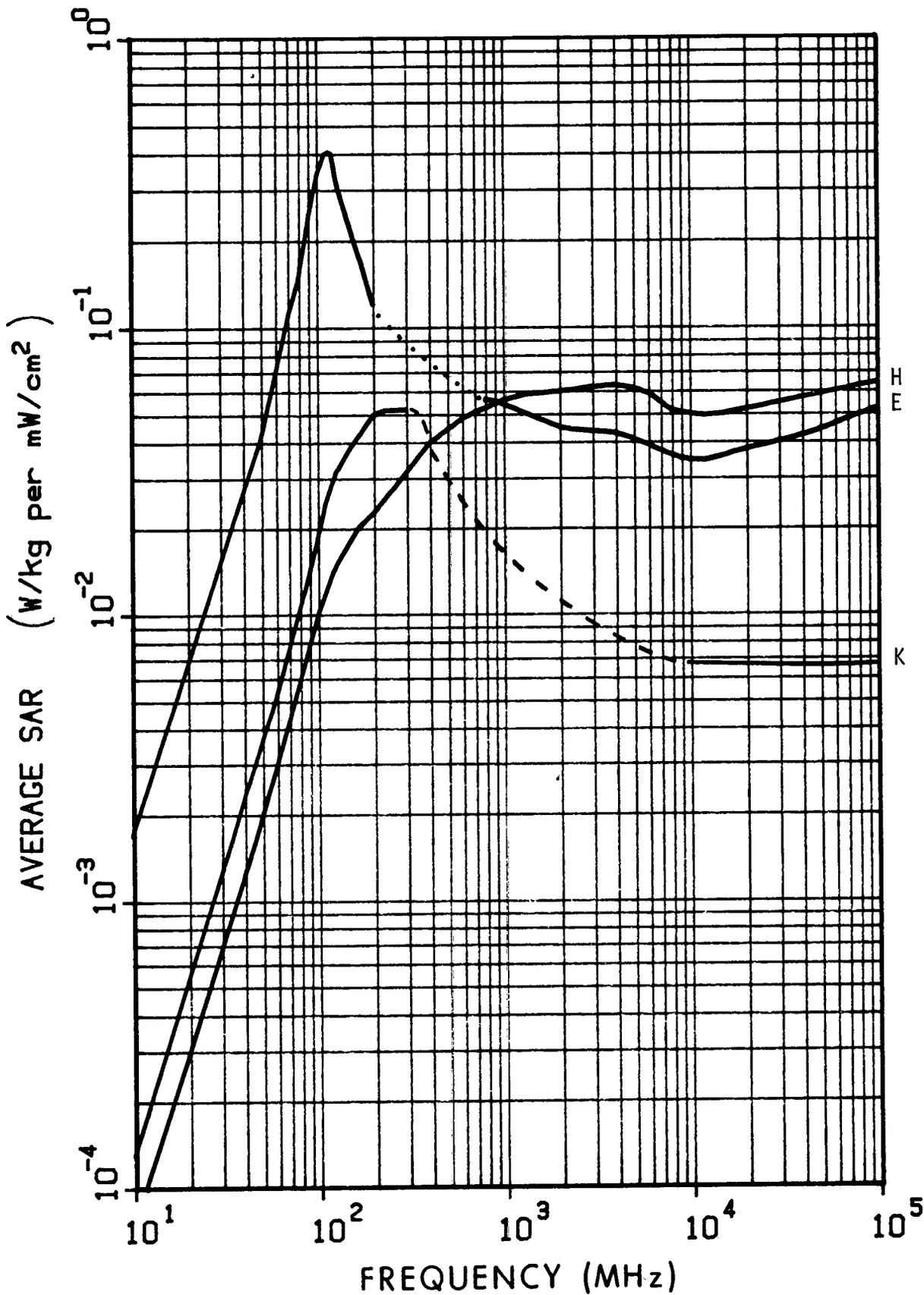
Figure 6.8. Calculated planewave average SAR in a prolate spheroidal model of a 5-year-old child for three polarizations;  $a = 0.56$  m,  $b = 0.091$  m,  $V = 0.0195$  m<sup>3</sup>. The dotted line is calculated from Equation 5.1; the dashed line is estimated values.
