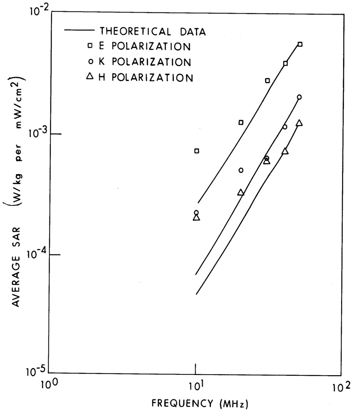
Figure 8.3. Calculated and measured values of the average SAR for a prolate spheroidal phantom of a sitting rhesus monkey;  $a = 0.2$  m,  $b = 6.46$  cm,  $V = 3.5 \times 10^{-3}$  m<sup>3</sup> (Allen et al., 1975).
