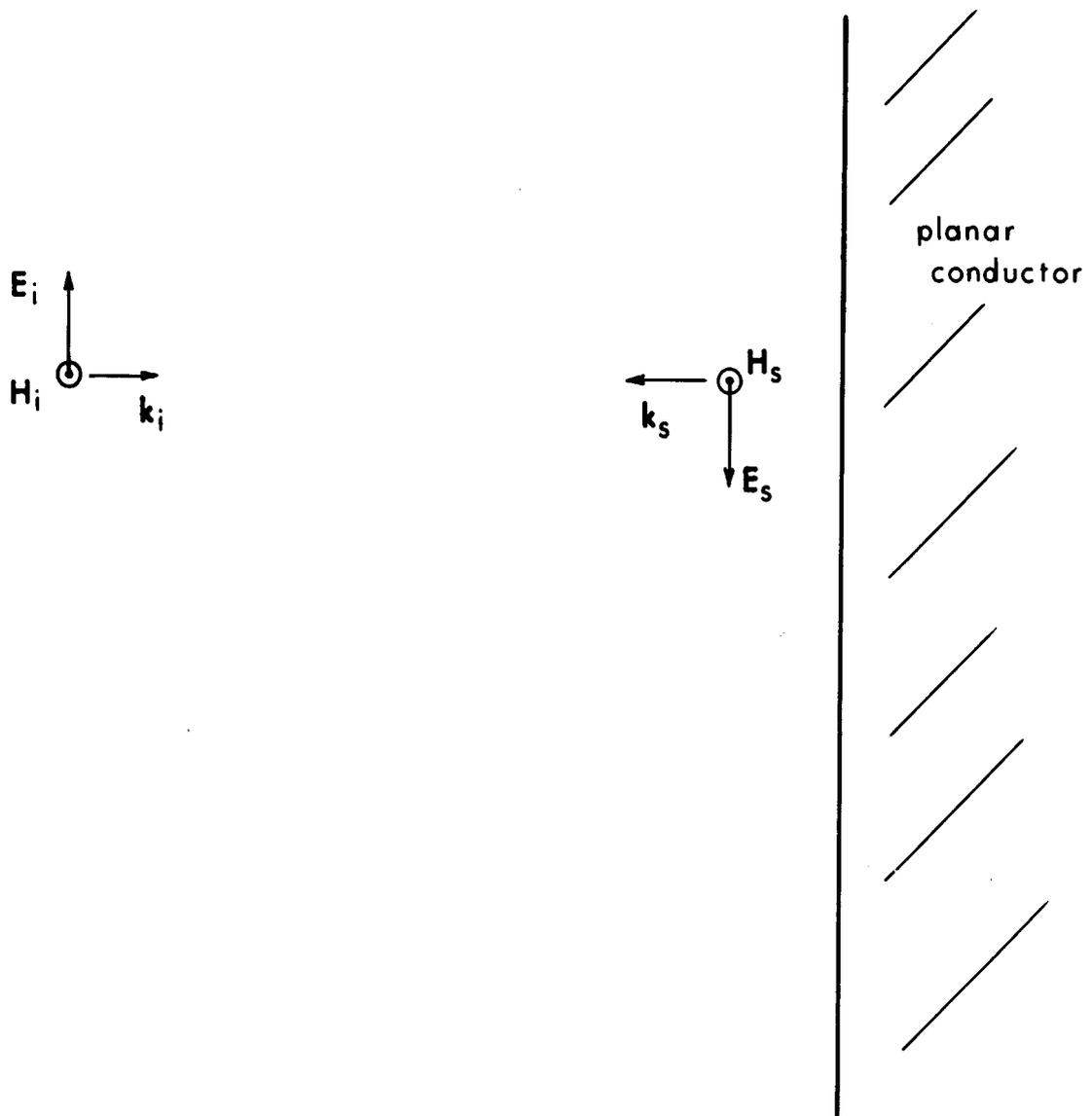
Figure 3.31. Planewave incident on a planar conductor. The conductor produces a scattered wave.
