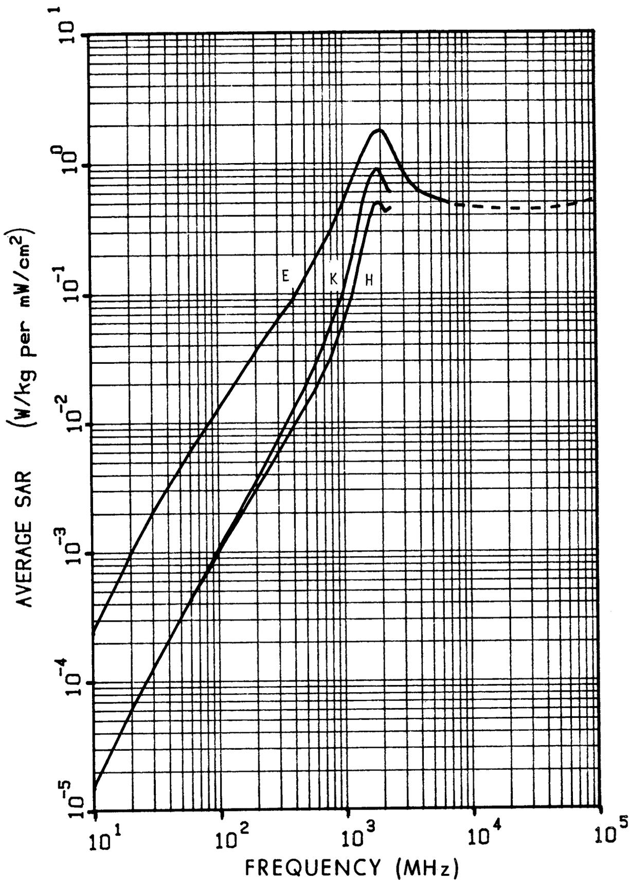
Figure 6.18. Calculated planewave average SAR in a prolate spheroidal model of a medium mouse for three polarizations;  $a = 3.5$  cm,  $b = 1.17$  cm,  $V = 20$  cm<sup>3</sup>. The dashed line is estimated values.
