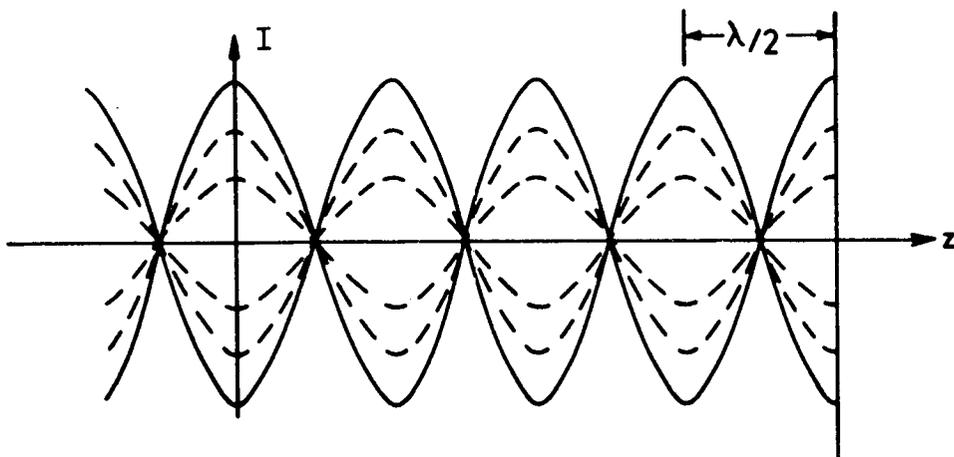
(c) Total current as a function of position at various times through a full cycle, and the envelope of the standing wave.
