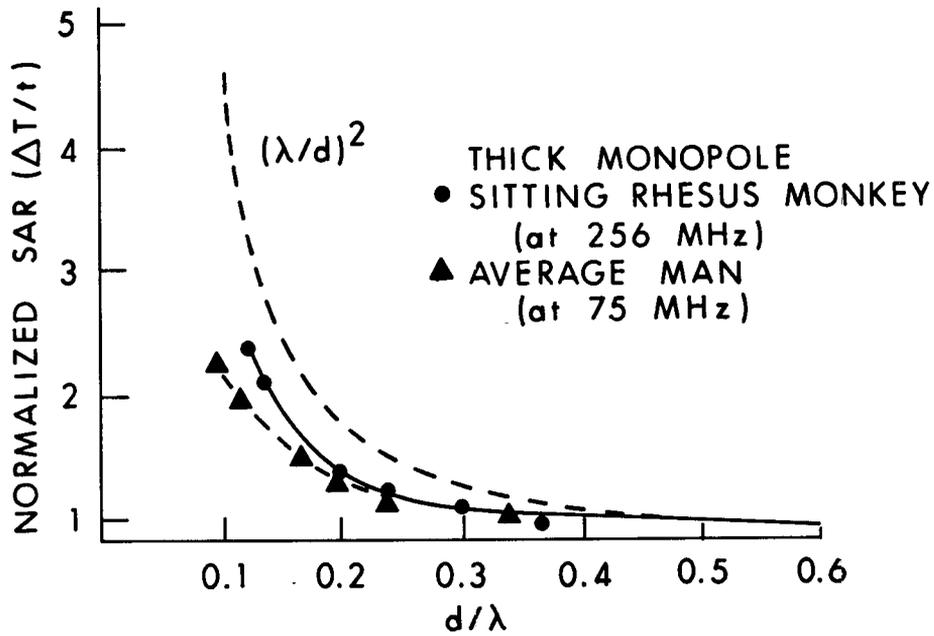
Figure 8.20. Measured relative SARs in scaled saline spheroidal models versus distance. SAR values for the different models are normalized with respect to their planewave value.  $\Delta T$  is the temperature rise in the saline solution after exposure for time  $t$  (Iskander et al., 1981).
