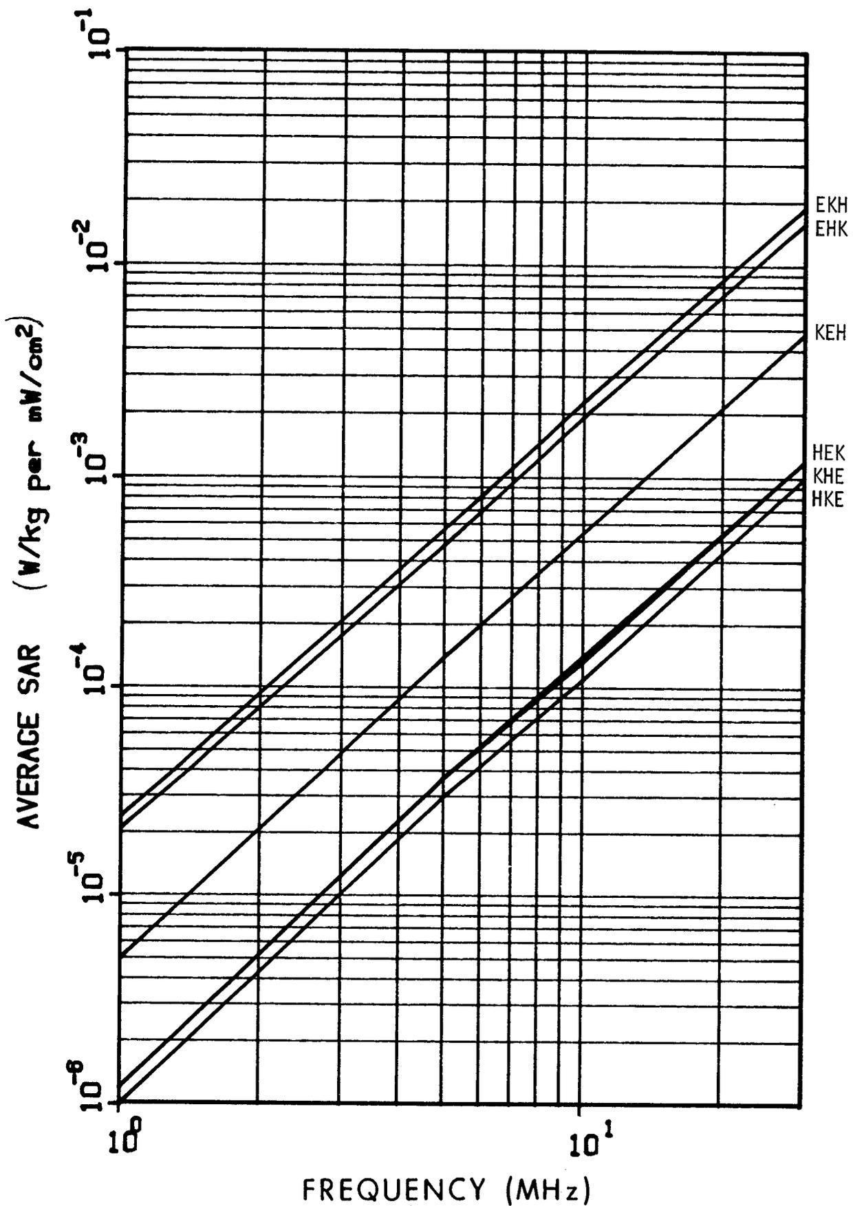
Figure 6.1. Calculated planewave average SAR in an ellipsoidal model of an average man, for the six standard polarizations;  $a = 0.875$  m,  $b = 0.195$  m,  $c = 0.098$  m,  $V = 0.07$  m<sup>3</sup>.
