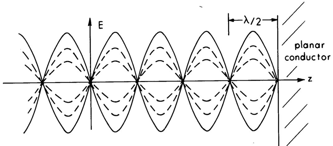
(b) Total  $\mathbf{E}$ -field as a function of position at various times through a full cycle, and the envelope of the standing wave.
