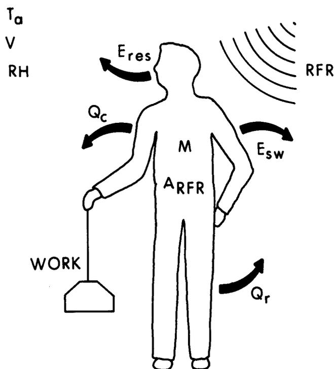
Figure 10.1. A schematic diagram of the sources of body heat (including radiofrequency radiation) and the important energy flows between man and the environment. The body is in thermal equilibrium if the rate of heat loss equals the rate of heat gain. Figure modified from Berglund (1983).
