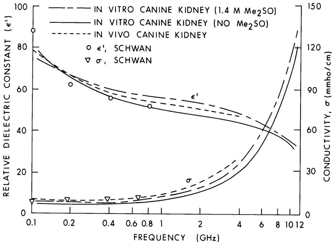
Figure 4.16. Measured values of relative dielectric constant and conductivity of in vivo and in vitro canine kidney cortex (Burdette et al., 1980) compared to reference data (Schwan, 1957).
