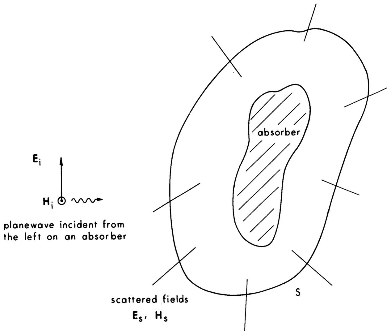
Figure 3.28. A planewave irradiating an absorber.  $S$  is a closed surface used with Poynting's theorem. Scattered fields are produced by the incidence of the planewave on the absorber.
