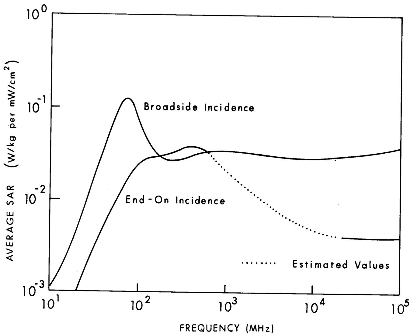
Figure 6.25. Calculated planewave average SAR in a prolate spheroidal model of an average man irradiated by a circularly polarized wave, for two orientations;  $a = 0.875$  m,  $b = 0.138$  m,  $V = 0.07$  m<sup>3</sup>.
