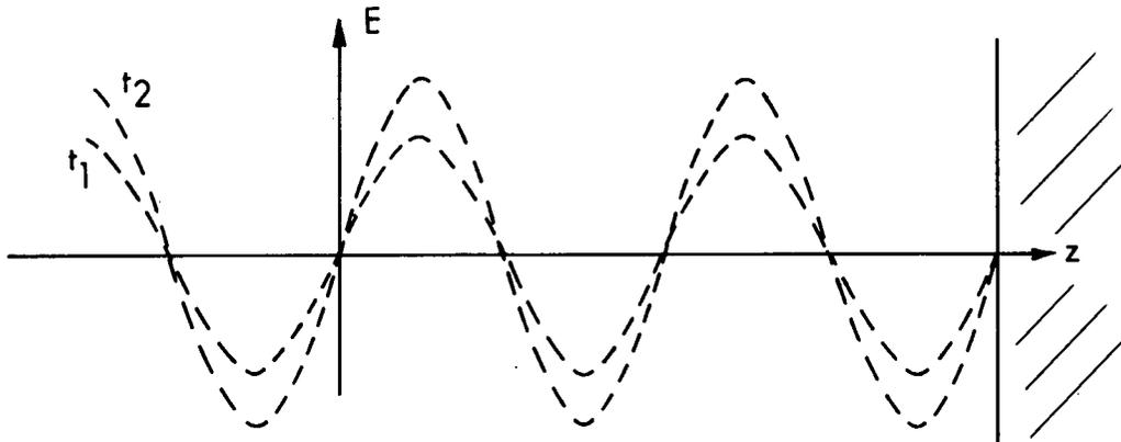
(a) Total  $\mathbf{E}$ -field as a function of position at two times,  $t_1$  and  $t_2$ .
