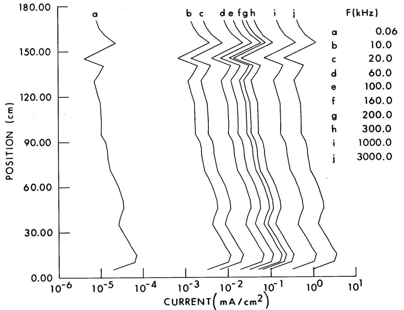
Figure 9.12. Calculated current distribution as a function of position in man exposed to 1-kV/m VLF-MF fields in free space (Guy and Chou, 1982).
