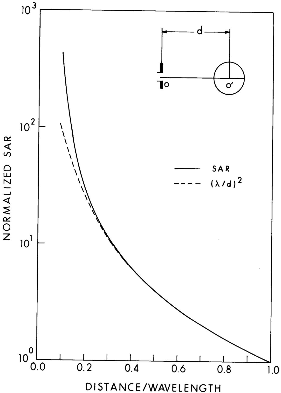
Figure 6.36. Calculated average SAR (by long-wavelength approximation) as a function of the electric dipole location for H polarization at 100 MHz in a prolate spheroidal model of a medium rat.
