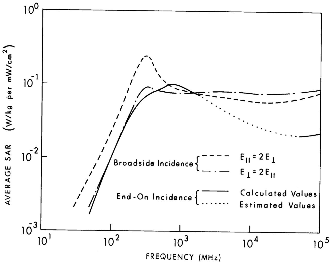
Figure 6.29. Calculated planewave average SAR in a prolate spheroidal model of a sitting rhesus monkey irradiated by an elliptically polarized wave, for two orientations;  $a = 0.2$  m,  $b = 0.0646$  m,  $V = 3.5 \times 10^{-3}$  m<sup>3</sup>.
