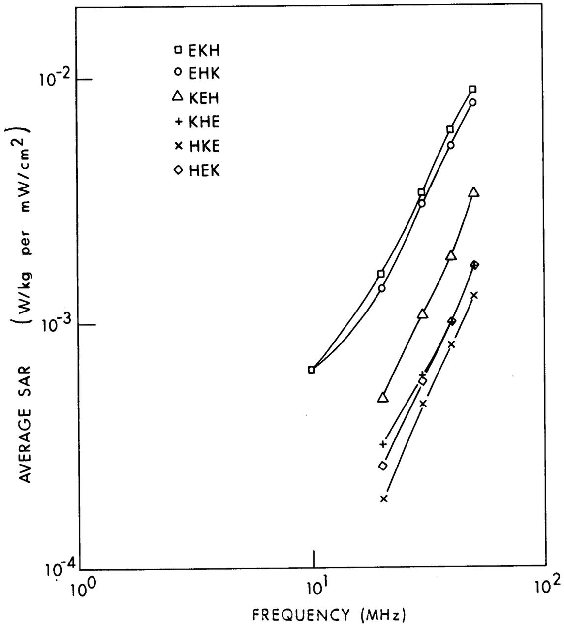
Figure 8.6. Measured values of the average SAR for saline-filled ellipsoidal phantoms, for six standard polarizations;  $a = 20$  cm,  $b = 7.92$  cm,  $c = 5.28$  cm,  $\sigma = 0.54$  S/m (Allen et al., 1976).
