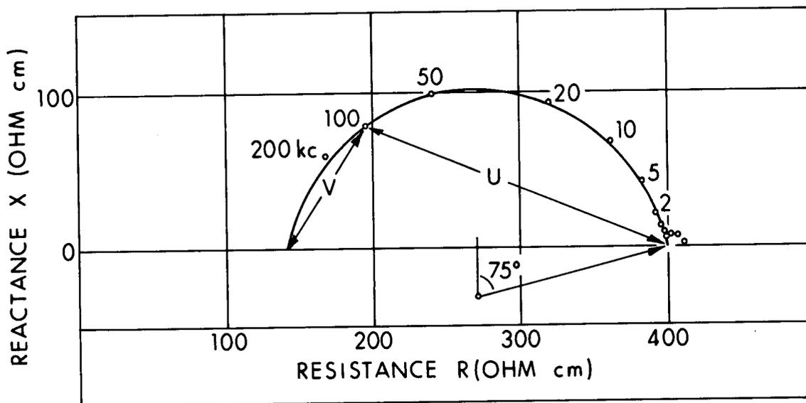
Figure 4.2. Dielectric properties of muscle in the impedance plane, with reactance  $X$  plotted against resistance  $R$  and the impedance  $Z = R + jX$  (Schwan, 1957). The large circle results from the  $\beta$ -dispersion and the small one from the  $\alpha$ -dispersion. The plot does not include the  $\gamma$ -dispersion.
