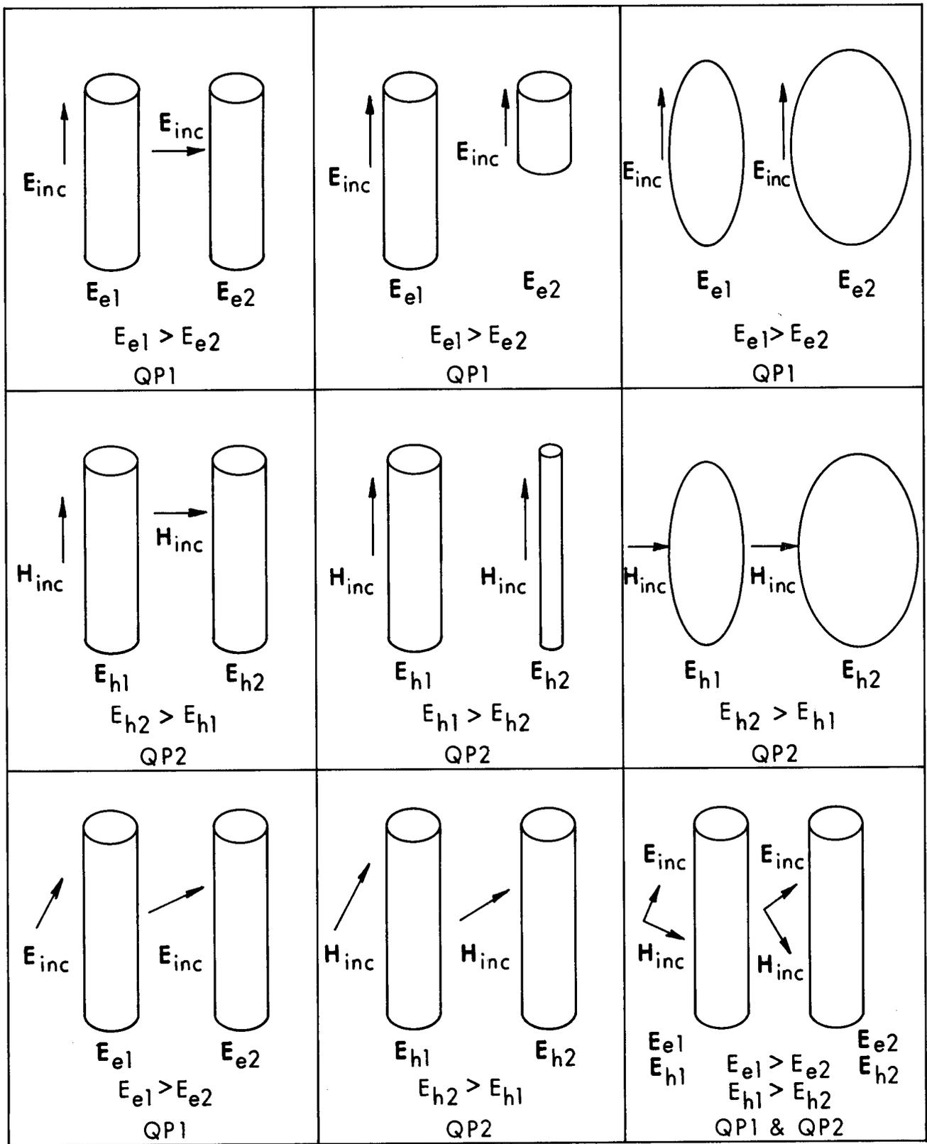
Figure 5.12. Qualitative evaluation of the internal fields based on qualitative principles QP1 and QP2.  $E$  is the internal E-field generated by  $E_{inc}$ , the incident E-field, and  $H_h$  is the internal H-field generated by  $H_{inc}$ , the incident H-field.
