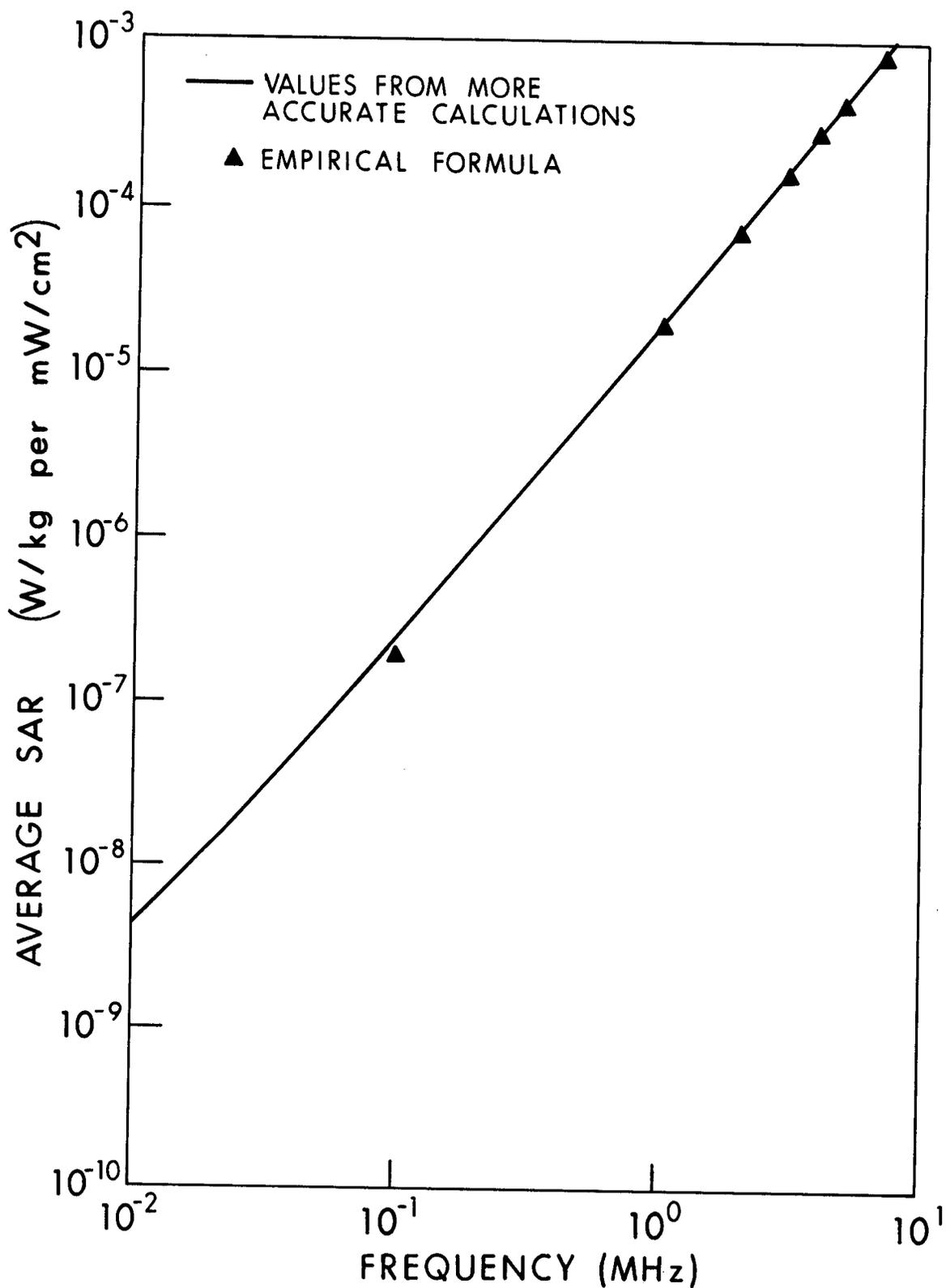
Figure 5.2. Average SAR calculated by the empirical formula compared with the curve obtained by other calculations for a 70-kg man in E polarization. For the prolate spheroidal model,  $a = 0.875$  m and  $b = 0.138$  m; for the cylindrical model, the radius of the cylinder is 0.1128 m and the length is 1.75 m.
