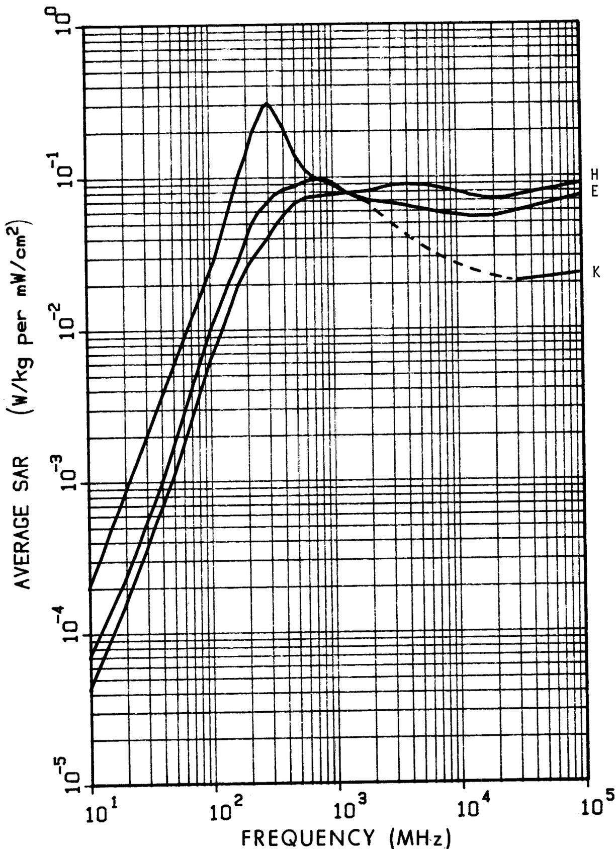
Figure 6.10. Calculated planewave average SAR in a prolate spheroidal model of a sitting rhesus monkey for three polarizations;  $a = 0.2$  m,  $b = 0.0646$  m,  $V = 3.5 \times 10^{-3}$  m<sup>3</sup>. The dashed line is estimated values.
