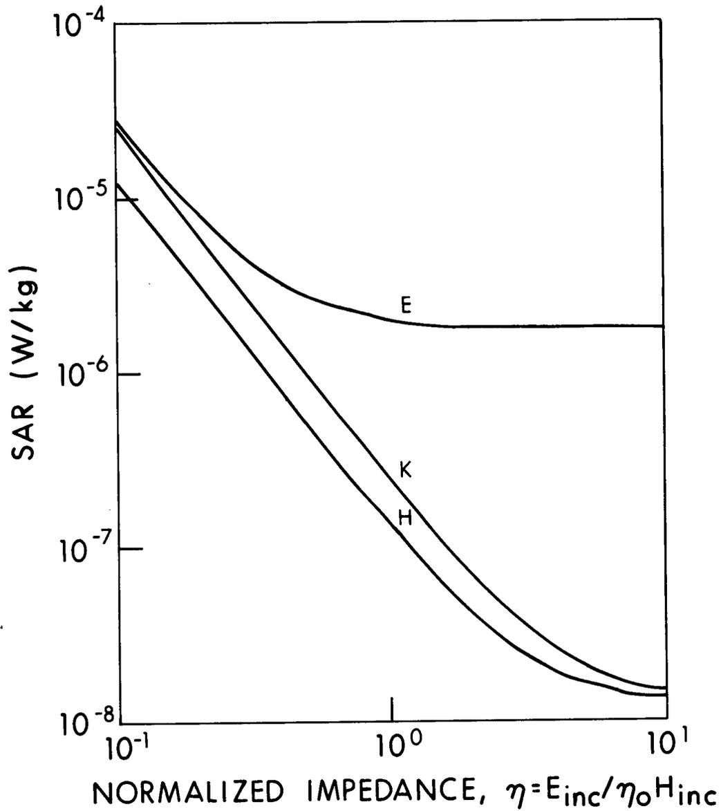
Figure 5.13. Average SAR in a prolate spheroidal model of an average man as a function of normalized impedance for each of the three polarizations. ( $a = 0.875$  m,  $b = 0.138$  m,  $f = 27.12$  MHz,  $\sigma = 0.4$  S/m, incident  $\mathbf{E}$ -field is 1 V/m.)
