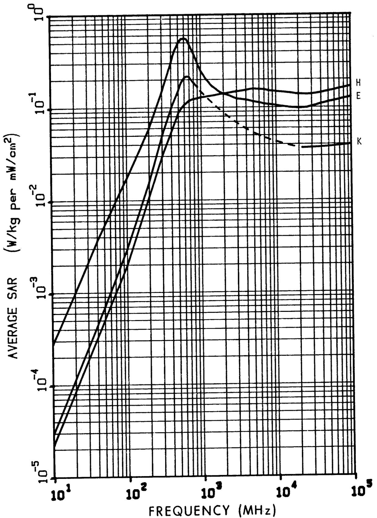
Figure 6.14. Calculated planewave average SAR in a prolate spheroidal model of a guinea pig for three polarizations;  $a = 0.11$  m,  $b = 0.0355$  m,  $V = 5.8 \times 10^{-4}$  m<sup>3</sup>. The dashed line is estimated values.
