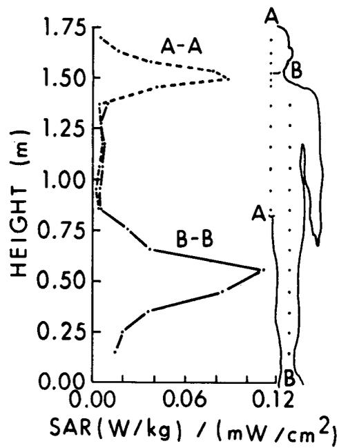
Figure 8.47. SAR distribution along an average man-model height for two cross sections;  $1\text{-mW/cm}^2$  incident-power density on the surface of the model, frequency 350 MHz EIL, K back to front (Krazewski et al., 1984) (© 1984, IEEE).
