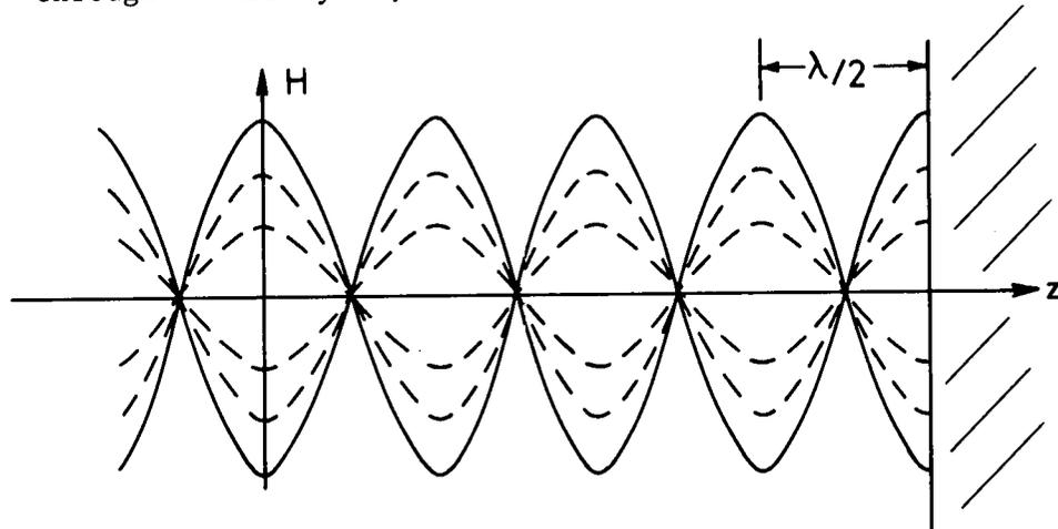
(c) Total  $\mathbf{H}$ -field as a function of position at various times through a full cycle, and the envelope of the standing wave.
