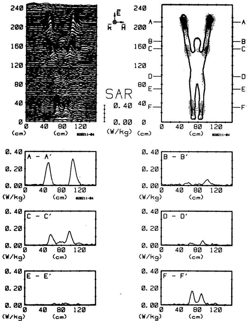
Figure 8.40. Computer-processed whole-body thermograms expressing SAR patterns for man with arms up, exposed to 1-mW/cm<sup>2</sup> 450-MHz radiation with EHK polarization (Guy et al., 1984) (© 1984 IEEE).
