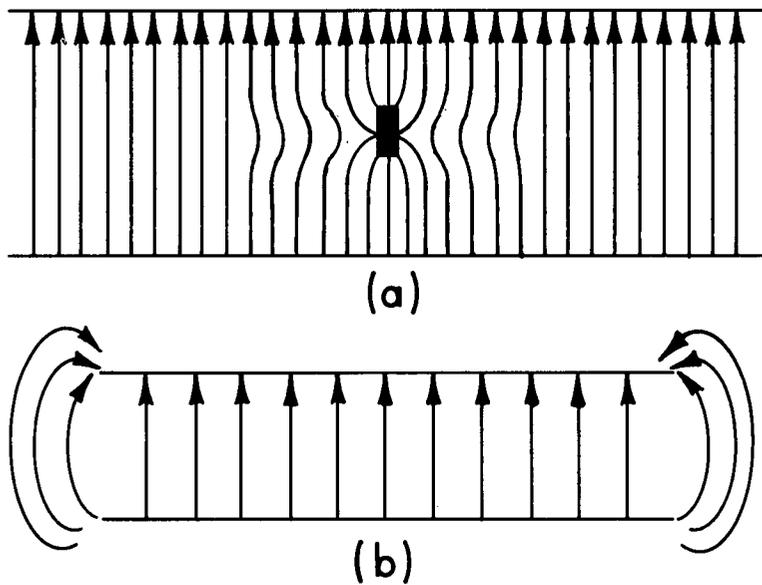
Figure 3.10. (a) **E**-field lines when a small metallic object is placed between the plates.
