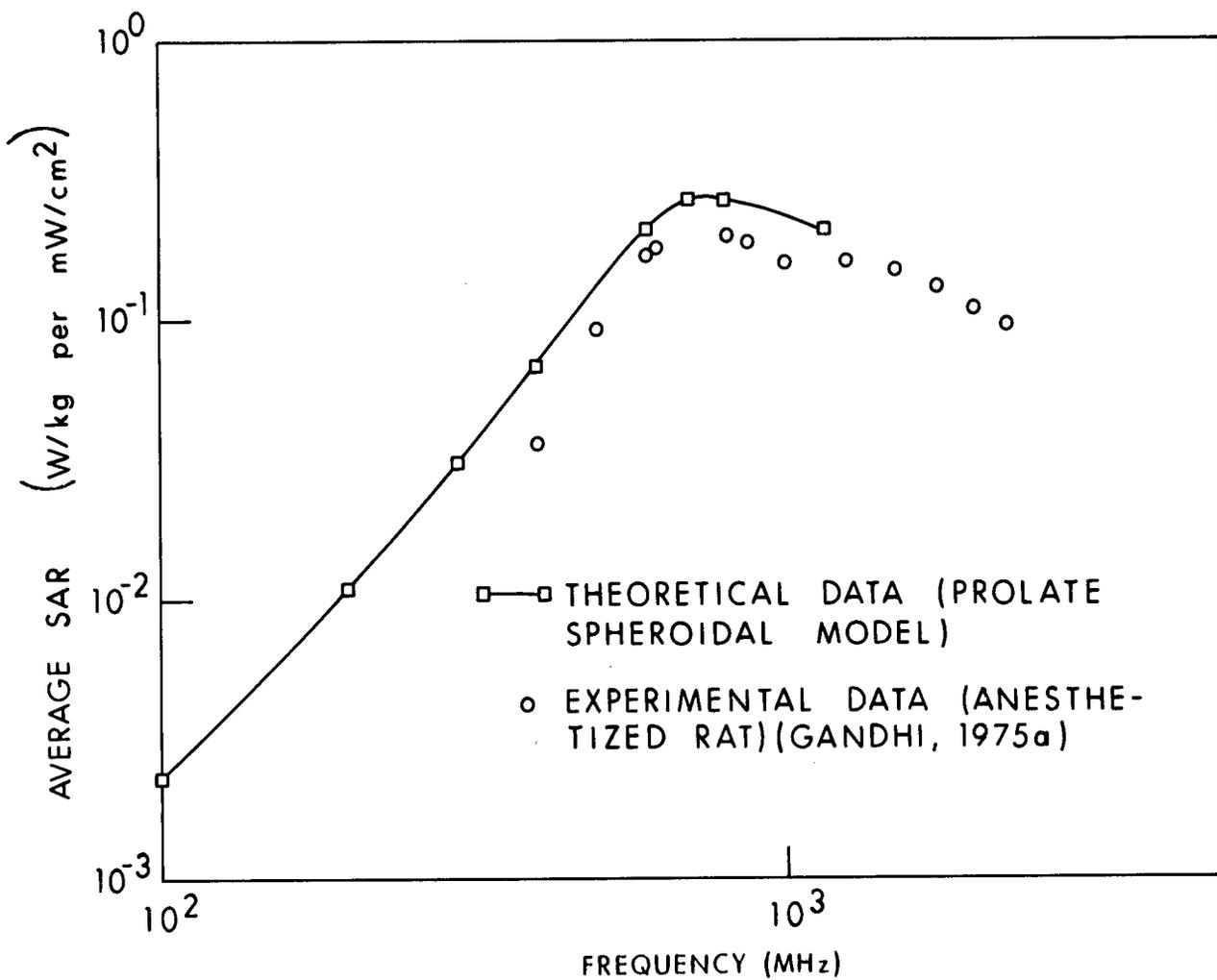
Figure 8.12. Calculated and measured values of the average SAR for a 390-g rat, K polarization.
