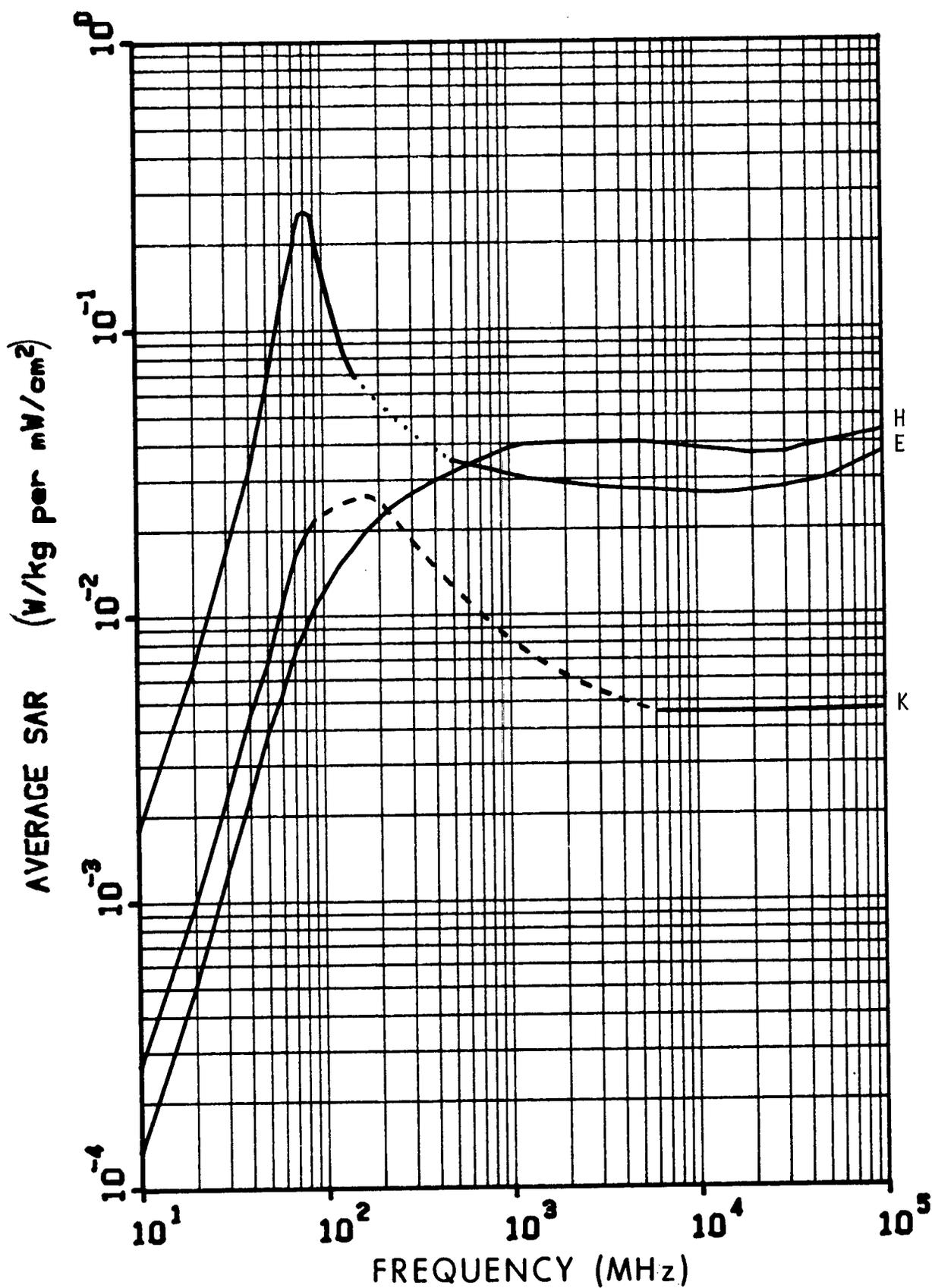
Figure 6.6. Calculated planewave average SAR in a prolate spheroidal model of an average woman for three polarizations;  $a = 0.805$  m,  $b = 0.135$  m,  $V = 0.06114$  m<sup>3</sup>. The dotted line is calculated from Equation 5.1; the dashed line is estimated values.
