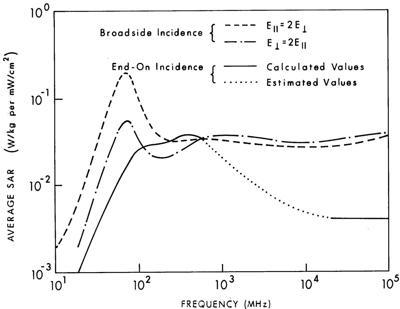
Figure 6.28. Calculated planewave average SAR in a prolate spheroidal model of an average man irradiated by an elliptically polarized wave, for two orientations;  $a = 0.875$  m,  $b = 0.138$  m,  $V = 0.07$  m<sup>3</sup>.
