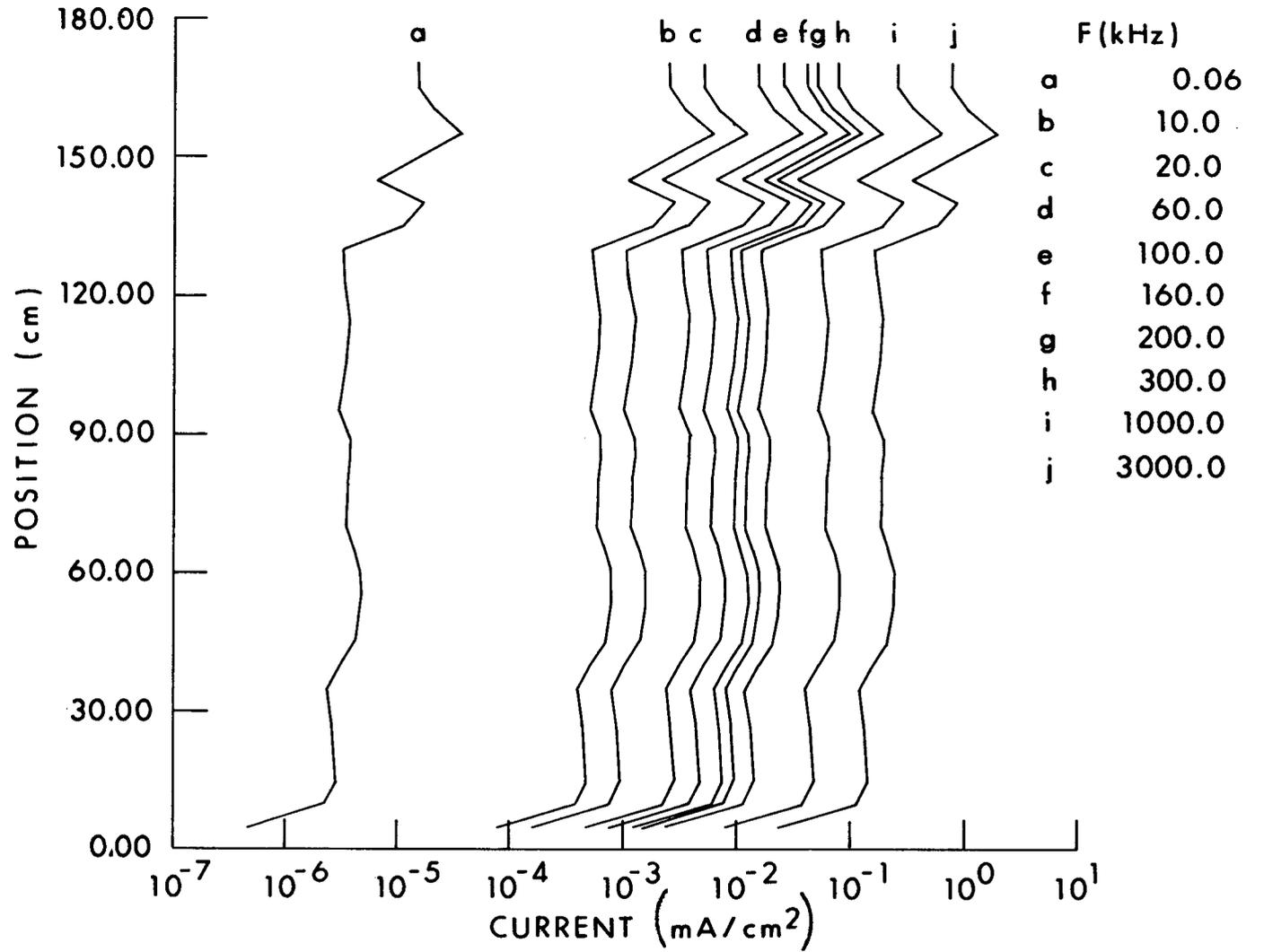
Figure 9.14. Calculated current distributions as a function of position in man exposed to 1-kV/m VLF-MF fields with feet insulated but hands grounded (Guy and Chou, 1982).
