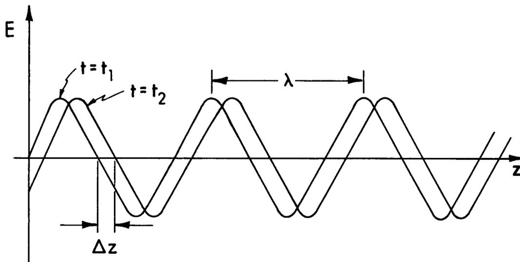
Figure 3.16. Snapshots of a traveling wave at two instants of time,  $t_1$  and  $t_2$ .
