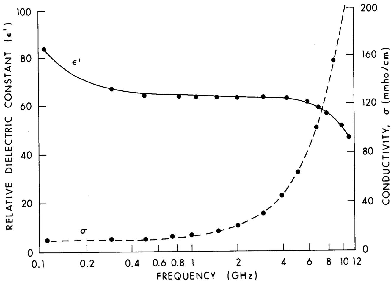
Figure 4.19. Measured values of relative dielectric constant and conductivity of rat blood at 23°C (Burdette et al., 1980).
