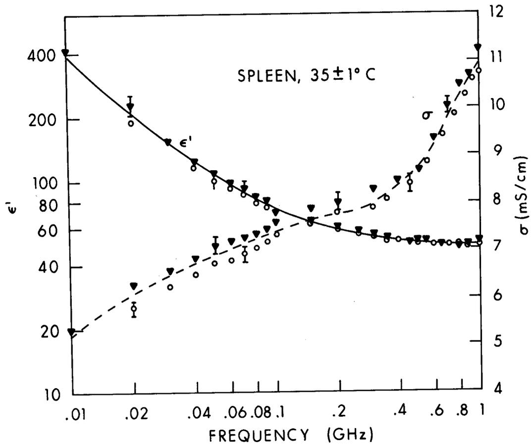
Figure 4.21. Relative permittivity of cat spleen in vivo:  $\blacktriangledown$  and  $\circ$  show results obtained for two locations; the vertical bars show the uncertainty due to estimated measurement errors (SD) (Stuchly et al., 1981).
