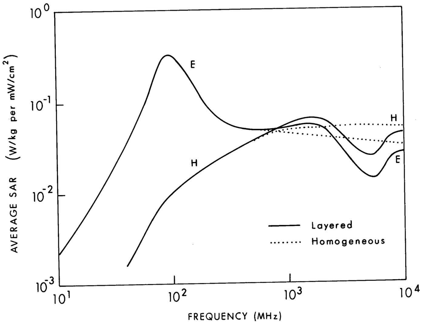
Figure 6.22. Calculated planewave average SAR in homogeneous and multi-layered models of a 10-year-old child for two polarizations.
