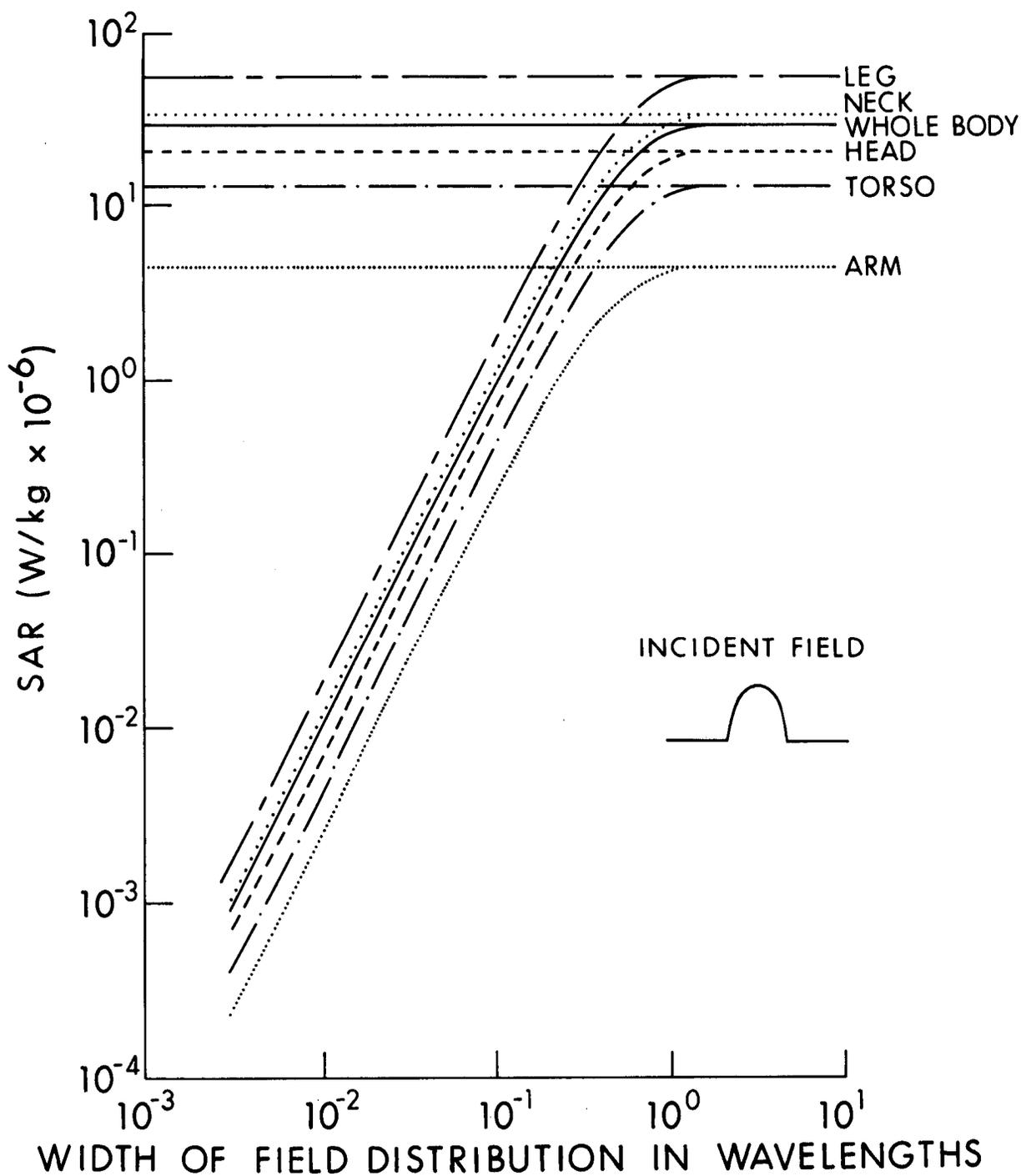
Figure 6.46. Average whole- and part-body SAR in the block model of man placed in front of a half-cycle cosine field,  $E_z$ ; frequency = 77 MHz,  $E_z|_{\max} = 1$  V/m. Calculated by Chatterjee et al. (1980a, 1980b, 1980c).
