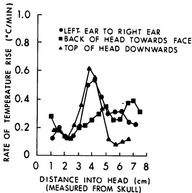
Figure 8.26. Rate of temperature rise from RFR exposure at the right side of a detached *M. mulatta* head; 1.2 GHz, CW, 70 mW/cm<sup>2</sup>, far field (Burr and Krupp, 1980).
