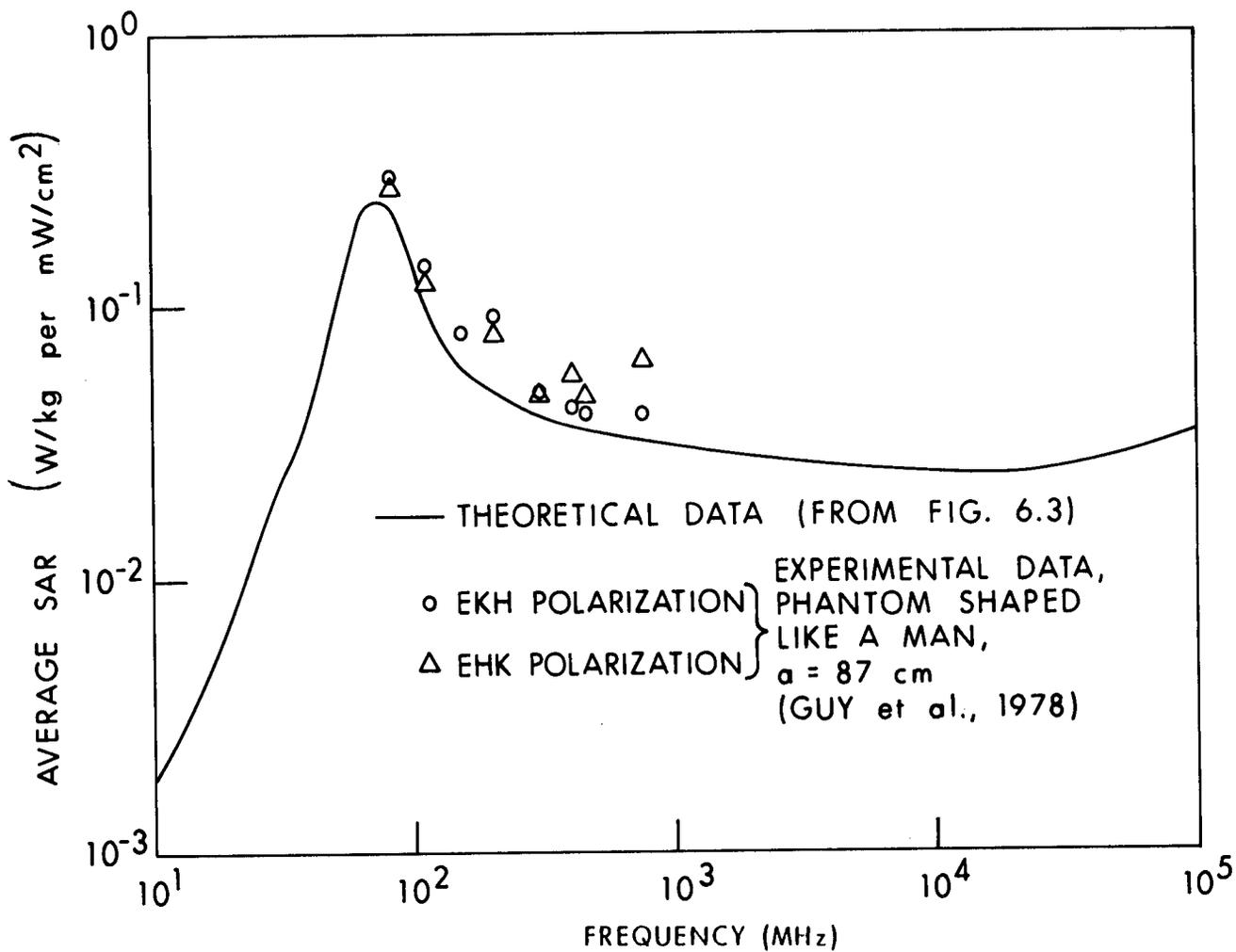
Figure 8.8. Calculated and measured values of the average SAR for models of an average man, E polarization.
