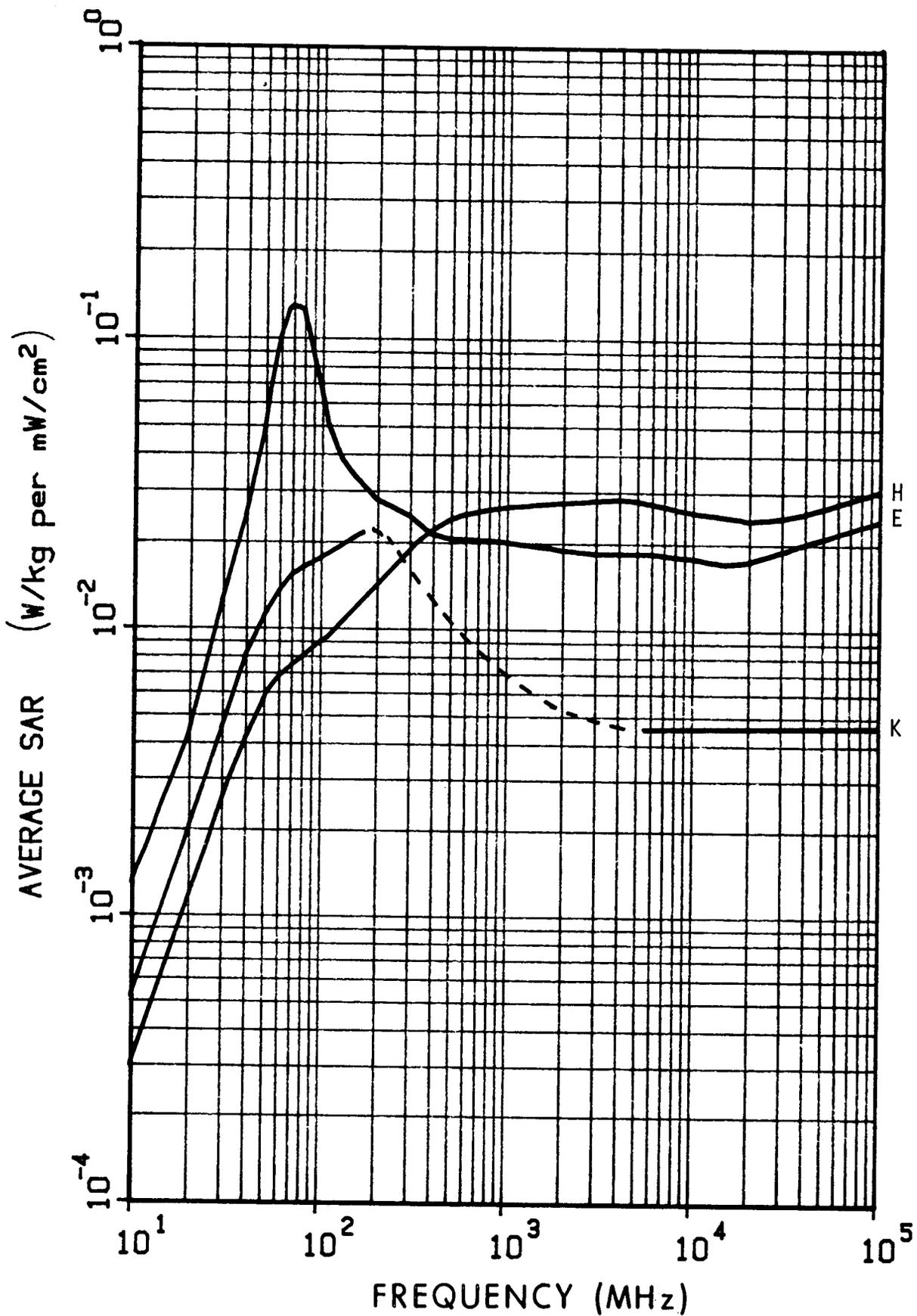
Figure 6.5. Calculated planewave average SAR in a prolate spheroidal model of an average endomorphic (fat) man for three polarizations;  $a = 0.88$  m,  $b = 0.195$  m,  $V = 0.141$  m<sup>3</sup>. The dashed line is estimated values.
