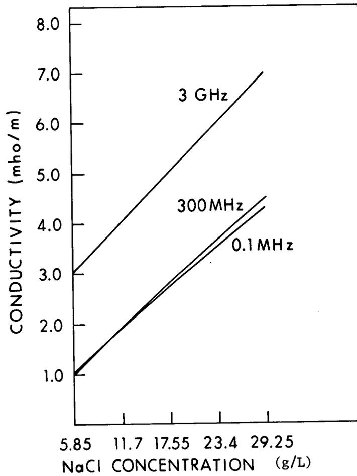
Figure 7.7. Electrical conductivity of saline solution as a function of the NaCl concentration at 25°C.
