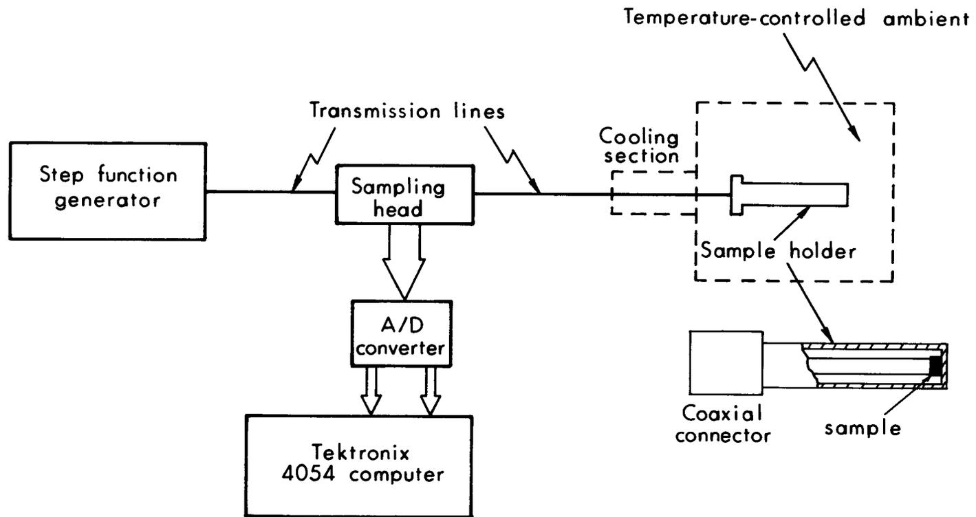
Figure 4.9. Typical experimental setup for time-domain measurement of complex permittivities.
