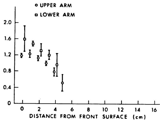
Figure 8.23. Profiles of electromagnetic absorption in the sitting rhesus model at 225 MHz. Vertical bars represent  $\pm 1$  SD (N = 3) in calculated mean SAR (Olsen and Griner, 1982).
