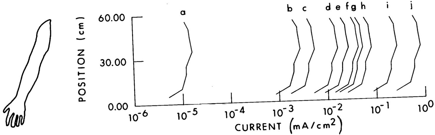
Figure 9.13. Calculated current density flowing through one arm. The exposure condition is the same as for Figure 9.12 (Guy and Chou, 1982).
