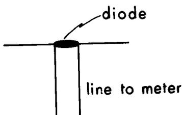
Figure 3.42. Simple electric-field probe with a diode detector.
