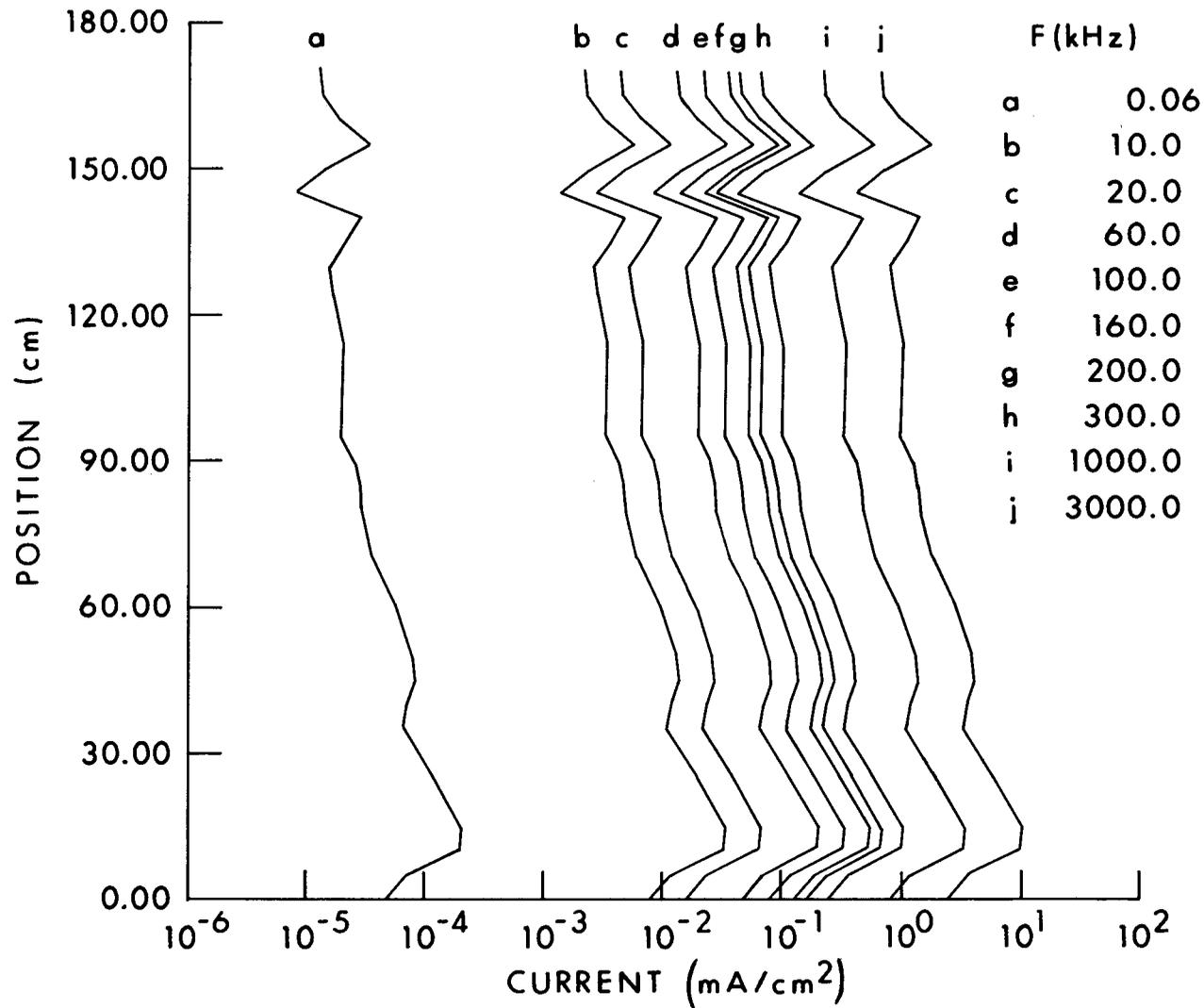
Figure 9.10. Calculated current distributions as a function of position in man exposed to 1-kV/m VLF-MF fields with feet grounded (Guy and Chou, 1982).
