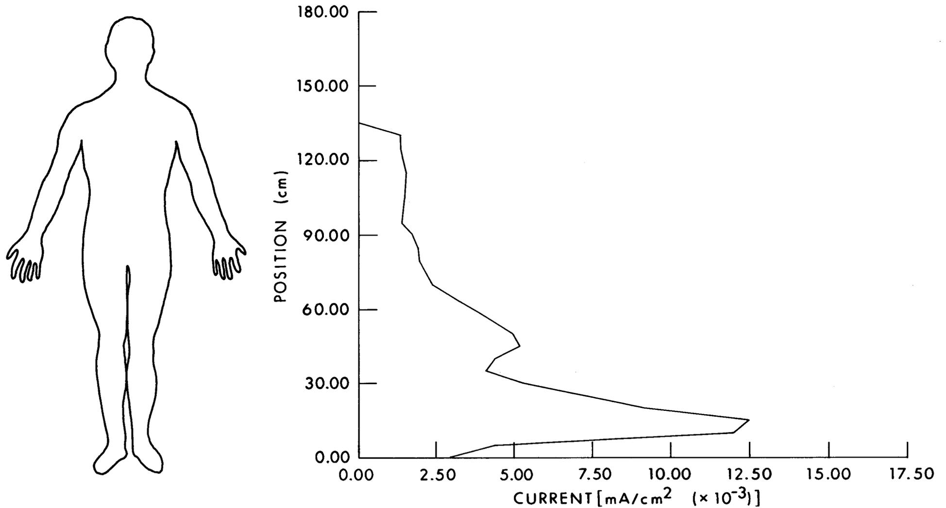
Figure 9.16. Calculated current distribution as a function of position in man with hand contacting a large object and with feet grounded. A 1-mA current is assumed to be flowing through the arm, thorax, and legs of the subject to ground,  $F = 60$  Hz (Guy and Chou, 1982).
