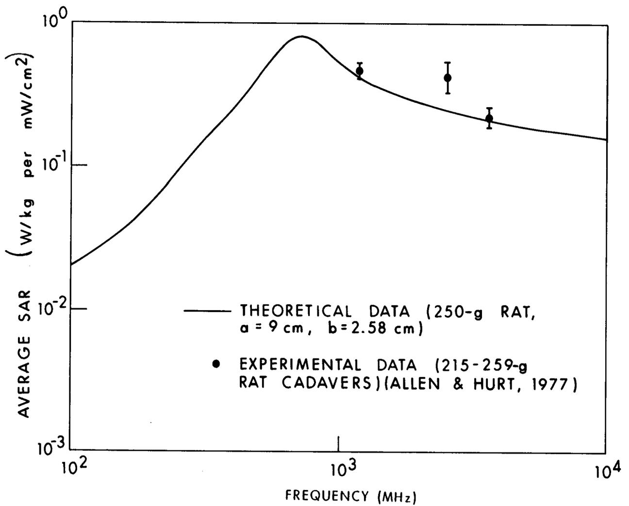
Figure 8.15. Calculated and measured values of the average SAR for models of a rat, E polarization.
