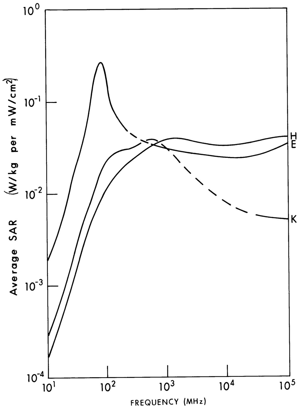
Figure 3.39. Calculated whole-body average SAR versus frequency for models of an average man for three standard polarizations. The incident-power density is 1 mW/cm<sup>2</sup>.
