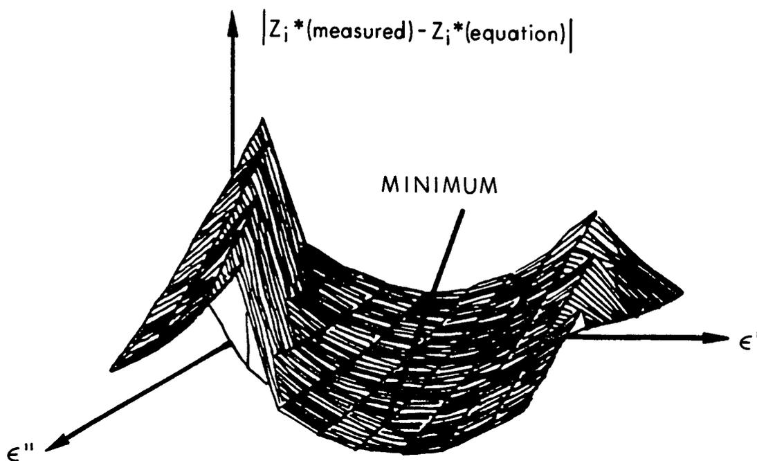
Figure 4.11. Graphical illustration of the iterative procedure for calculating complex permittivity parameters by minimizing the difference between measured and calculated values of the input impedance of the in vivo dielectric probe. The minimum on the error surface  $|Z_{\text{measured}} - Z_{\text{calculated}}|$  indicates the most appropriate values of  $\epsilon'$  and  $\epsilon''$  that satisfy the measured value of the input impedance.
