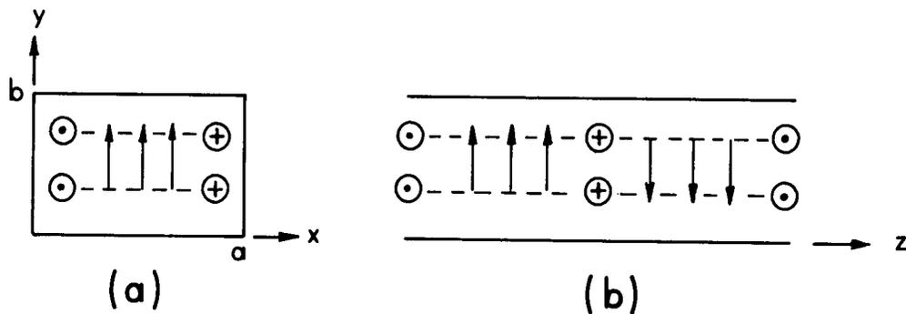
Figure 3.25. Field variation of the  $TE_{10}$  mode in a rectangular waveguide (a) as would be seen looking down the waveguide and (b) as seen looking at the side of the waveguide. The solid lines are electric field and the dotted lines are magnetic field.
