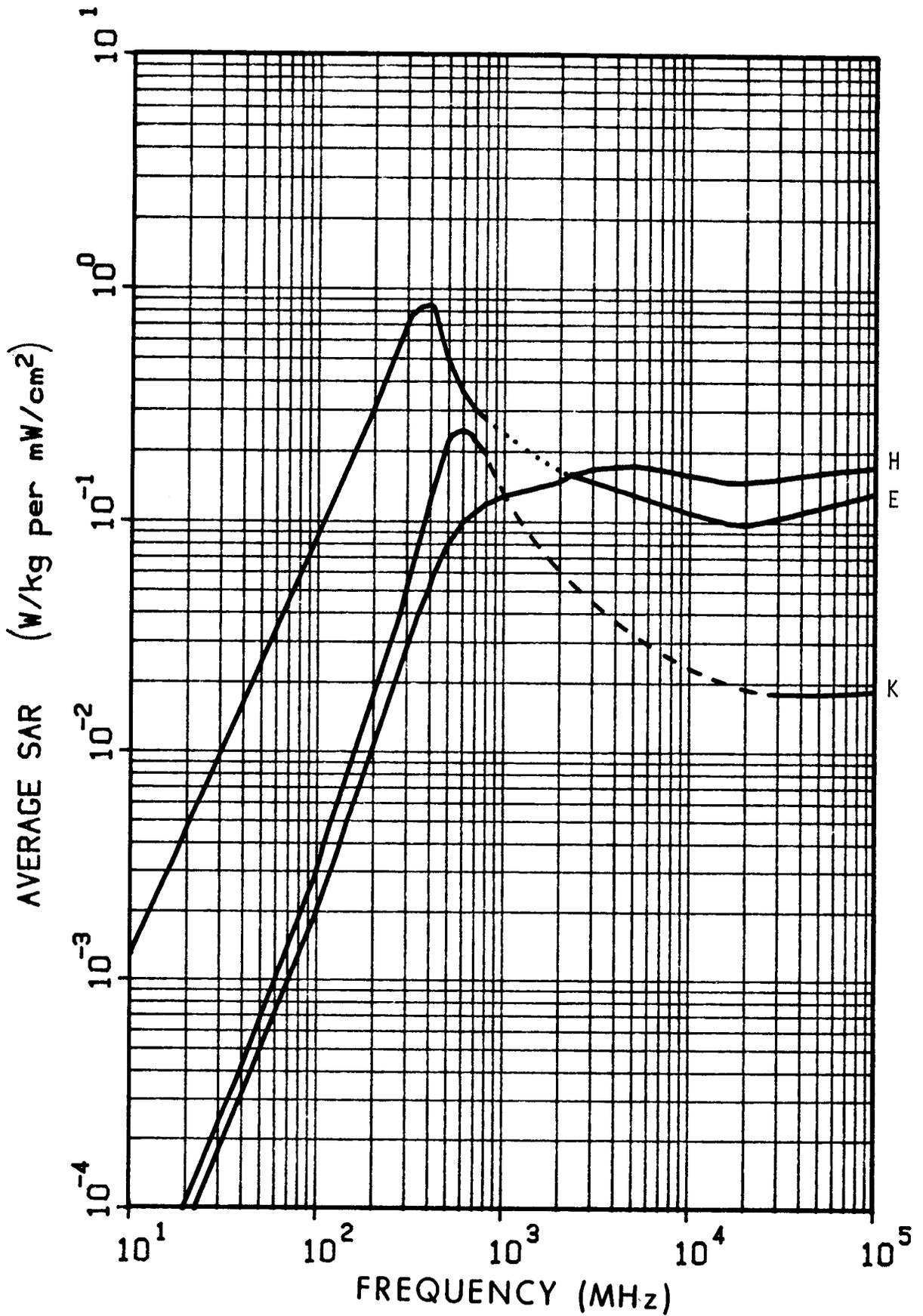
Figure 6.13. Calculated planewave average SAR in a prolate spheroidal model of a rabbit, for three polarizations;  $a = 0.2$  m,  $b = 0.0345$  m,  $V = 1 \times 10^{-3}$  m<sup>3</sup>. The dotted line is calculated from Equation 5.1; the dashed line is estimated values.
