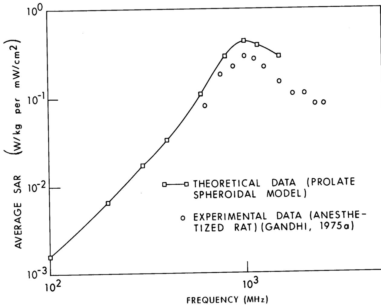
Figure 8.10. Calculated and measured values of the average SAR for a 158-g rat, K polarization.
