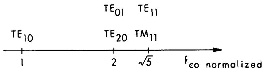
Figure 3.26. Some relative cutoff frequencies for a waveguide with  $b = a/2$ , normalized to that of the  $TE_{10}$  mode.
