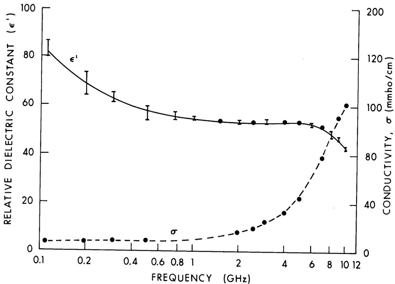
Figure 4.18. Measured values of relative dielectric constant and conductivity of in vivo rat brain at 32°C. Maximum SEM for  $\epsilon'$  is indicated by error bars and SEM for  $\epsilon'' = \pm 0.9$  (Burdette et al., 1980).
