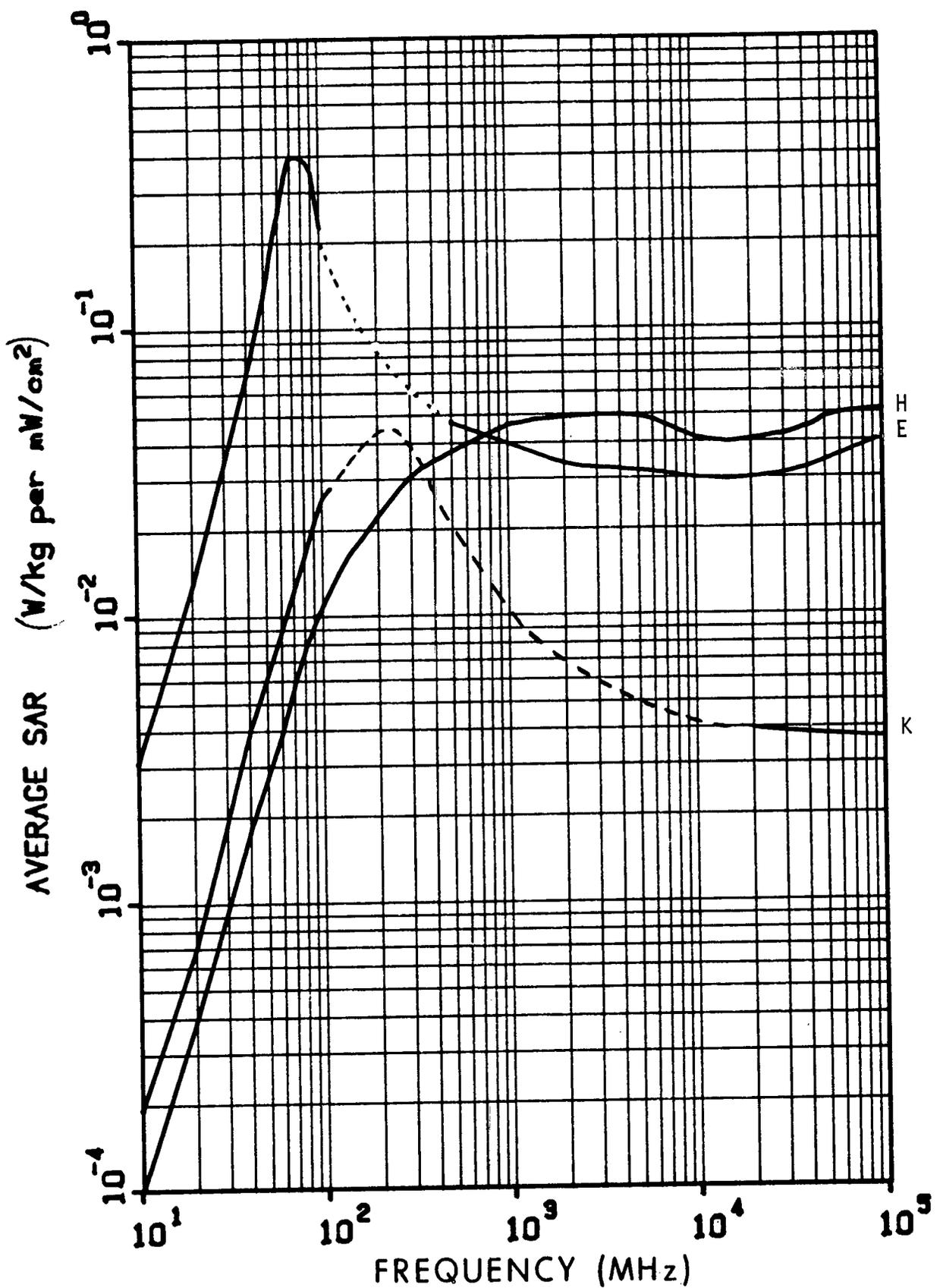
Figure 6.4. Calculated planewave average SAR in a prolate spheroidal model of an average ectomorphic (skinny) man for three polarizations;  $a = 0.88$  m,  $b = 0.113$  m,  $V = 0.04718$  m<sup>3</sup>. The dotted line is calculated from Equation 5.1; the dashed line is estimated values.
