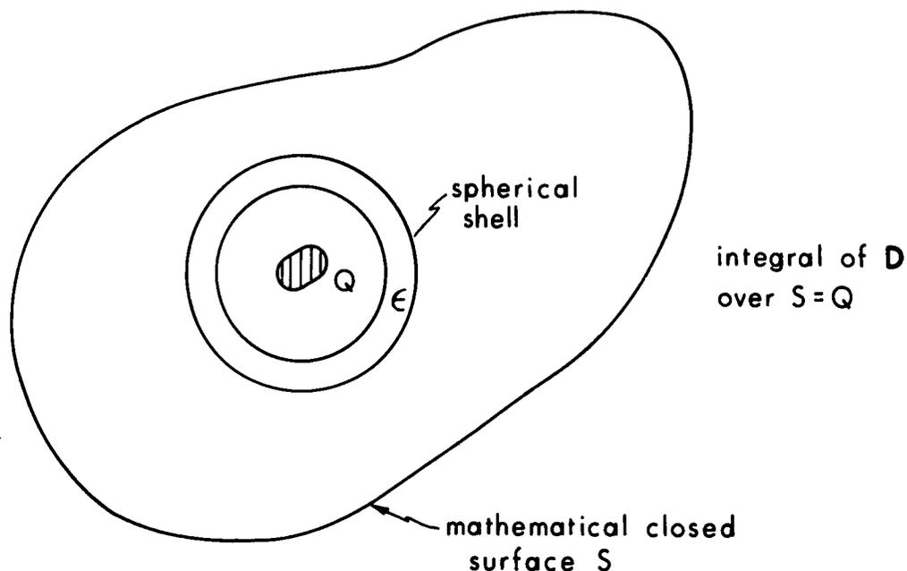
Figure 3.15. Charge  $Q$  inside a dielectric spherical shell.  $S$  is a closed mathematical surface.
