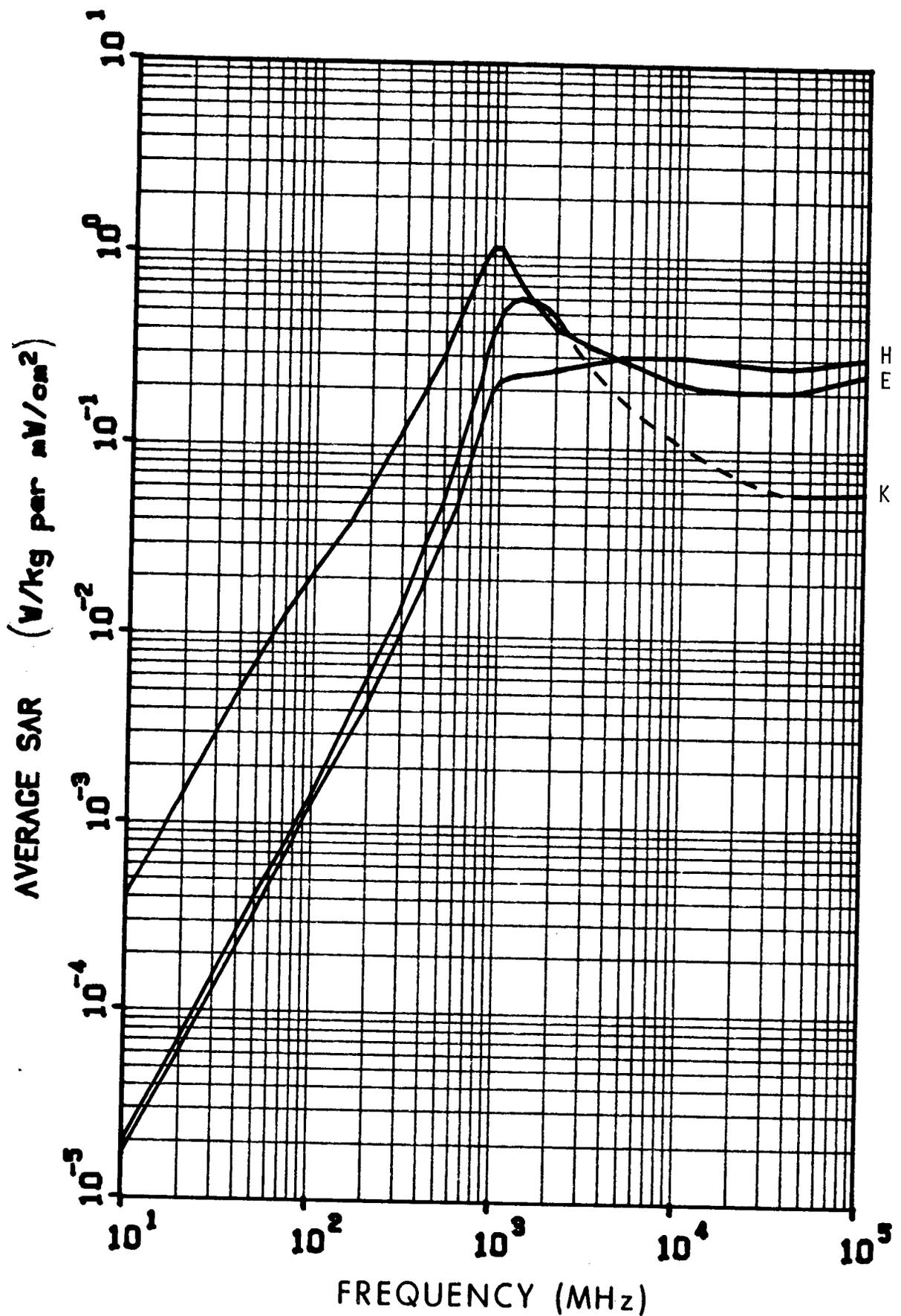
Figure 6.15. Calculated planewave average SAR in a prolate spheroidal model of a small rat for three polarizations;  $a = 0.07$  m,  $b = 0.194$  m,  $V = 1.1 \times 10^{-4}$  m<sup>3</sup>. The dashed line is estimated values.
