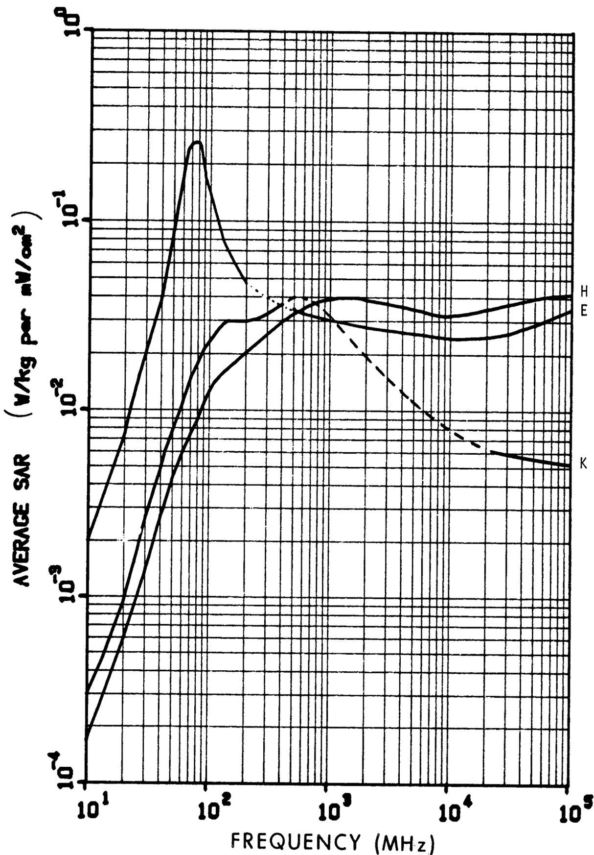
Figure 6.3. Calculated planewave average SAR in a prolate spheroidal model of an average man for three polarizations;  $a = 0.875$  m,  $b = 0.138$  m,  $V = 0.07$  m<sup>3</sup>. The dotted line is calculated from Equation 5.1; the dashed line is estimated values.
