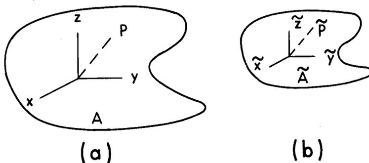
Figure 7.4. Schematic diagram illustrating the coordinate system used in the scaling procedure. (a) Full-size object with coordinate system  $x, y, z$ ; (b) scaled model with coordinate system  $\tilde{x}, \tilde{y}, \tilde{z}$ .
