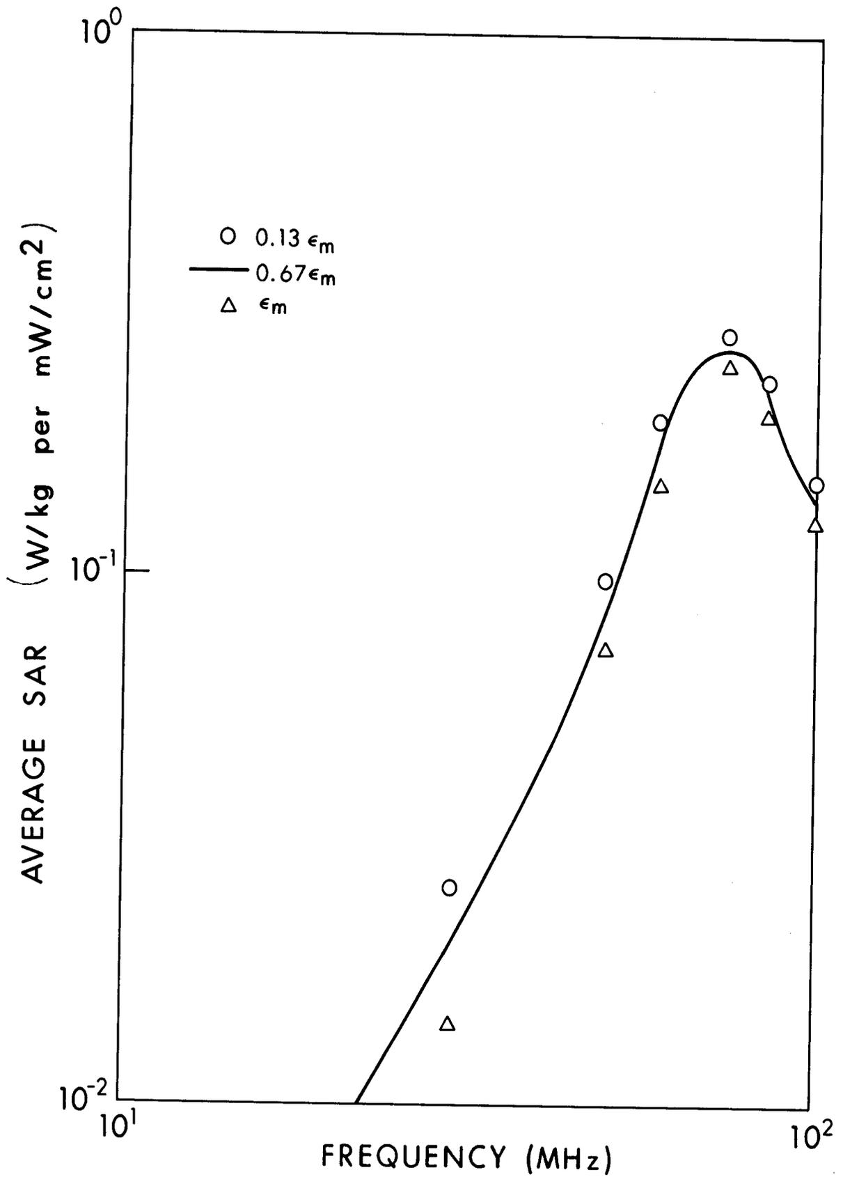
Figure 5.7. Calculated average SAR in a prolate spheroidal model of an average man, as a function of frequency for several values of permittivity.  $\epsilon_m$  is the permittivity of muscle tissue.
