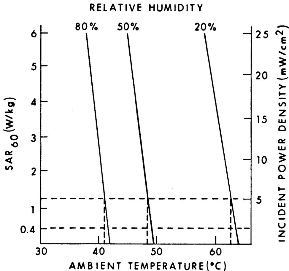
Figure 10.7. Calculated SAR<sub>60</sub> values in an average man, unclothed and quiet, irradiated by an electromagnetic planewave with E polarization at resonance (about 70 MHz). Dashed horizontal lines indicate the psychrometric conditions (in still air) that yield an SAR<sub>60</sub> of 1.25 W/kg and 0.4 W/kg at this frequency.
