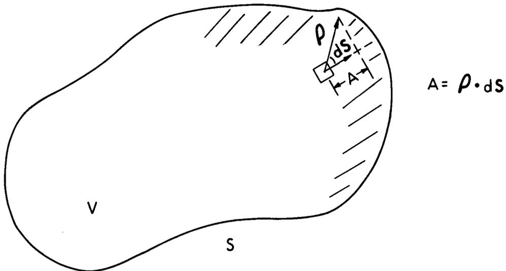
Figure 3.27. A volume ( $V$ ) bounded by a closed surface ( $S$ ).  $d\mathbf{S}$  is the differential surface vector.  $\rho \cdot d\mathbf{S}$  is the projection of  $\rho$  on  $d\mathbf{S}$ , which corresponds to power passing out through  $dS$ .
