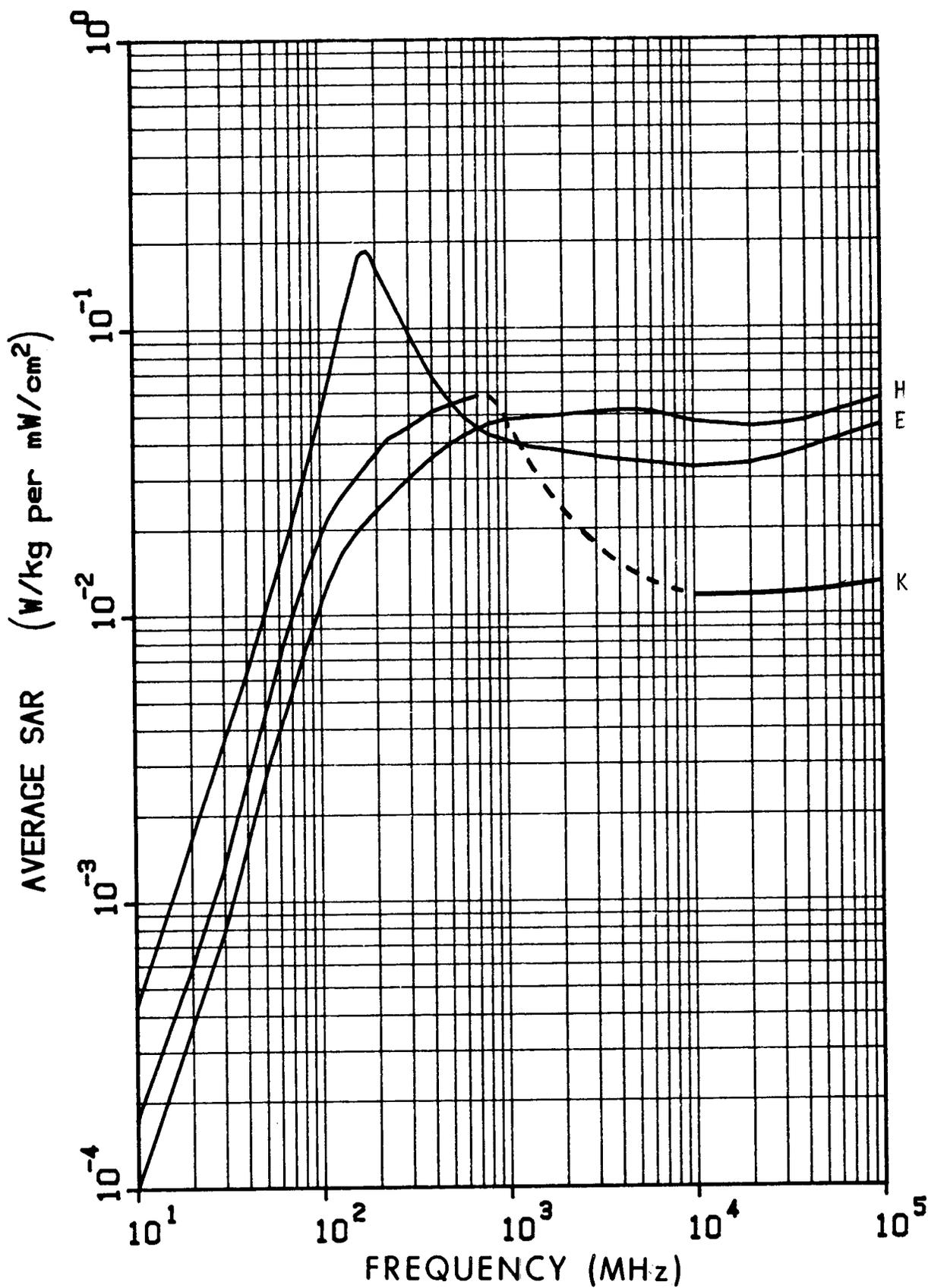
Figure 6.12. Calculated planewave average SAR in a prolate spheroidal model of a Brittany spaniel for three polarizations;  $a = 0.344$  m,  $b = 0.105$  m,  $V = 0.0159$  m<sup>3</sup>. The dashed line is estimated values.
