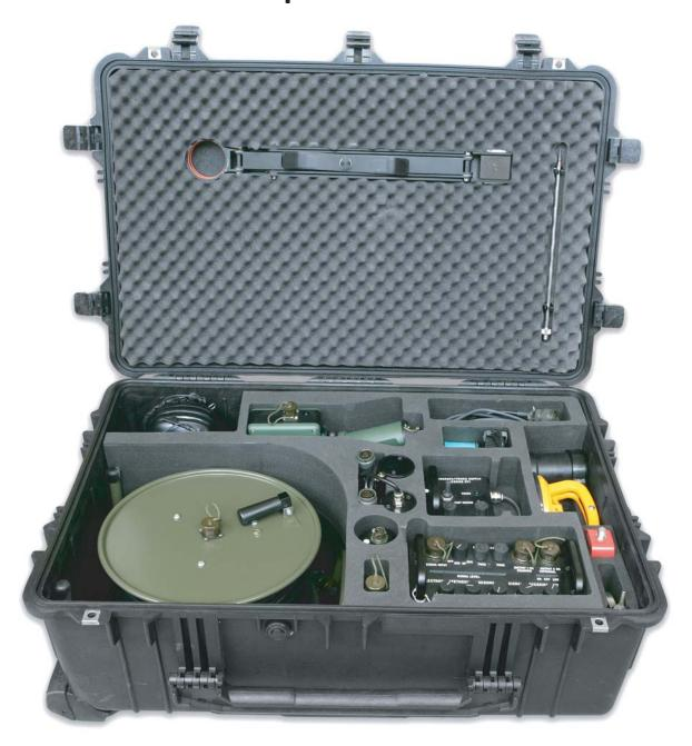
The RE 80 M2 EST is an advanced modular electronic stethoscope designed for both EOD & IEDD applications. The equipment has the capability of amplifying acoustic vibrations which are the basis of sound waves, emanating from mechanical, electro mechanical and certain electronic fuses and timing devices.
