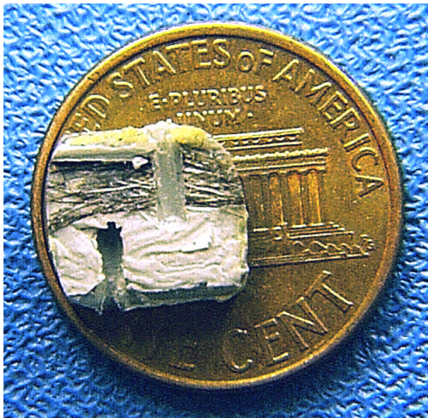
Figure 7. Inside the dielectric component, fibers across upper half of component are human hair.
