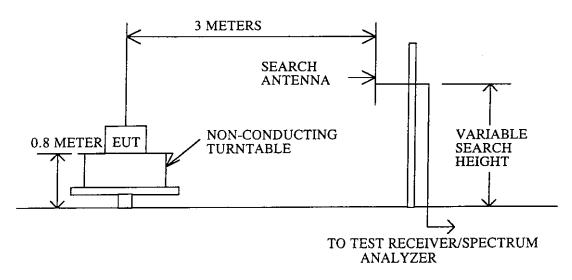
For Super Regenerative Receivers the receiver was activated using a tuned dipole antenna fed with a CW signal. The frequency of the activating signal is adjusted to obtain worst-case field strength of the EUT oscillator emission.
