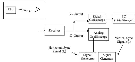
Figure 3 - Reconstruction Test Setup.
