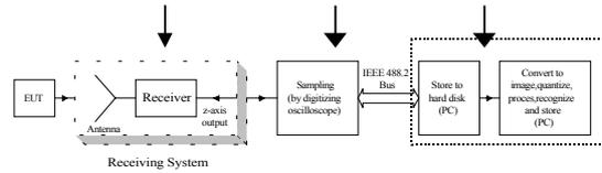
(b) Corresponding Building Blocks in Reconstruction Test Setup.
