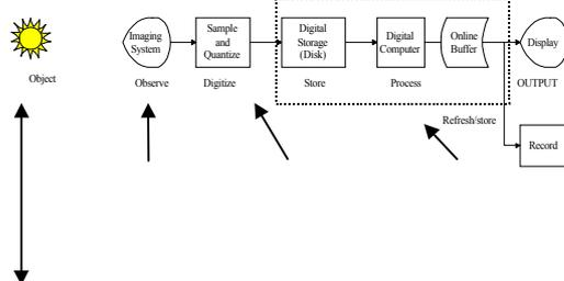
(a) A typical digital image processing system.
