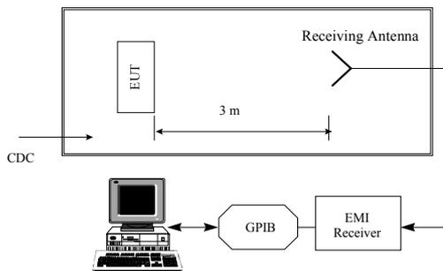
Figure 2 - Frequency Domain Test Set-up
