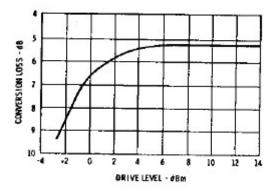
Conversion Loss vs. LO Drive Level: The minimum recommended drive level is +4 dBm. The maximum recommended drive level is +13 dBm.
