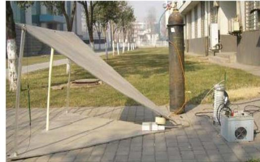
**Figure 7.** Photo of TEM horn antenna.
