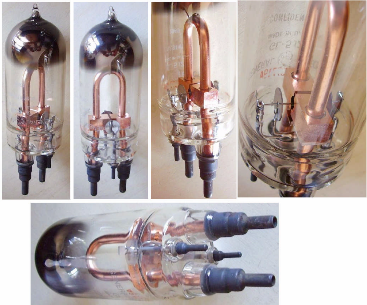
Fig. 6 - 5J29 was the first of three split-anode magnetrons designed by General Electric for high-frequency jammers. The two anode copper blocks are internally connected by a short copper tubing which acts as shorting termination of the external tuning line, also granting inside the circulation of the cooling fluid.
