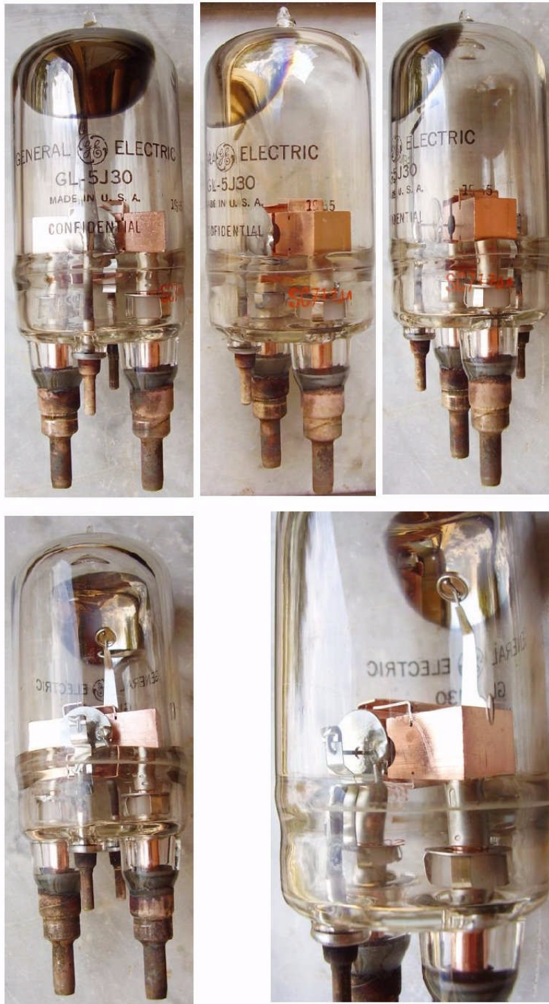
Fig. 7 - General Electric 5J30, split anode magnetron. Each anode block is fluid cooled through coaxial copper tubing. The two blocks are insulated from each other, the resonant line being shorted by a tuning stub on the side opposite to the magnetron. Thoriated tungsten filamentary cathode with shielding rings at each end and small shielding vanes along the filament axis.
