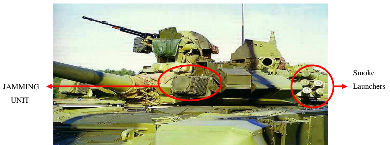
Figure 4 Shtor-1 employs a pair of electro-optical jammer
