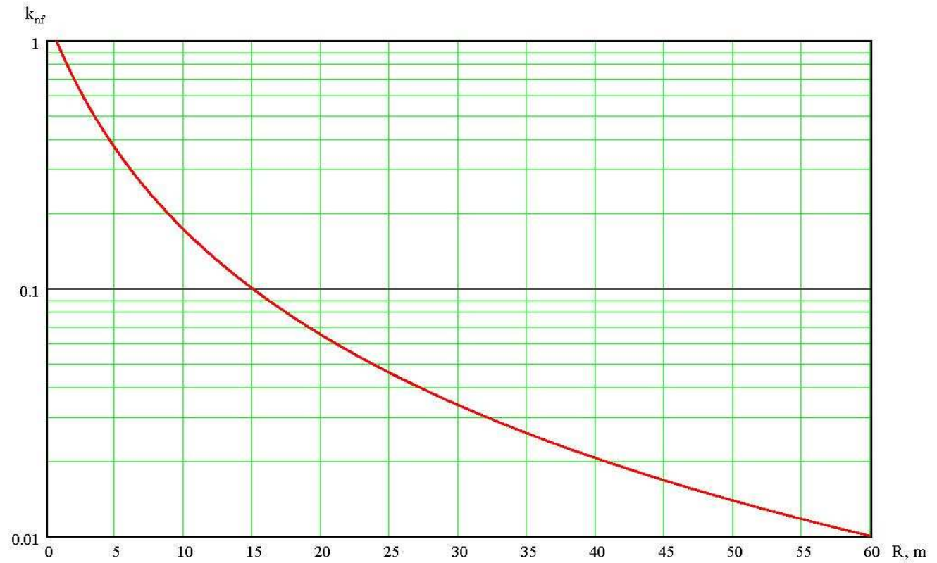
Figure 22 Calibration curve where transmission of attenuator filters vs. range
