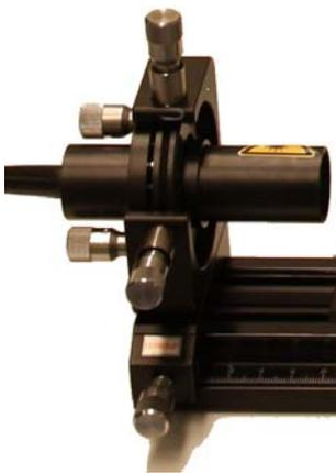
As a laser source a frequency doubled Nd:YVO<sub>4</sub> laser of 30 mW output power (class 3B !) at 532 nm is used. The laser head is mounted in an X,Y –  $\phi$  alignment holder for quick and easy beam adjustment.
