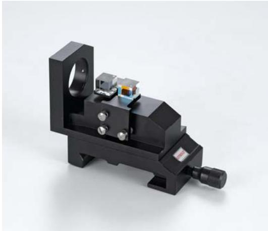
The beam combining unit consists of two different beam splitter cubes: a polarizing cube PBS-01, and a non-polarizing cube BS-02, each mounted on a small adjustment holder. The BS-02 is used for combining the reference and the signal beam, while the PBS-01 directs the laser beam first to the target and then reflects it towards BS-02.
