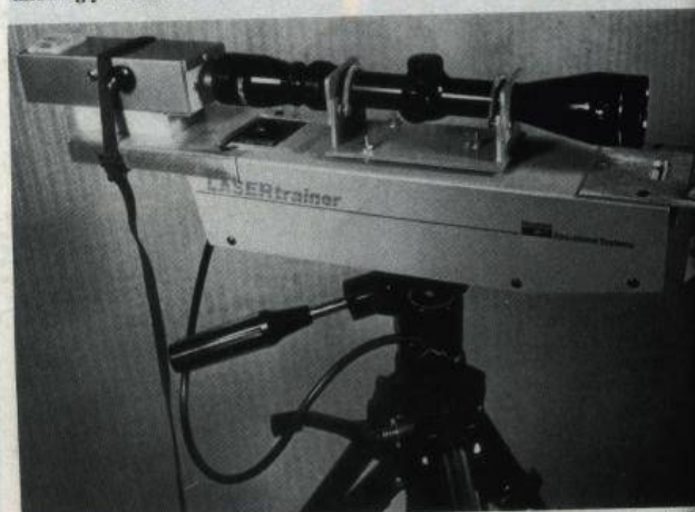
FIG. 2—FOR LONG-RANGE USE the laser and the receiver should be combined into an integral unit. Both are aimed together. The telescopic signal provides precision aiming on the target.
