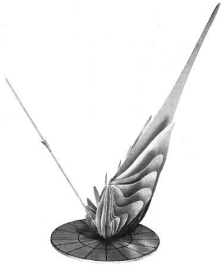
Figure 3: Bidirectional Reflectance Distribution Function of Aluminum
