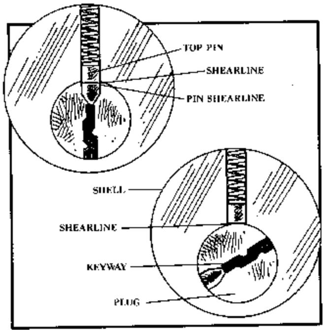
Figure 2. The pin tumbler lock, front view.
