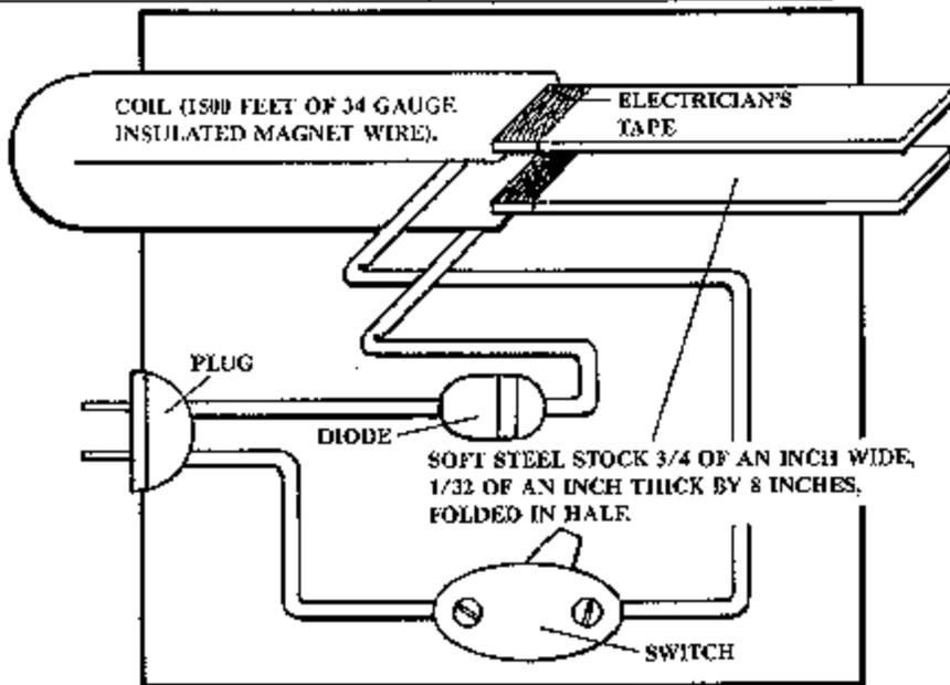
Figure 30. The magnetic pick is easy to construct.
