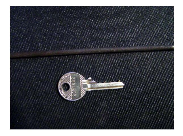
Great, our key now resembles the deepest cuts for this blank. Now we can remove a bit from the tip of the blank and a bit from the shoulder of the key! When we are finished the bumpkey should appear just like this:
