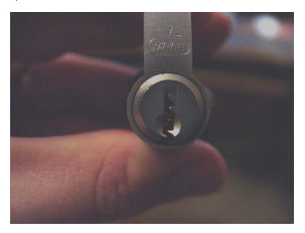
Step one of modifying the key is cutting all depths to the deepest cut. We will use the narrow side of our flat file to take the cuts down to the deepest depth trying to keep our cuts as straight as possible. When we are finished our key looks just like this:
