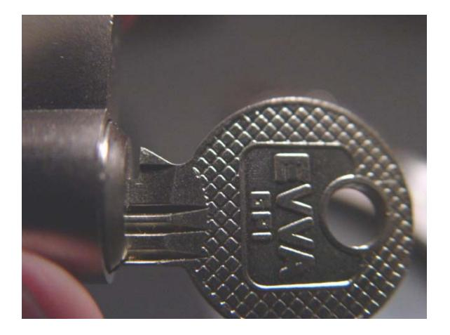
When the key is bumped it will be pushed into the lock against the shoulder of the key as appears in the following picture:
