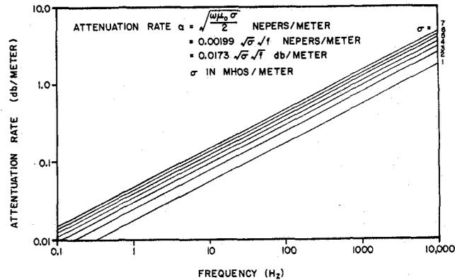
Figure 9. Attenuation factor for different situations as a function of frequency.
