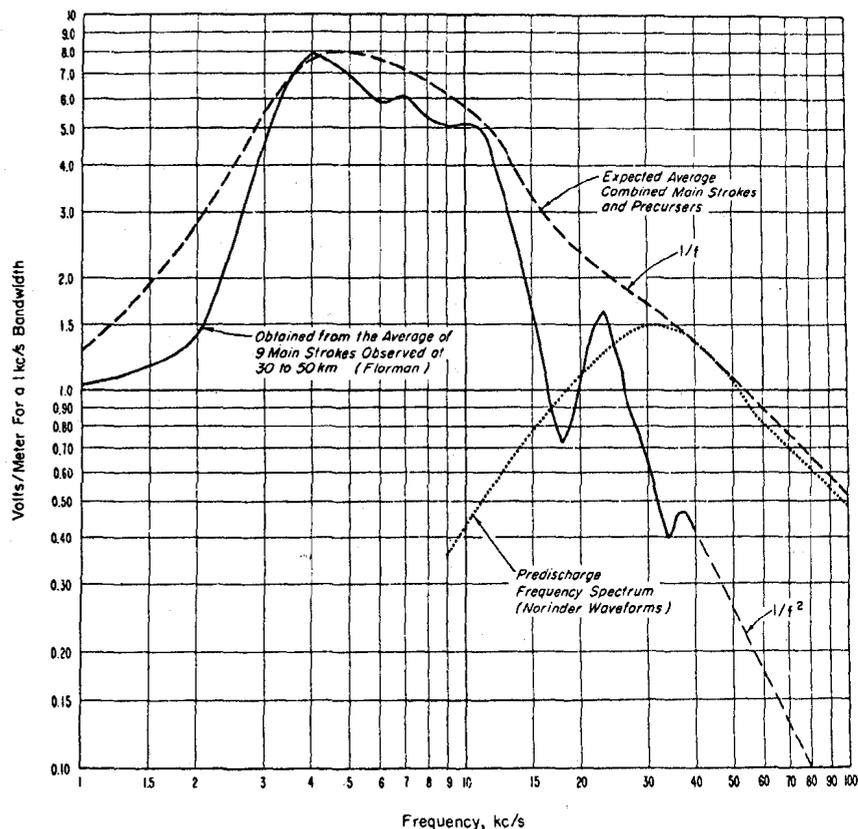
Figure 12. Frequency spectrum of the radiation component, equivalent field intensity at a distance of one mile.
