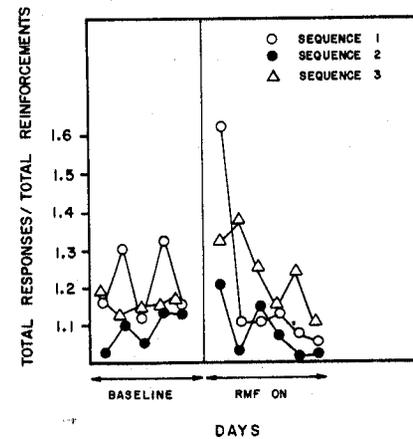
Figure 7. Efficiency ratios ( $R/S^+$ ) for an adult rat daily tested on a DRL-12 second schedule (30 min. daily sessions) during various baseline (sham-field) and RMF (0.8 to 3.0 gauss) exposures. During testing in the operant chamber, the subject was removed from the exposure area. Two control/sham-field control condition rats and another sham-field/RMF condition rat did not display comparable results (Persinger, unpublished data, 1973).
