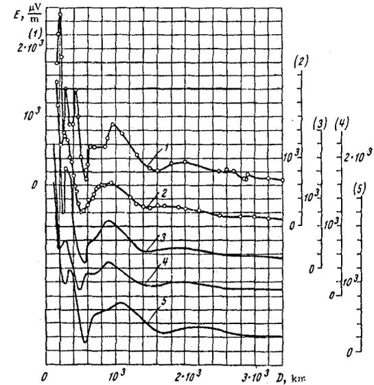
Figure 7. Comparison of the results of field intensity measurements at a frequency of 16.6 kHz and power  $W = 1$  kW (curves 1 and 2) with theoretical calculations (curves 3 - 5).
