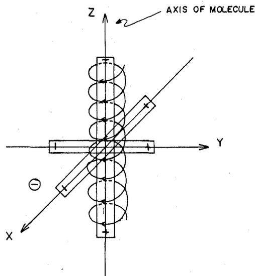
Figure 3. Molecule with a strong heliaxial dipole moment along the z axis. Note relatively weak radial dipole moments (x and y axes).
