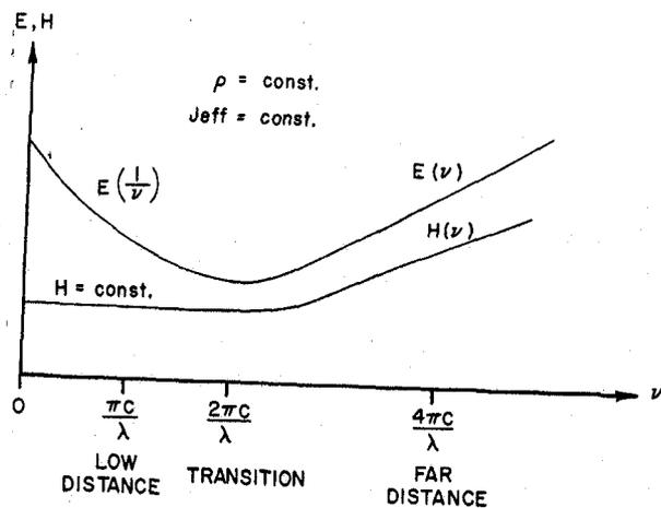
Figure 4. E- and H-field strengths at a fixed distance from the source as dependent on the frequency. Effective antenna current  $J_{\text{eff}}$  is held constant.
