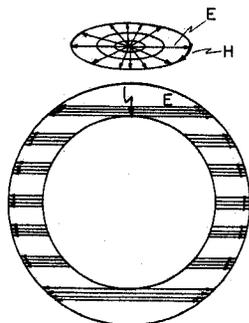
Figure 5. Schumann waves in the earth-ionosphere system for lightning events (above in Fig. 5). A higher order is shown.
