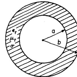
Figure 7. Cross-section of a shielded box having the material constants,  $\epsilon_r$ ,  $\mu_r$ ,  $\sigma$ .
