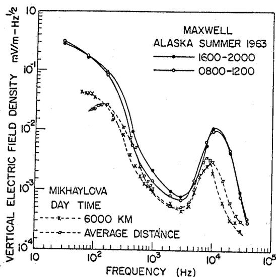
Figure 13. Frequency spectrum of atmospheric noise at the ELF and VLF range.
