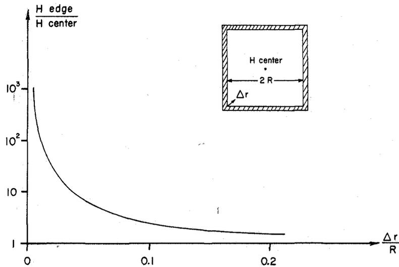
Figure 12. "Corner Effect" in an angular shielded chamber.
