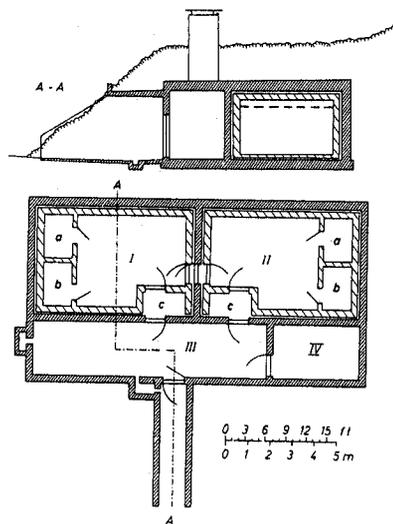
Figure 7. Floor plan and cross section of the isolation station. Narrowly shaded areas: reinforced concrete; widely shaded areas: brick walls. I and II: experimental units (a: kitchen; b: bath room; c: lock); III: control room; IV: experimental chamber. (Wever, 1969b)
