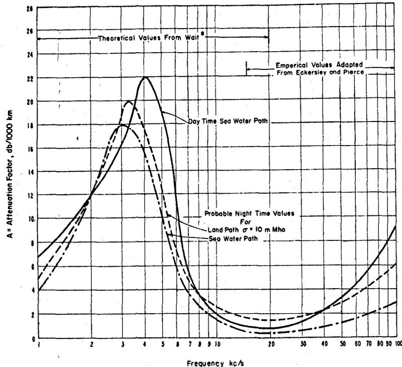
Figure 10. Attenuation rate in sea water for various values of sea water conductivity.
