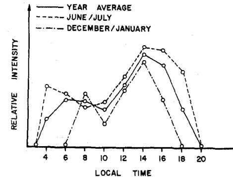
Figure 5. Diurnal variation of strong ELF atmospherics (Schumann resonance at 8 Hz).
