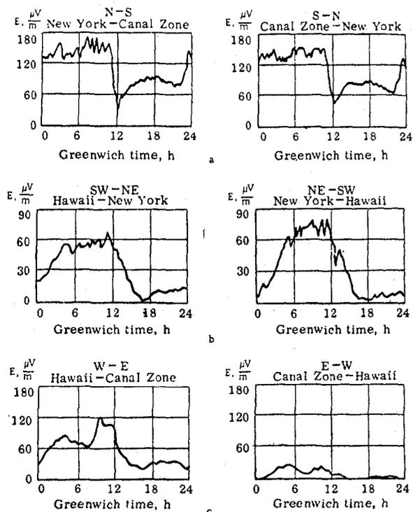
Figure 11. Diurnal variation of the field intensity, measured on different routes at a frequency of 10.2 kHz.
