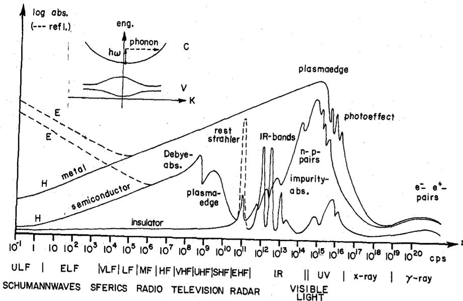
Figure 6. Absorption (and dashed, reflection) of insulators, semi-conductors and metals (qualitatively) as a function of the frequency. Above: Band-diagram for clarification of the plasma-absorption.
