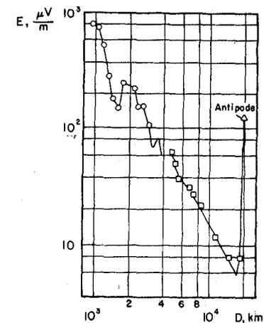
Figure 8. Results of field strength measurements at frequencies of 16.6 kHz (circles), 17.5 kHz (squares) and 14.7 kHz (triangles).
