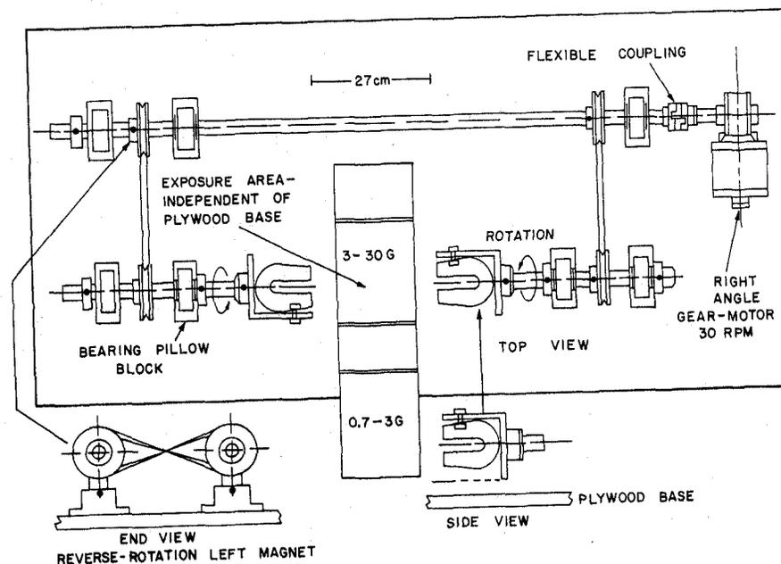
Figure 1. One of the rotating magnetic field apparatus and associated exposure areas (modified from Persinger and Pear, 1972).
