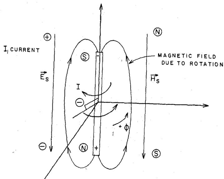
Figure 6. Induced H field caused by rotation in  $+\phi$  direction.
