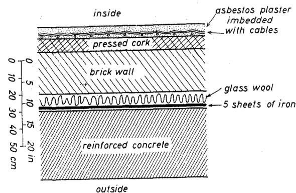
Figure 10. Cross section through a wall of experimental unit II.
