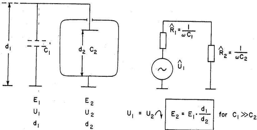
Figure 14. "Antenna Effect" through cables which conduct electromagnetic waves into a shielded chamber from outside. Right: schematic diagram. The circumflex accent over  $U$  and  $R$  indicate alternating size.
