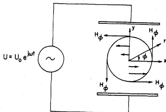
Figure 1. H-curl in an artificially induced field between two condenser plates.
