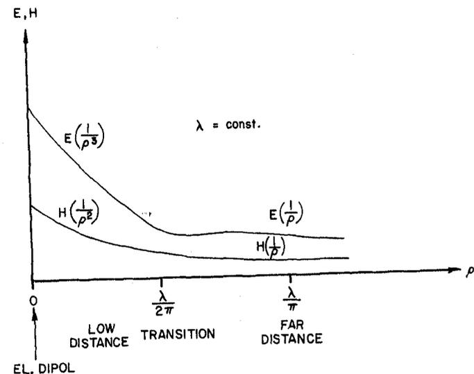
Figure 3. E- and H-field strengths as dependent on distance from the source (electric dipole at the co-ordinate source) for constant frequency or wavelength.
