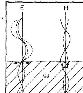
Figure 9. Perpendicular incidence of an electromagnetic wave on copper for the explanation of reflection and weakening.
