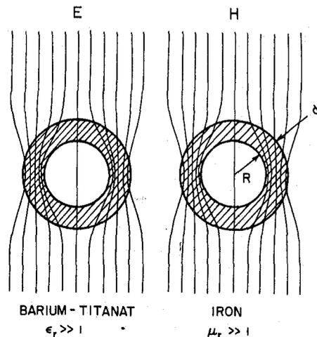
Figure 10. E- and H-field line paths in materials with high  $\epsilon_r$  or  $\mu_r$ .
