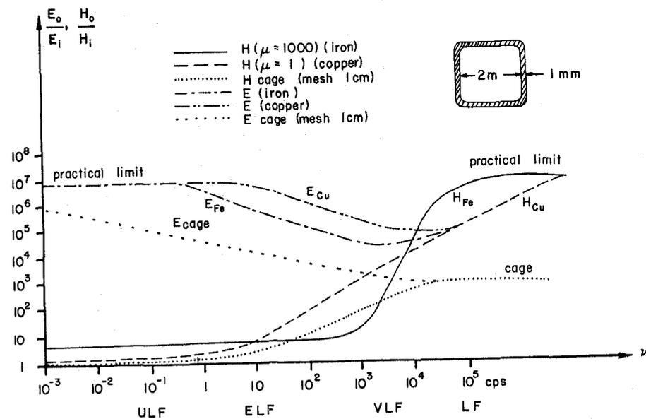
Figure 11. Practical shield factors for electric ( $E_o/E_i$ ) and magnetic ( $H_o/H_i$ ) components at low frequencies for a special box or cage made of copper or steel ( $r = 100$  cm;  $d = 0.1$  cm; mesh distance 1 cm). The practical limit in respect to the theory (eqn 39 to 49) is due to idealization in the theory (homogeneity, smooth surfaces, perfect joints a.s.o.).
