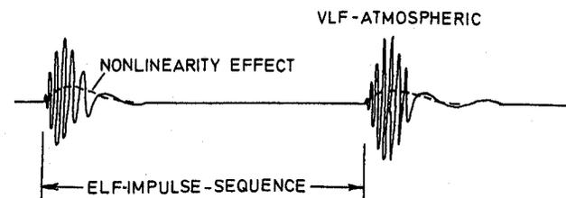
Figure 14. ELF-signal caused by VLF-signals in connection with non-linear effects.
