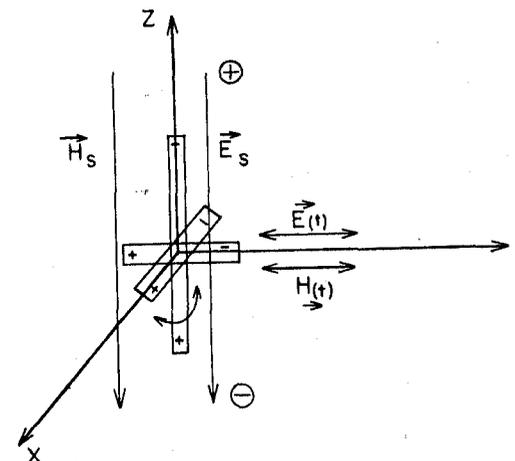
Figure 5. Direction of molecule rotation under applied electric fields.
