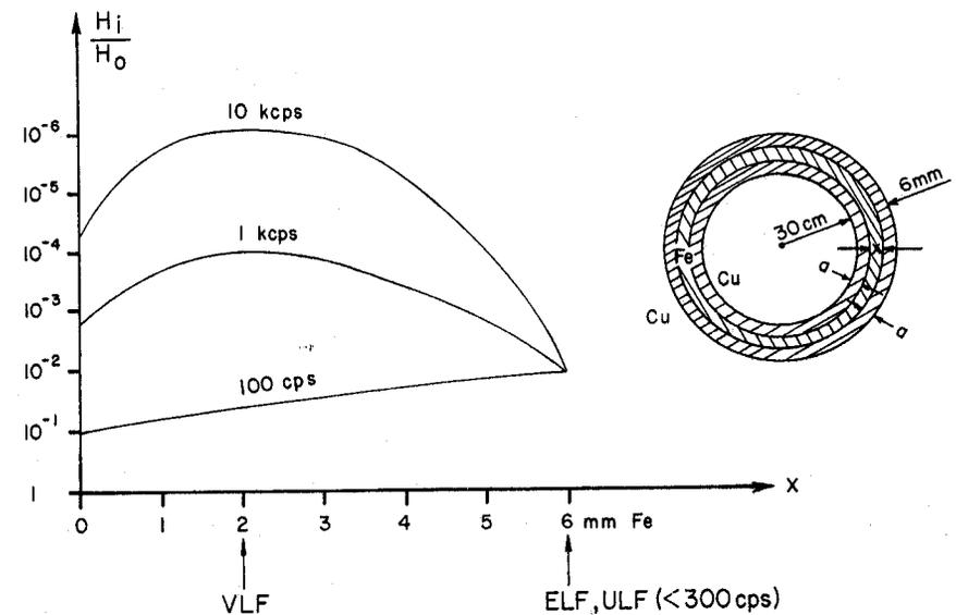
Figure 15. Three-layer shielding as a function of thickness ratios between the three layers.
