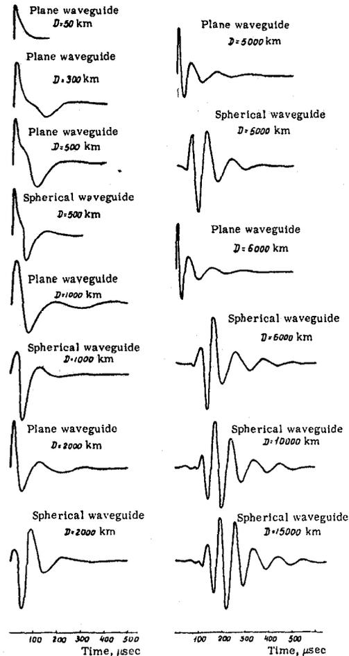
Figure 6. Signal forms  $E(t, D)$  calculated for atmosphericics at distances of 50 - 15,000 km in plane and spherical waveguides.
