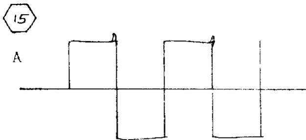
WAVESHAPE AT E & F WITHOUT TRANSDUCERS CONNECTED
