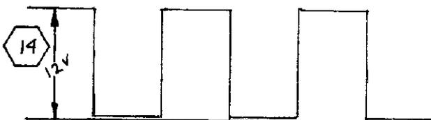
Vce must be no more than .2 volts with Vce being equal to 12V. Waveform must be symmetrical respective to one another with a minimum of ringing and rounding of corners. The adverse conditions will increase as the load is increased.
