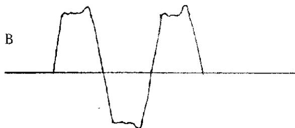
WAVESHAPE AT E & F WITH TRANSDUCERS CONNECTED APPROXIMATELY 30 to 40 VOLTS PEAK TO PEAK.
