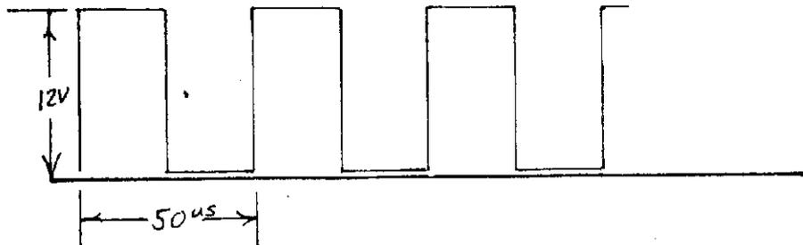
DRIVER OUTPUT TO BASE - THESE WAVE FORMS ARE 180 degrees OUT OF PHASE RESPECTIVE TO ONE ANOTHER (TEST POINTS AND (11 and 12) MUST SUPPLY SUFFICIENT CURRENT TO CAUSE COMPLETE SATURATION OF THE FINAL AMPLIFIER TRANSISTORS.
