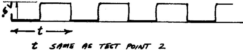
THIS IS THE STEP VOLTAGE TO I1A AND DETERMINES THE RATE OF STAIRCASE GROWTH. NOTE THE WAVE FORM BEING CLIPPED DOWN TO .5V DUE TO THE INPUT OF THE AMPLIFIER I1.
