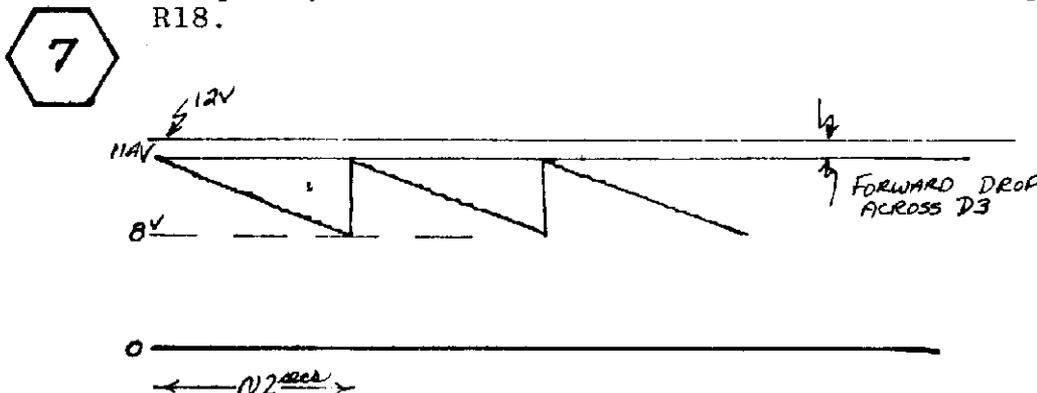
VCO OUTPUT WAVESHAVE - THE ABOVE WAVESHAVE VARIES FROM  $t=100$  usec to 50 usec OR A CORRESPONDING FREQUENCY OF FROM 10KHZ TO 20KHZ, depending on Step 20 adjustments. NOTE SYMETRY OF THIS WAVESHAVE.
