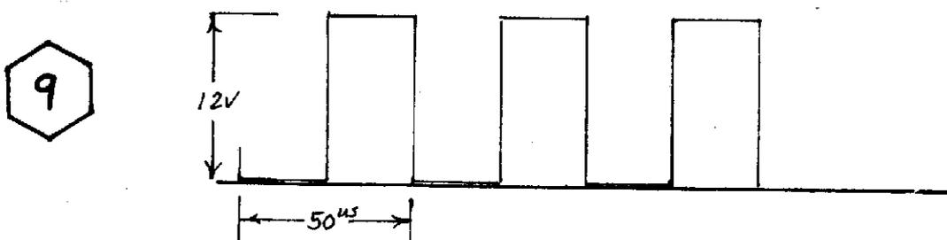
BUFFER STAGE OUTPUT - THIS SINGLE IS A SYMETRICAL SQUARE WAVE SATURATING Q6 AND APPEARING ACROSS R25.
