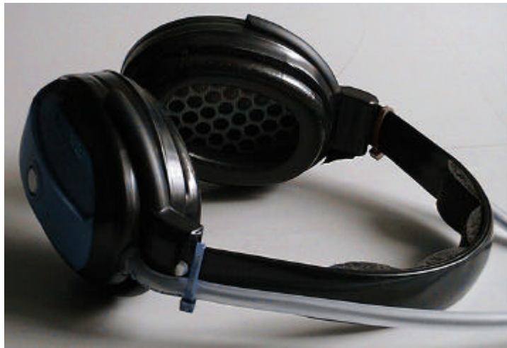
Figure 3: The headphones with safety grill and thick plastic cable protection.
