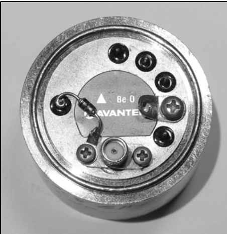
Fig 7: A YIG oscillator with no FM mode.
