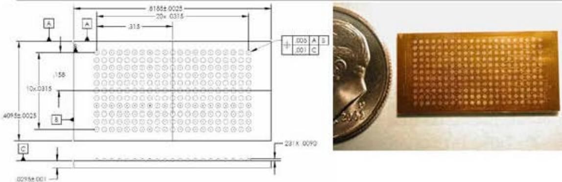
(TS//SI//REL) MAESTRO-II uses the TAO standard implant architecture. The architecture provides a robust, reconfigurable, standard digital platform resulting in a dramatic performance improvement over the obsolete HC12 microcontroller based designs. A development Printed Circuit Board (PCB) using packaged parts has been developed and is available as the standard platform. The MAESTRO-II Multi-Chip-Module (MCM) contains an ARM7 microcontroller, FPGA, Flash and SDRAM memories.
