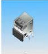
(TS//SI//REL) CM-II will provide software persistence capability, "in-field" re-programmability, and covert communications with a host software implant over the USB. CM-II will also communicate with Data Network Technologies (DNT) software (STRAITBIZARRE) through a covert channel implemented on the USB, using this communication channel to pass commands and data between hardware and software implants. CM-II will be a GENIE-compliant implant based on CHIMNEYPOOL.
