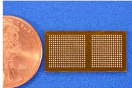
(TS//SI//REL) TRINITY uses the TAO standard implant architecture. The architecture provides a robust, reconfigurable, standard digital platform resulting in a dramatic performance improvement over the obsolete HC12 microcontroller based designs. A development Printed Circuit Board (PCB) using packaged parts has been developed and is available as the standard platform. The TRINITY Multi-Chip-Module (MCM) contains an ARM9 microcontroller, FPGA, Flash and SDRAM memories.
