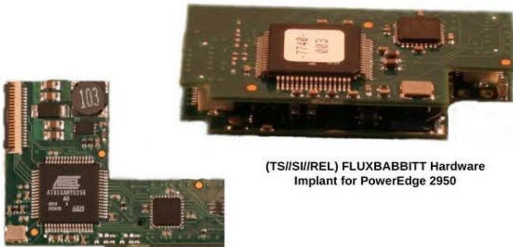
(TS//SI//REL) FLUXBABBITT Hardware Implant for PowerEdge 2950
