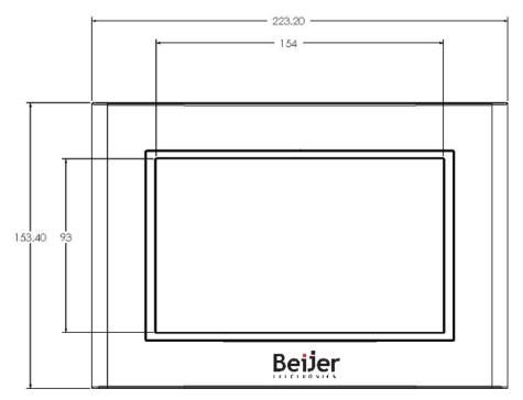
Figure 39 QTERM-G72 Front Panel Mount
