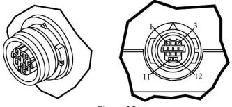
Figure 25 QTERM-G58 Handheld Connector
