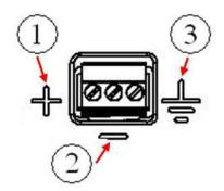
Figure 37 QTERM-G72 3-Pin Terminal Strip
