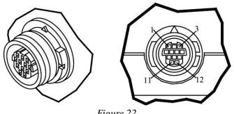
Figure 22 QTERM-G56 Handheld Connector
