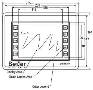
Figure 30 QTERM-Z60 Front Panel Mount
