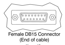
Figure 17 QTERM-G55 Integral Cable Connector
