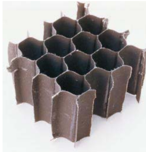
Figure 39. A Sample of Radar Absorbing Honeycomb Material (From [61])
