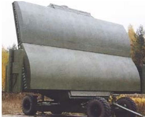
Figure 76. Gamma DE L-band Low Frequency (Upper UHF) Radar (From [107])
