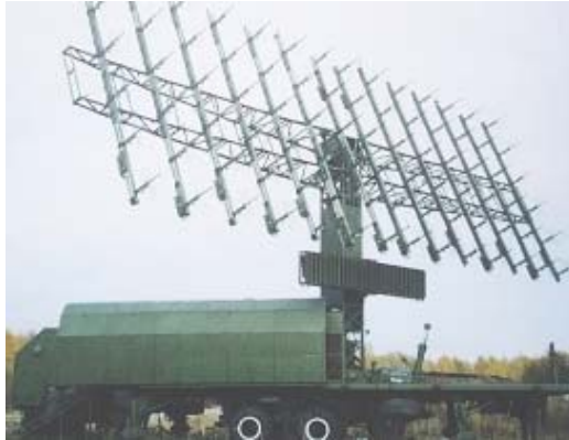
Figure 75. Russian Low Frequency (VHF) Radar Nebo SVU (From [107])
