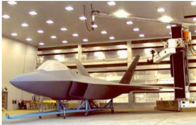
Figure 42. F-22 in the Robotics Coating Facility for Low Observable Material Applications (From [62])
