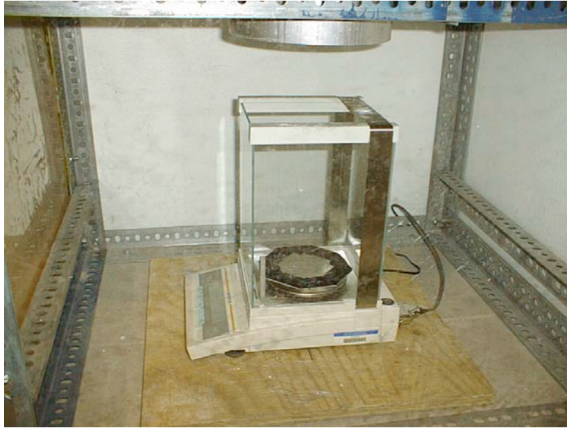
Figure 8b. Image of the scale used to record chaff mass versus time. The fall exit of the fall tower (diameter 8") is just visible at the top of the photograph. Velcro was applied to the perimeter of the scale plate to reduce chaff fall-off.
