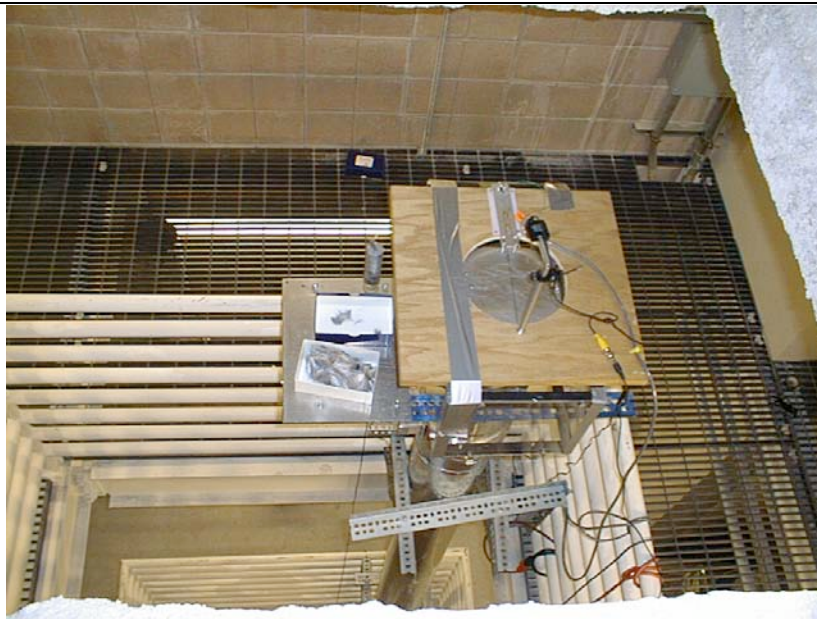
Figure 8a. Photograph of the release mechanism used to deliver chaff to the fall tower. Chaff was placed on the aluminum plates mounted to swing down below the wood platform when the release mechanism was triggered. A miniature black and white video camera, mounted vertically above the aluminum plates, was used to visualize chaff release.
