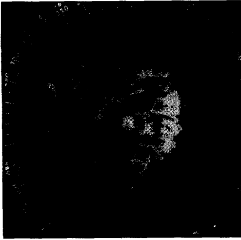
Fig. 15. WSR-57 PPI display of thunderstorm cells on a tornadic day (181704 CST April 19, 1976). Gray shadings (dim, bright, black, dim, etc.) represent dBZ levels differing by about 10 dBZ starting at 17 dBZ. Range marks are 100 km apart, elevation angle = 0.0^\circ . Unambiguous range is 910 km. The boxed area outlines a tornadic storm cell whose mesocyclone signature was detected in real time by NSSL's Norman (NOR) Doppler radar which is nearly colocated with the WSR-57.
