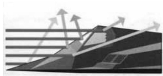
Figure 6: Redirected Radio Waves VII
