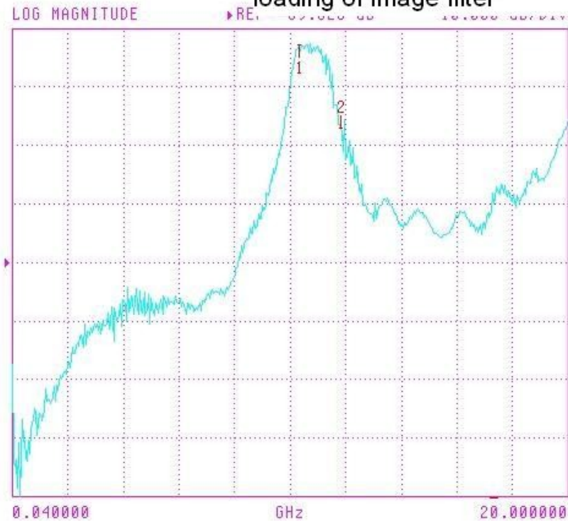
S12 REVERSE TRANSMISSION Amstrad SLB1 - Dielectric loading of image filter
