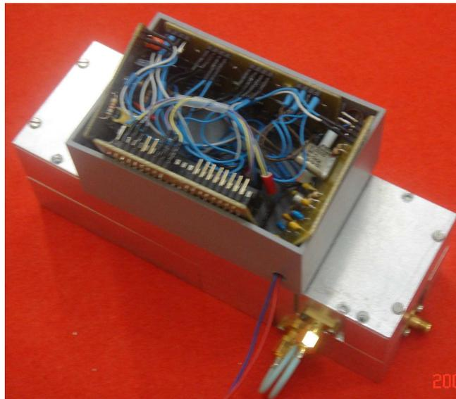
**Figure 5.9:** A photograph of the designed local oscillators.
