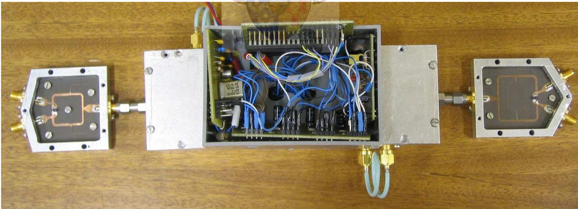
**Figure 5.27:** A photograph of the designed LOs with power dividers.
