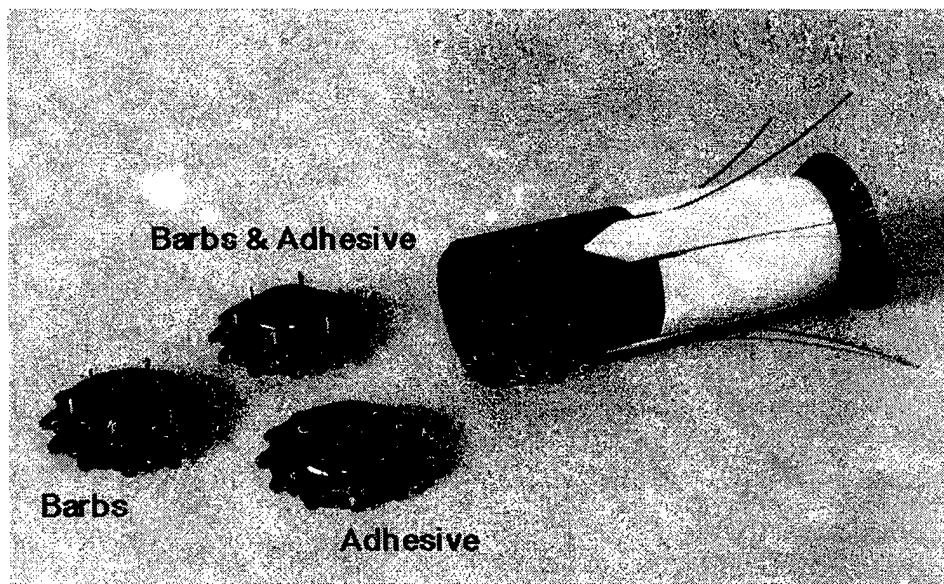
Figure 2. Photograph of Prototype Sticky Shocker projectile with three optional attachment tips.
