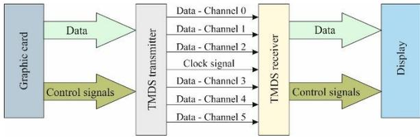
Fig.1. Signal transmission utilizing TMDS protocol
