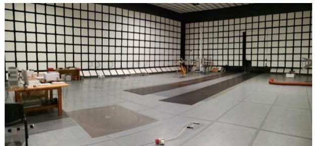
Fig.11. An anechoic chamber
