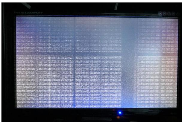
Fig.10. Image reconstructed from the sensitive emission signal for the data transfer via the DP interface; frequency of occurring of the sensitive emission signal  $f_o = 849\text{MHz}$ ,  $BW = 200\text{ MHz}$
