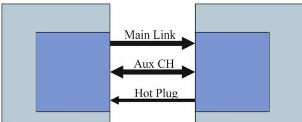
Fig.7. DisplayPort link structure
