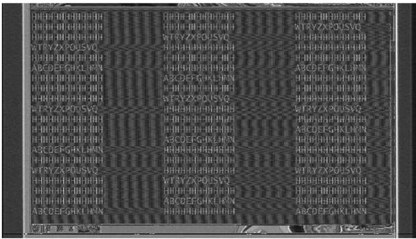
Fig.6. Image reconstructed from the sensitive emission signal for the data transfer via the HDMI interface; frequency of occurring of the sensitive emission signal  $f_o = 419$  MHz,  $BW = 50$  MHz
