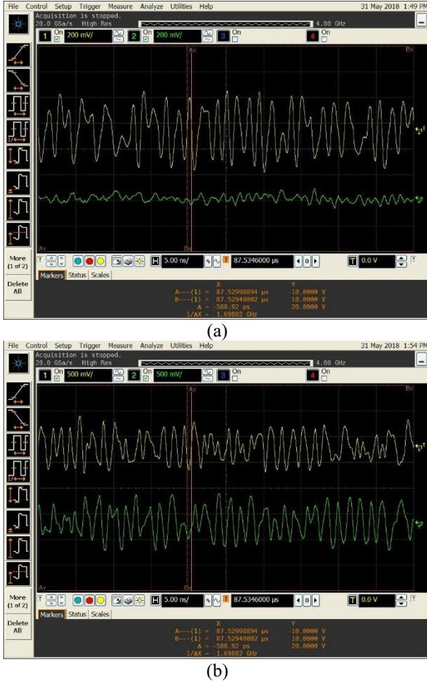
Fig.9. Time series of GREEN signal from DP interface in (a) 640×480/60 and (b) 1920×1080/60 (right) modes, corresponding to one bit of a 10-bit symbol of a pixel of the image displayed on the screen (upper course – Channel 0, lower course – Channel 1)
