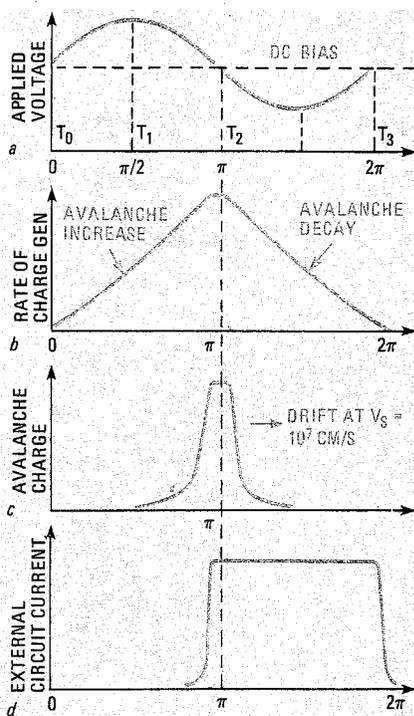
FIG. 12—AVALANCHE CURRENT pulse (b) continues to increase even after the RF voltage cycle has reached its peak (a).
