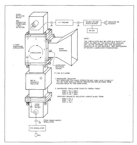
Fig. 1. Waveguide circulator 10-GHz transceiver.
