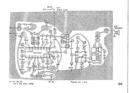
Fig. 3. 30-MHz FM receiver i-f amp (a) schematic, (b) circuit board, foil side, and (c) parts placement.
