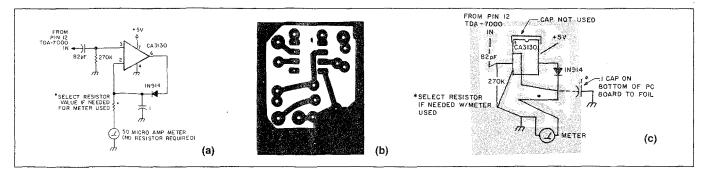
Fig. 2. Signal-strength meter circuit (a) schematic, (b) circuit board, foil side, and (c) parts placement.
