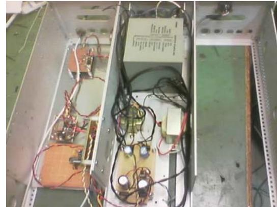
Rack unit: TX modules and power supply
