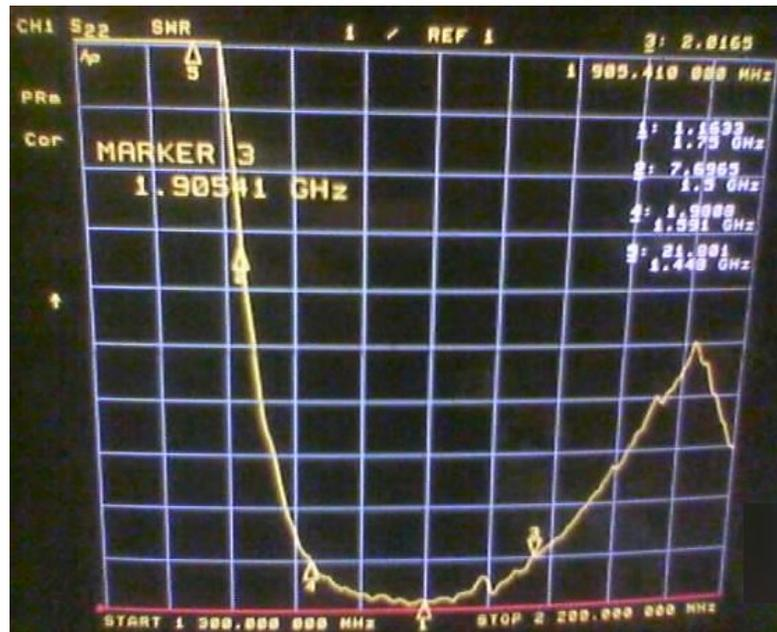
Measured VSWR of open-ended waveguide antenna
