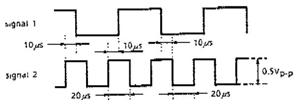
(Note 11) Keyed Pulse Allowable Period :  $T_1$ Input the signal below to pin 1 and open pin 27 and 28. Observe the pin 23 output and change  $f$  so as to be 2.5V voltage.
