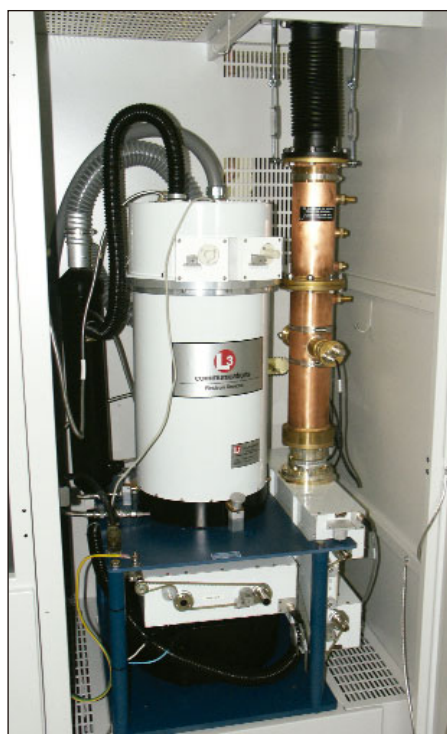
The L-3 CEA tube—an MSDC IOT—is shown here in the Thales DCX Paragon transmitter at WNEO-TV.
