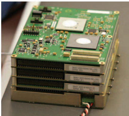
The inner workings of the ROVER, a high-speed, wireless data transmission system that can fit in a suitcase, is assembled in the L3 Communications plant. The unit receives images transmitted to the ground from an aircraft mounted camera and displays them on a laptop.
