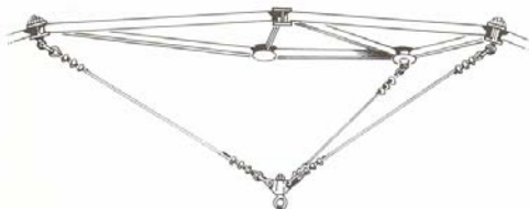
Three-Point Interior Lift Sling for Space Frame Radomes
