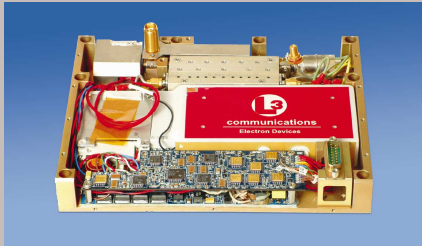
Mini tube integrated into an open Microwave Power Module.
