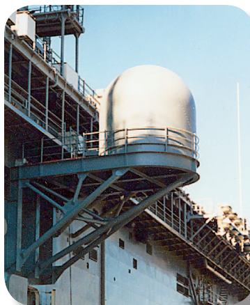
14-ft (4.4m) diameter sandwich radome for SATCOM application.
