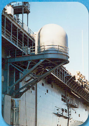
14-ft (4.4m) dia sandwich radome for SATCOM application
